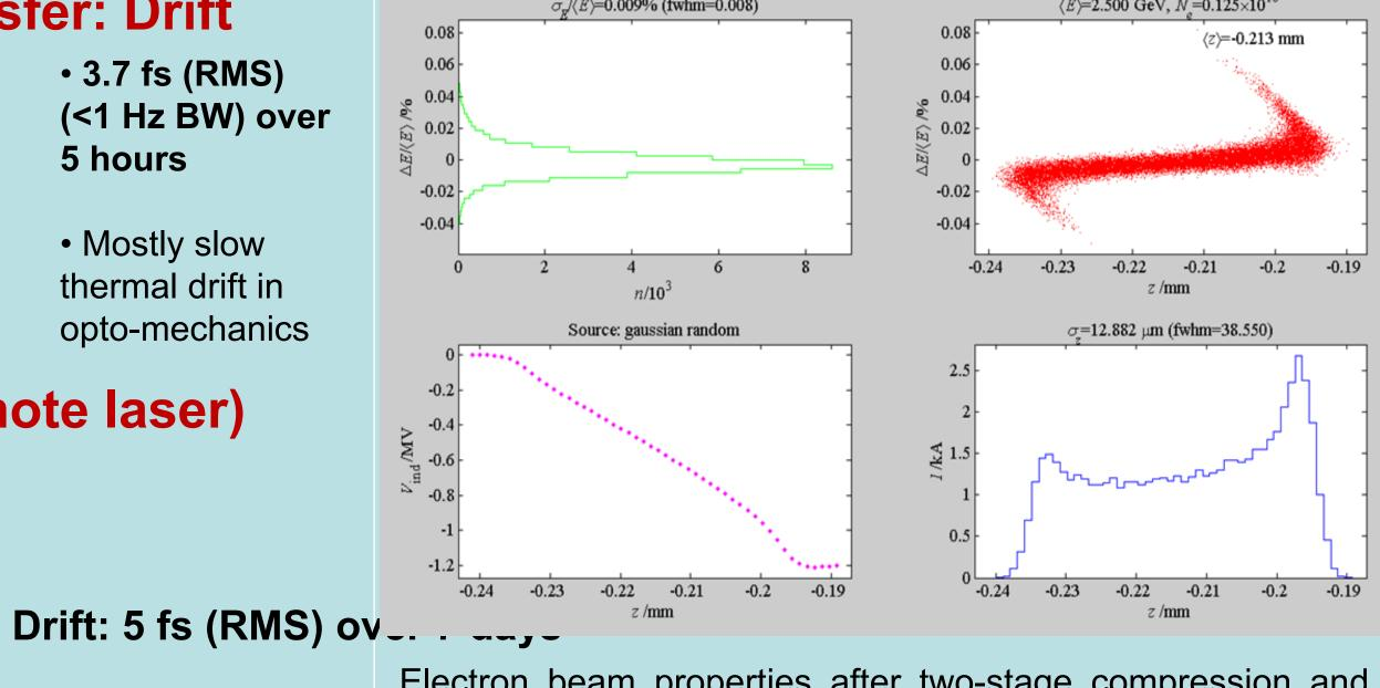
Electron beam properties after two-stage compression and acceleration to final energy of 2.5 GeV.
