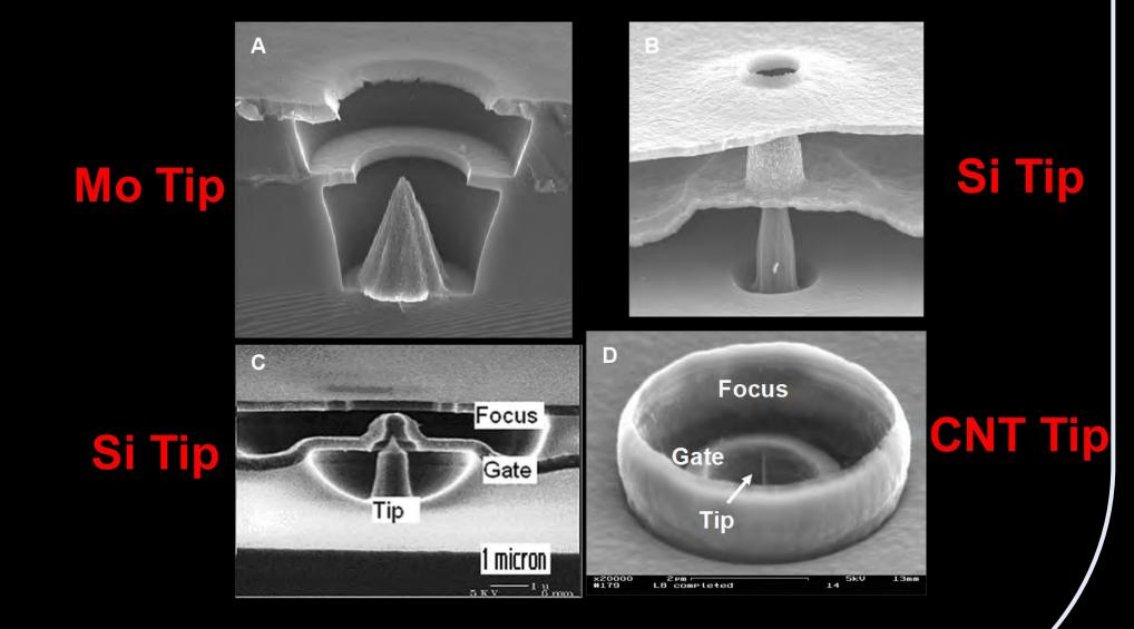
Nanocathode development for high brightness electron beams
