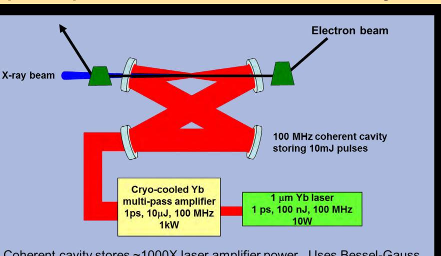
Coherent cavity stores ~1000X laser amplifier power. Uses Bessel-Gauss ring-shaped modes to avoid mirror damage and oscillator instability.
