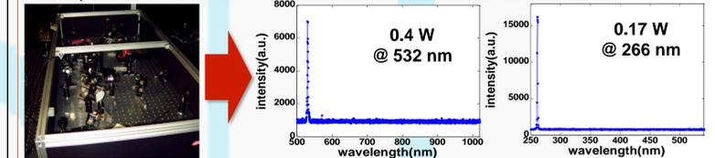
**LASER 2: Cryo-cooled Yb:YAG Laser from Qpeak Inc (STTR).**
