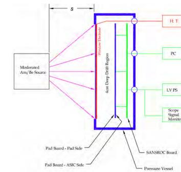
Diagram shows neutrons from moderated Am/Be source uniformly illuminating the full sensitive area of the detector, 24cm × 24cm. Distance "s" adjustable from ~0.1m to ~5m. Note minimal volume of equipment required outside the detector.
