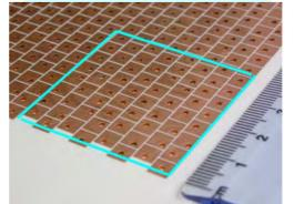
Bottom of anode pad board: 36 ASICs, each with 64 channels
