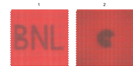
Response of entire 48 × 48 pad detector and full acquisition system to uniform illumination with thermal neutrons. Neutron source is very close to detector window, s ~10cm, and thus there is a fall off of neutron intensity from center to the sides.
