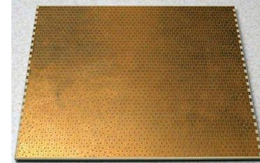
One corner of anode pad board, with outline of 8×8 pads that are connected to one ASIC
