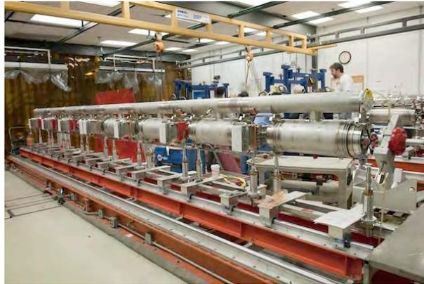
Fig. 3. High gradient superconducting linac cavity strings under assembly at Jefferson Lab.
