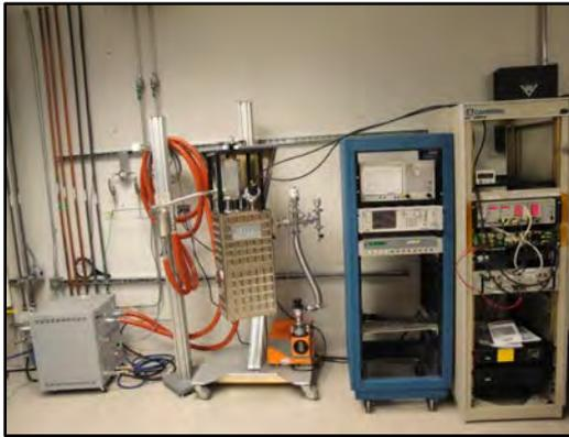
**Figure 1 -- ADR refrigerator setup and microwave test equipment.**
