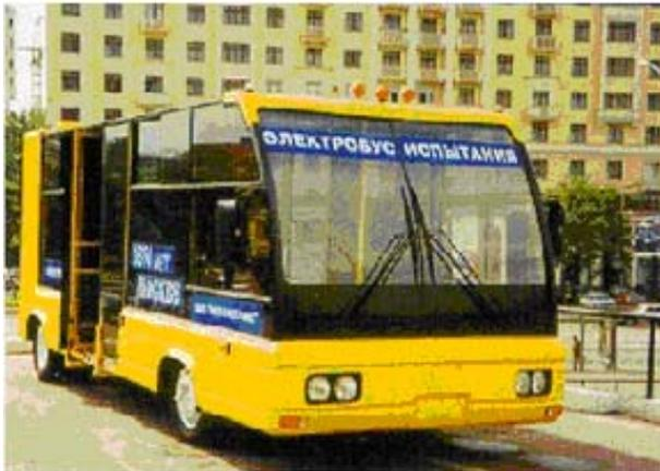
**Fig. 20. Electric bus powered solely by an asymmetric electrochemical capacitor system.**
