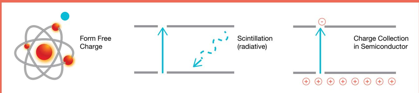
In each of these cases, a certain energy,  $\eta$ , is required to create those secondary quanta, so that  $N = E_e / \eta$  secondary quanta are created. If the X-ray was photoelectrically absorbed, in which case  $E_e = E_\gamma$ , then a measurement of  $N$  is a measurement of the X-ray's energy.
