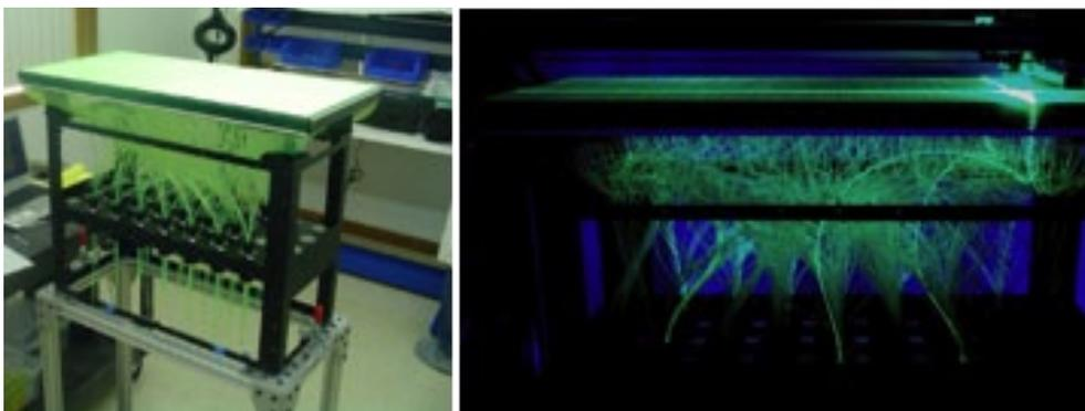
**Figure 14** The WLS fiber detector, in daylight (left) and dark (right). The flat scintillator has an area of 77 × 38 cm<sup>2</sup>, and scintillation light is coupled by 308 and 152 fibers feeding 25 and 7 photomultipliers, respectively, for the X and Y axes.
