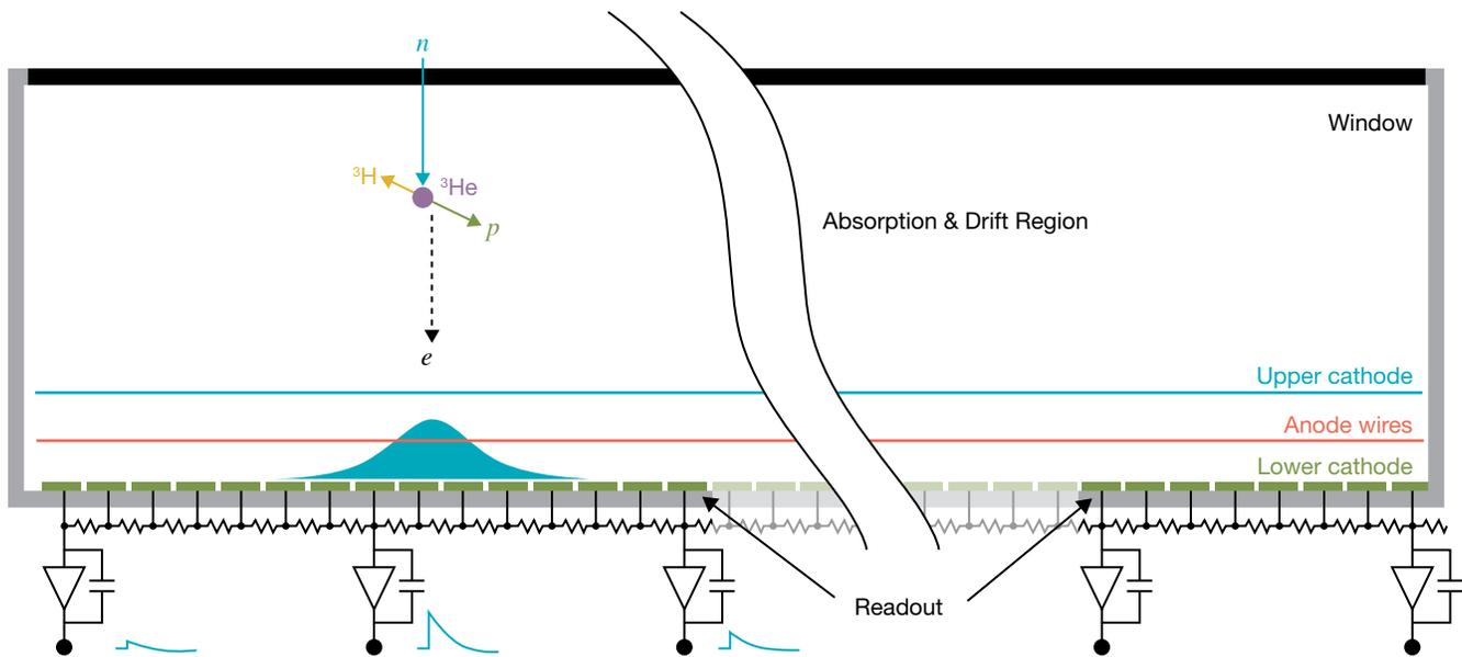
**Figure 18** Schematic of advanced He-3 filled multiwire chamber.
