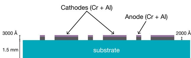
**Figure 20** Cross-sectional view of micro-strip gas chamber (MSGC).
