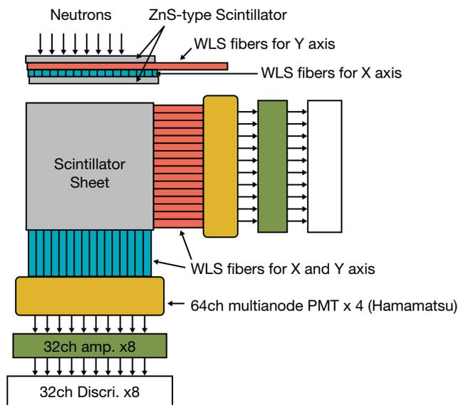
**Figure 23** Key elements of the J-PARC scintillator detector.
