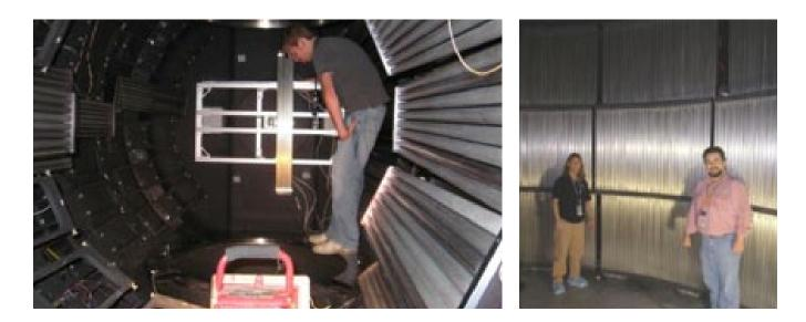
**Figure 17** View of the large-area LPSD detectors at SNS Nanoscale-Ordered Materials Diffractometer (NOMAD) (left) and Wide Angular-Range Chopper Spectrometer (ARCS) (right) instruments.
