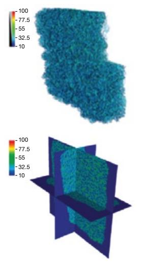
**Figure 27** An ex situ neutron tomographic snapshot of the evolution (suspended) of lithium oxide loading of a carbon graphite foam battery electrode. Microstructural resolution is at the 50 µm size range.
