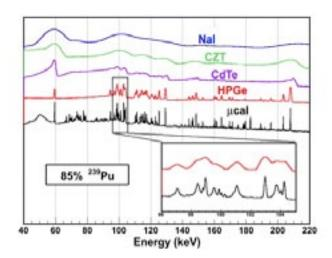
**Figure 11** Comparison of scintillator (Nal), room-temperature semiconductor (CdTe), cryogenic semiconductor (Ge), and superconducting calorimeter energy resolution for very hard X-rays. Figure courtesy NIST/LANL.
