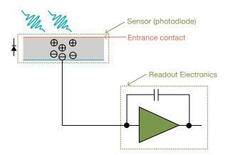
Figure 33 Connection of the sensor to its electronics.
