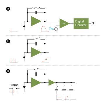
**Figure 8** Different pixel architectures: (a) counting, (b) integrating, (c) fast-framing.
