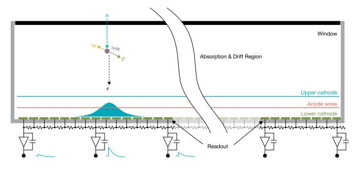
Figure 18 Schematic of advanced He-3 filled multiwire chamber.
