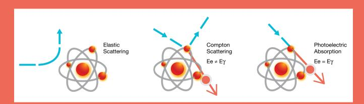
The excited electron can then undergo ionization loss in a material (free charges in a gaseous detector, visible light created in a scintillator, or charge collected in a semiconductor), leading to a detectable signal.
