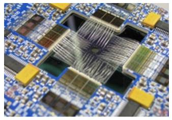
Figure 32 Maia detector showing intricate wire bonds.
