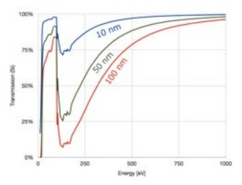
**Figure 10** Transmission vs. energy for different thicknesses of entrance window.
