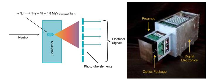
Figure 22 Schematic of Anger camera (left) and one module with 15×15 cm<sup>2</sup> sensitive area (right).
