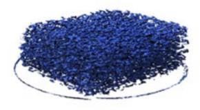
**Figure 28** 3-D Li distribution  $(Li_2O_2)$  in coarser foam matrix, which can help to address interfacial transport and the Li transport in complex electrodes (degradation issues).
