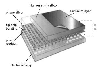
Figure 30 Hybrid pixel detector.
