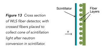
that absorbs the blue photons from the scintillator and re-emits the photons at a longer (green) wavelength (hence the name "wavelength-shifting"), some of which then travel to the ends of the fibers.
