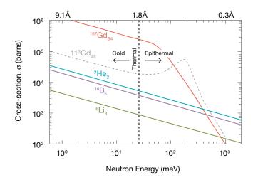
**Figure 12** Neutron absorption cross section vs. neutron energy.
