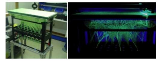
**Figure 14** The WLS fiber detector, in daylight (left) and dark (right). The flat scintillator has an area of 77 × 38 cm<sup>2</sup>, and scintillation light is coupled by 308 and 152 fibers feeding 25 and 7 photomultipliers, respectively, for the X and Y axes.
