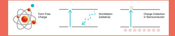
In each of these cases, a certain energy,  $\eta$ , is required to create those secondary quanta, so that  $N = E_e / \eta$  secondary quanta are created. If the X-ray was photoelectrically absorbed, in which case  $E_e = E_{\gamma}$ , then a measurement of N is a measurement of the X-ray's energy.
