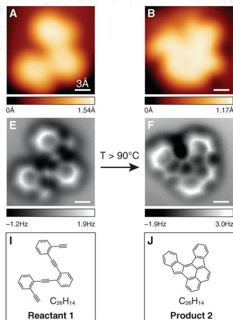
**Fig. 5.** Non-contact atomic force microscopy images (center) of a molecule before and after reaction show dramatic improvement over images from a scanning tunneling microscope (top) and closely resemble the classic molecular structure diagrams (bottom) [de Oteyza 2013].
