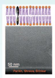
Nanostructure supported ion channel system.
