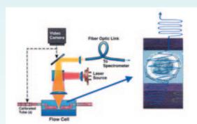
Fig. 2. Compact microfluidic system for reading nanolaser chip output spectra and images for high throughput analysis of endospores.
