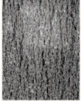
Field-Structured Composites – showing simulated (top) and actual (bottom) structures.
