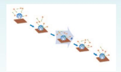
Magnetic particles labeled with molecular recognition elements bind target if present. After 1-second pulse of magnetic field, only bound particles send relaxation signal for detection in the next second. No more than 2000 magnetic particles are required, which, for detection of bacteria or viruses, could translate into fewer than 10 targets.
