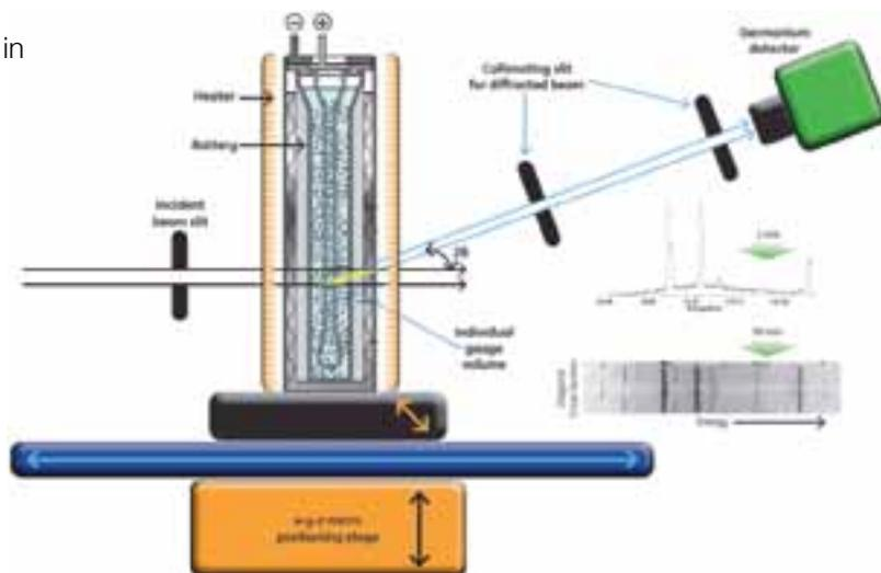
**Experimental Setup on X-Ray Beamline X17B1 at the National Synchrotron Light Source.** The powerful x-ray beam penetrates deep into a full-size sodium-metal-halide battery during charging and discharging. Using a detector to measure the energy and intensity of the diffracted x-ray beam, researchers can track chemical fluctuations inside the battery. [Courtesy of General Electric.]
