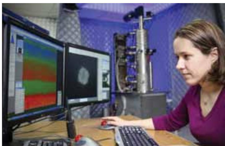
**New Imaging Technique Enables Spin Mapping at the Atomic Scale.** Using an electron microscope, Maria Varela views the atomic arrangements of a magnetic oxide interface. Varela and her colleagues are using this advanced instrument to better understand magnetic properties of materials (see Research Accomplishment on p. 18). [Courtesy of Oak Ridge National Laboratory.]
