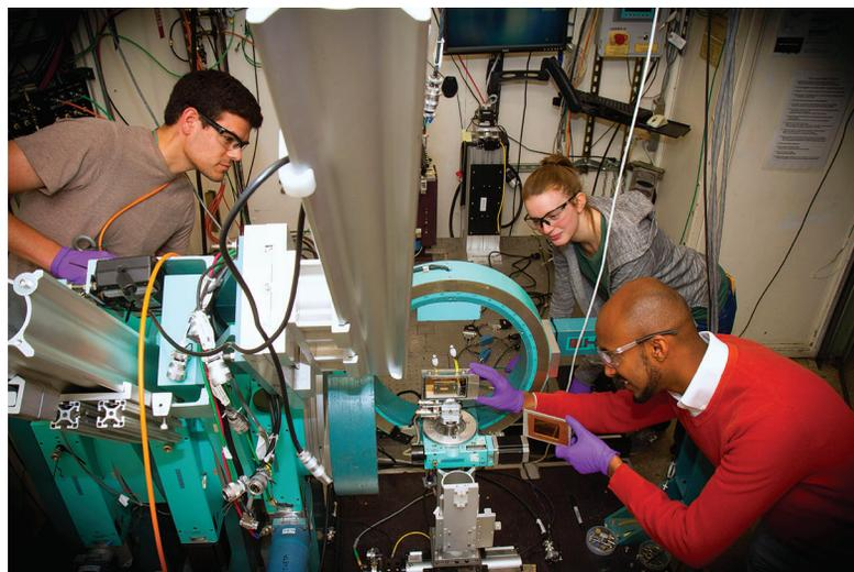
*Stanford University graduate students install an X-ray cell for battery research using the SLAC National Accelerator Laboratory X-ray synchrotron.*
