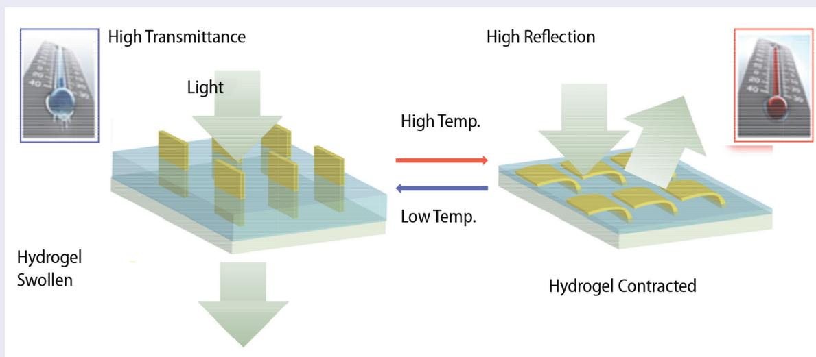
Schematic showing the mechanism by which temperature-sensitive hydrogel polymers can self-regulate the transparency of window (CREDIT: DR. PHILSEOK KIM, AIZENBERG LAB)
