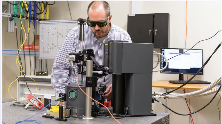
*Argonne scientist Alan Dibos aligns optics to study materials for a possible quantum repeater device; the materials are in a cryostat that keeps them at a temperature just 3 degrees above absolute zero.*
