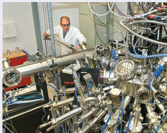
*Ivan Bozovic with the atomic-layer-by-layer synthesis system he developed and uses at Brookhaven National Lab to engineer superconducting materials one atomic layer at a time.*
