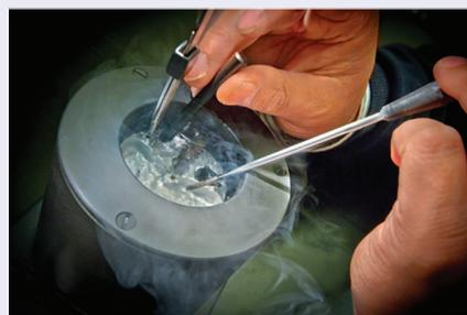
*Cryo-electron microscopes, such as the one shown here, are the most powerful in the world because they capture images with electrons, not light. Samples are frozen in a super-cooled container (inset).*
