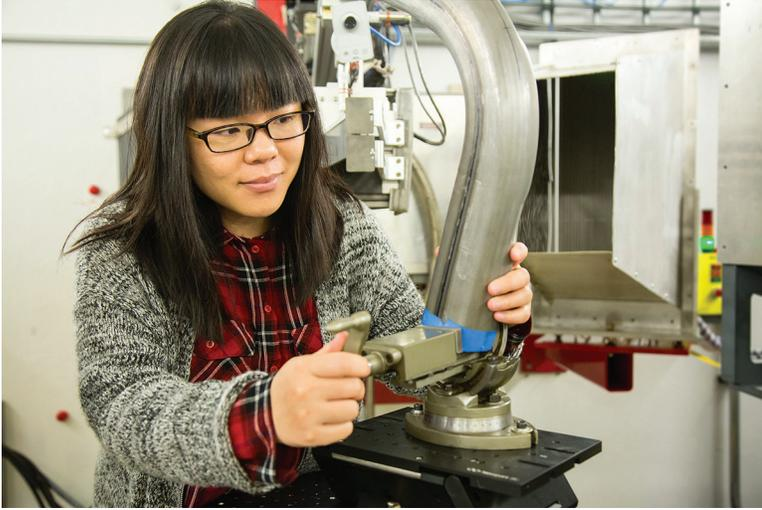
Lu Huang, an industrial research engineer with United States Steel Corporation, prepares a light-weight high-strength steel component for neutron research at Oak Ridge National Laboratory's Spallation Neutron Source. (CREDIT: GENEVIEVE MARTIN/ORNL)
