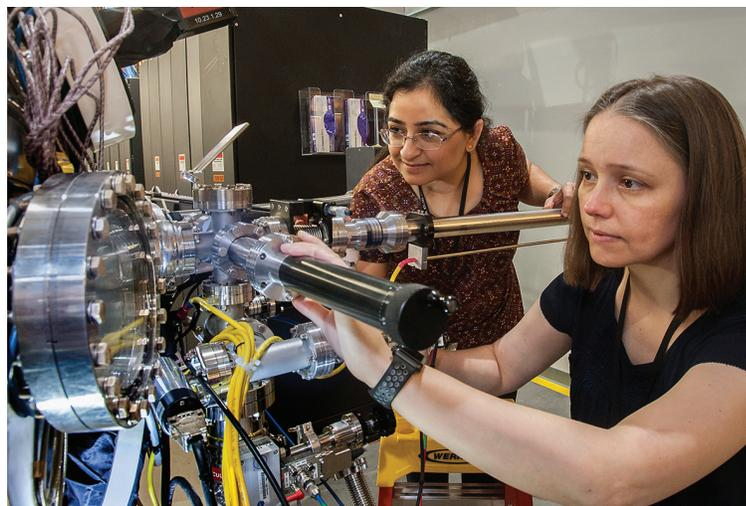
*A Brookhaven National Laboratory staff scientist and a visiting researcher mount a material sample to measure its electronic structure with the laboratory's X-ray synchrotron. (CREDIT: BROOKHAVEN NATIONAL LABORATORY)*
