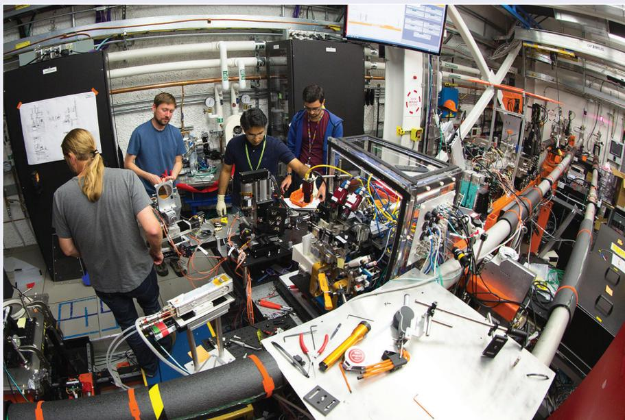
*The experimental setup for documenting the chemistry of the water-splitting reaction at the XFEL X-ray laser*
