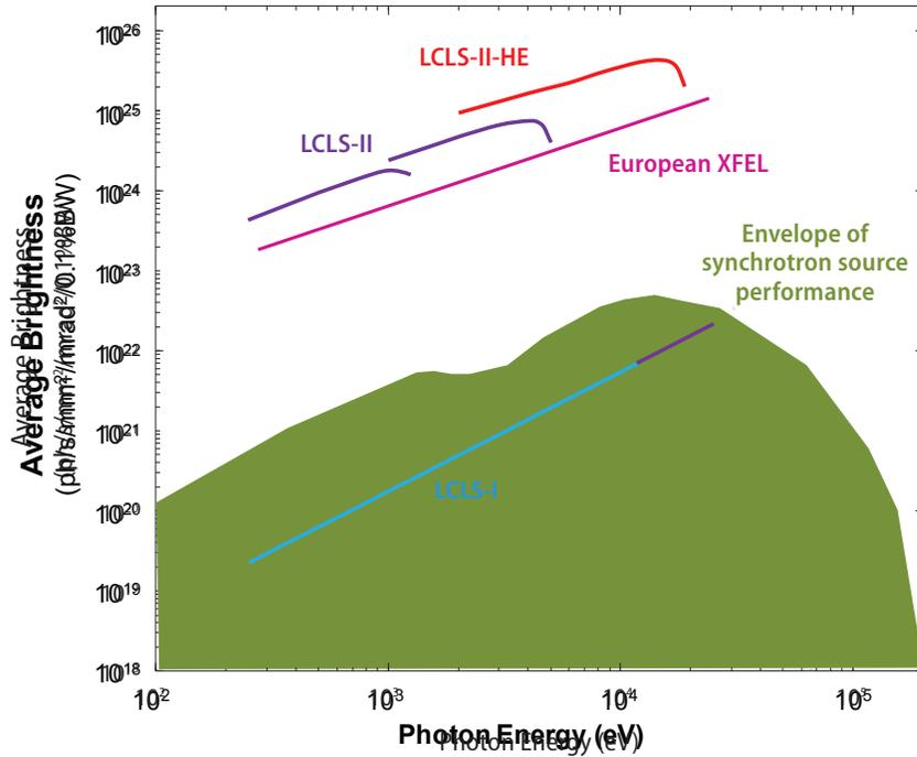
FIGURE 2. Comparative plot of the average brightness of the LCLS facility, along with representative curves for the European XFEL and synchrotron sources. Other current XFEL sources are comparable to LCLS-I; SHINE will be at the level of LCLS-II-HE or higher.
