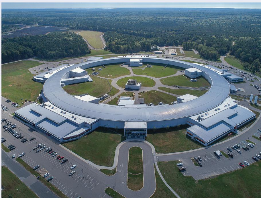
*This aerial view illustrates the enormous scale of the recently upgraded Brookhaven National Laboratory's X-ray synchrotron. Electrons travelling near the speed of light in the circular magnetic storage ring are converted into X-rays for research use at dozens of individual experimental stations adjacent to the ring.*
