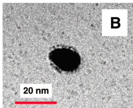
**Figure 2:** CryoEM observation of a single Ag(0) nanoparticle protected from aggregation by the association of polyoxometalate ions [31].
