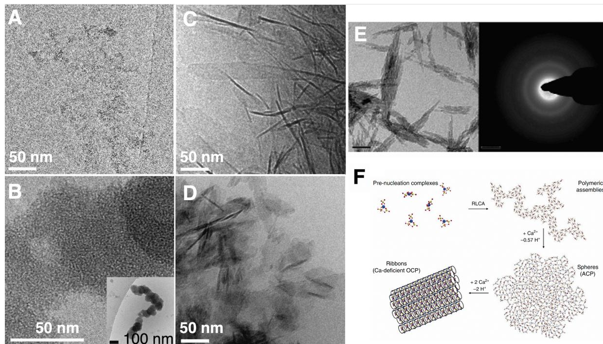
**Figure 3:** CryoEM observations of intermediates in the early-stage formation of calcium phosphate from aqueous solution of (A) polymeric strands from nanometer-sized units, (B) aggregated spheres, (C) ribbons, and (D) elongated plates. (E) Structural analysis using electron diffraction. (F) Mechanism of nucleation, growth and phase transformation developed from cryoEM and molecular simulation studies [38].
