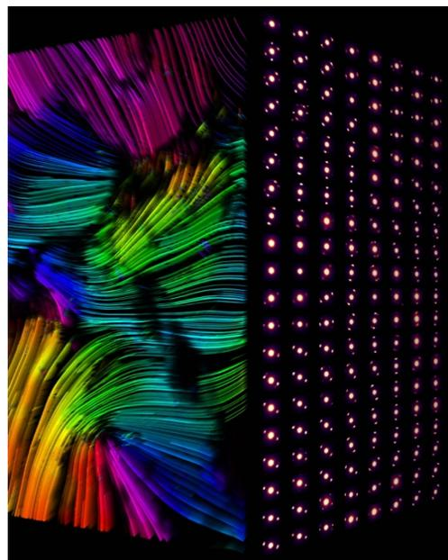
**Figure 7:** Cryo 4D-STEM of a dropcast p-DTS(FBTTh<sub>2</sub>)<sub>2</sub> small molecule sample. At left is a flow map showing the continuity of lattice orientations in space. At right is a selection of diffraction patterns that generated the flow maps. Adapted from [81].
