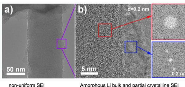
**Figure 13:** CryoEM (a) image and (b) regional zoomed-in image with the bulk and surface FFT result of the EDLi using conventional carbonate electrolyte [96].
