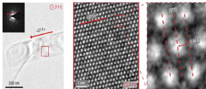
**Figure 12:** Atomic-resolution cryoEM of Li metal dendrites: Left, TEM images of Li metal dendrite. Middle and right, higher magnification images of the boxed region [95].
