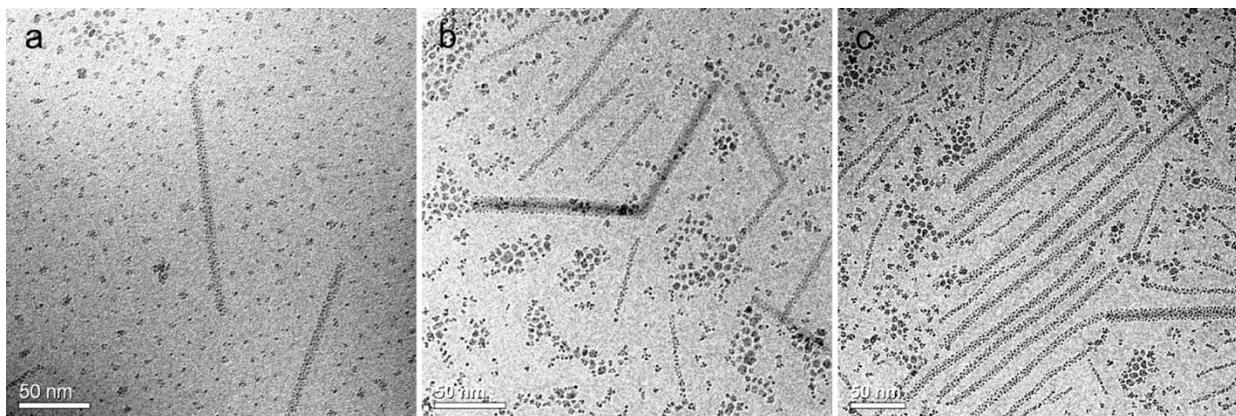
**Figure 5:** CryoEM images of goethite mesocrystals after (a) 5 days, (b) 10 days, (c) 24 days of aging at 80°C [41].
