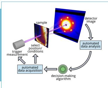
Autonomous control of experimental systems promises to open the study of problems previously considered impossible. Automating the entire experimental workflow—instrument setup and tuning, sample selection and synthesis, measurement, data analysis and model-driven data interpretation, and follow-up experimental decision-making—will bring about revolutionary efficiencies and research outcomes.
