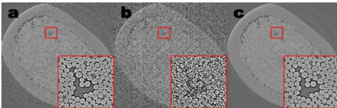
**Figure 23. Tomographic images of a fiber-reinforced minicomposite, reconstructed using (a) 1,024 projections and (b) 128 projections and the result from the (c) MS-D training.** *Source: Jamie Sethian, University of California–Berkeley.*
