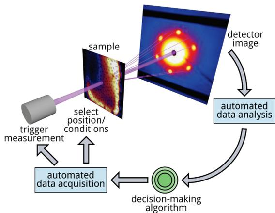
**Figure 22. CAMERA schematic of an autonomous x-ray scattering experiment.** When the measurement is performed, the data acquisition and processing occur automatically. From the processed data, the SMART algorithm selects the next measurement parameters. *Source: Kevin Yager, Brookhaven National Laboratory.*
