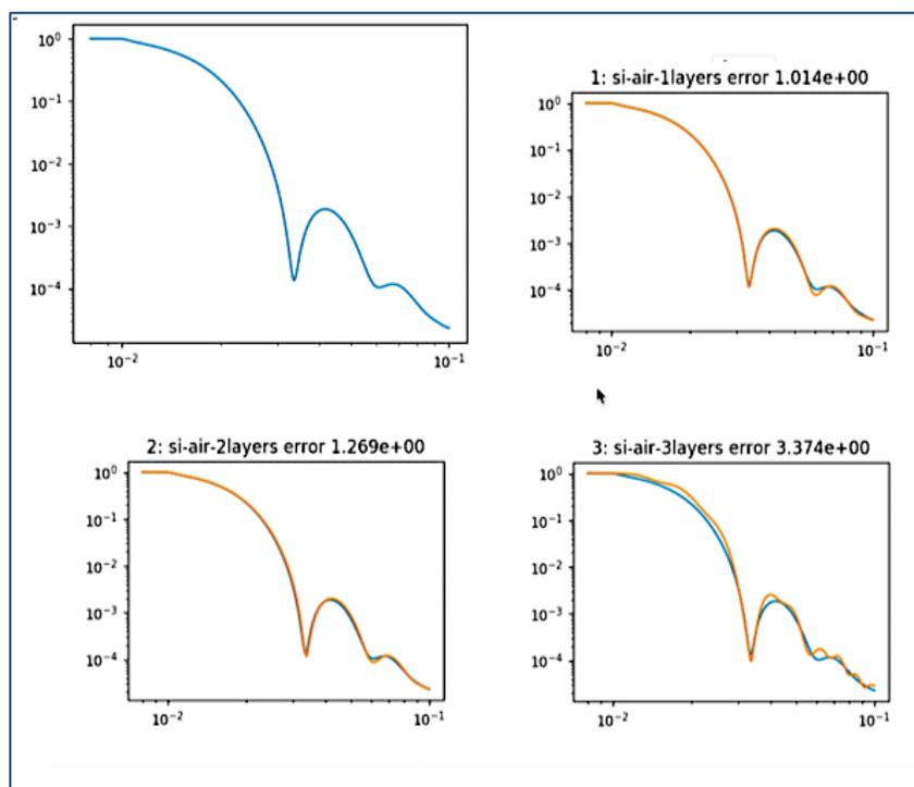
**Figure 20. An application of regression-based ML for neutron reflectivity.** The k-NN algorithm successfully modeled input data with thin-film models. *Source: Mathieu Doucet, Oak Ridge National Laboratory.*
