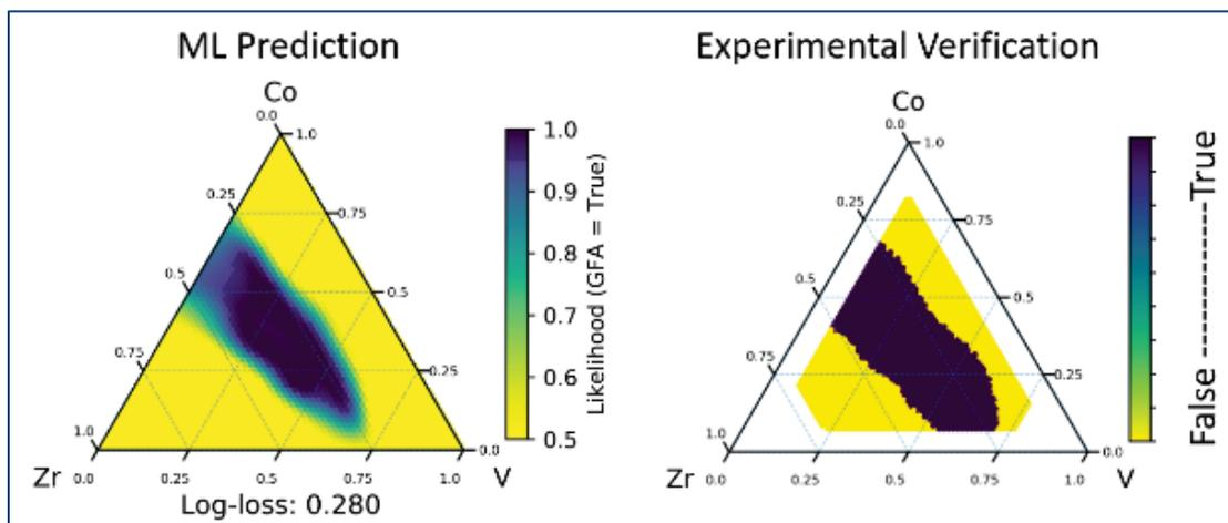
**Figure 16. Machine-learned prediction of amorphous compositionally complex alloys and experimental verification.** Source: F. Ren et al., *Sci. Adv.* 4(4) (2018), eaaq1566. Distributed under terms of Creative Commons Attribution License.
