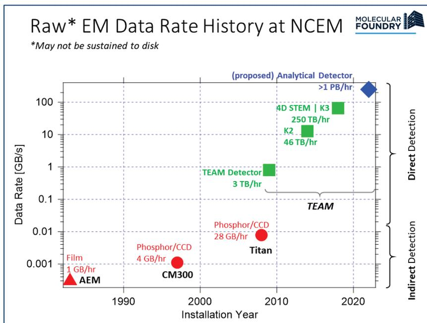
**Figure 3. Electron microscopy data rate at the National Center for Electron Microscopy/ The Molecular Foundry.** Source: Lawrence Berkeley National Laboratory.
