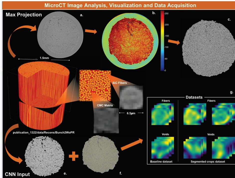
**Figure 5. Multiscale image analysis (a–g) from global analysis of ceramic matrix composites to local detection of fiber profiles with convolutional neural networks leveraging knowledge from previous experiments at the ALS.** *Source: Image courtesy of Daniela Ushizima, Lawrence Berkeley National Laboratory.*
