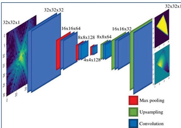
**Figure 10. Structure of CDI NN, a deep convolutional encoder–decoder network trained to predict structure and strain from raw x-ray diffraction imaging data.** Source: Cherukara, M. J., Nashed, Y. S., and Harder, R. J. (2018). *Sci. Rep.* 8(1), 16520. Distributed under terms of Creative Commons CC BY License.
