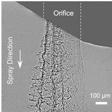
**Figure 11. A 100 ps x-ray phase contrast image showing a fast-turbulent flow of liquid from a fuel injector.** Combined simulation and reconstructive techniques that incorporate AI and deep learning are being developed to reveal 3D liquid complex morphology and fast dynamics. *Source: Image courtesy of J. Wang, Argonne National Laboratory.*
