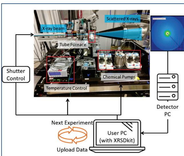
**Figure 17. Data collection and computation workflow for an autonomous experiment designed to discover process conditions for a nanocrystal catalyst material of specific size and polydispersity.** *Source: Apurva Mehta, SLAC National Accelerator Laboratory, Stanford University.*
