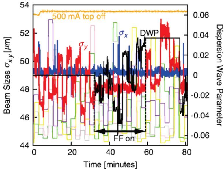
**Figure 7. Vertical beam size (red) is shown to stabilize under application of a feed-forward neural network.** The area between the arrows highlights the influence of the neural network on the beam size and the dispersion wave parameter. *Source: Permission to use image granted by Alexander Hexemer. Licensed under Creative Commons Attribution 4.0 International License.*
