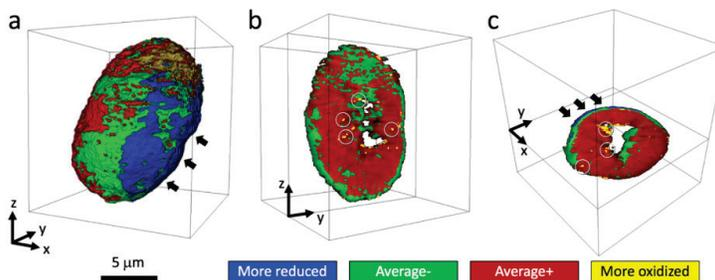
**Figure 18. 3D distribution of four cobalt phases discovered from a hybrid supervised and unsupervised analysis of a collection of x-ray absorption spectra collected on a multiply cycled and partially charged battery cathode particle.** The red and green phases were anticipated, but the blue and the yellow phases were unexpected. *Source: Y. Mao, et al. Adv. Func. Mater. 29, 1900247 (2019) Permission granted by Wiley.*
