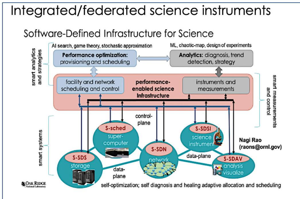
Figure 25. Schematic diagram illustrating different levels of “self-optimizing” computing and the concept of a federated software infrastructure for science. Source: Nagi Rao, Oak Ridge National Laboratory.
