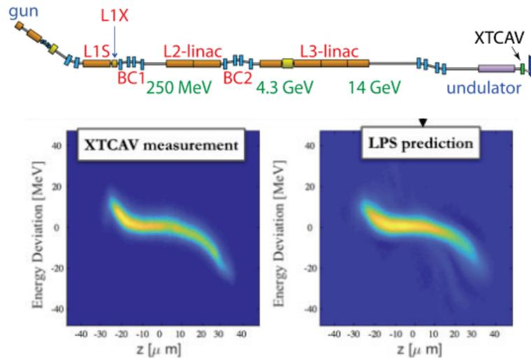
**Figure 13. The NN-based surrogate model prediction (right) reproduces the electron beam distribution obtained through measurement (left) for the LCLS beamline (schematic at top).** Source: C. Emma, et al., *Phys. Rev. Accel. Beams* (2018), American Physical Society under terms of Creative Commons Attribution 4.0 License.
