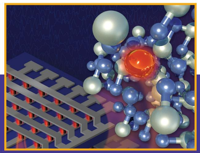
Cover image: A simplified schematic of a cross-bar circuit element designed for future low power, non-volatile memory or neuromorphic computing applications. "Row" and "column" metal interconnects form the cross-bar structure, with nanoscale memory elements residing at the intersections. Current research is focused on the design of these materials at the atomic level to enable dense digital and analog memory arrays with performance characteristics well beyond today's circuits.
