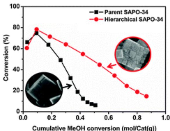
**Figure 23.** Fluoride-treated zeolites show enhanced catalytic activity compared with the pristine material.<sup>73</sup> | Reproduced with permission of The Royal Society of Chemistry from X. Chen et al. 2016. "The Preparation of Hierarchical SAPO-34 Crystals via Post-Synthesis Fluoride Etching." *Chemical Communications* 52 [17]: 3512–15.
