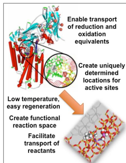
**Figure 22.** Translating design principles seen in enzymes into inorganic materials could enable synthesis of catalysts that exhibit high activity and selectivity near ambient temperature. | Image courtesy of Bruce Garrett
