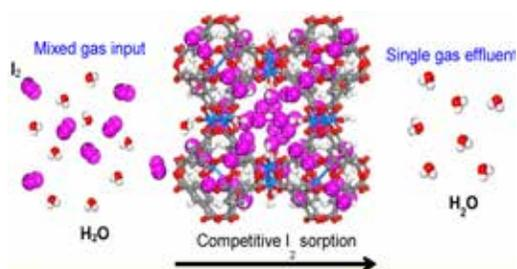
**Figure 26.** Example of selective sorption in surface functionalized MOFs.<sup>78</sup> | Reprinted with permission from D. F. Sava et al. "Competitive I<sub>2</sub> Sorption by Cu-BTC from Humid Gas Streams." *Chemistry of Materials*, 25 [13]: 2591–96. DOI: 10.1021/cm401762g. © 2013 American Chemical Society.
