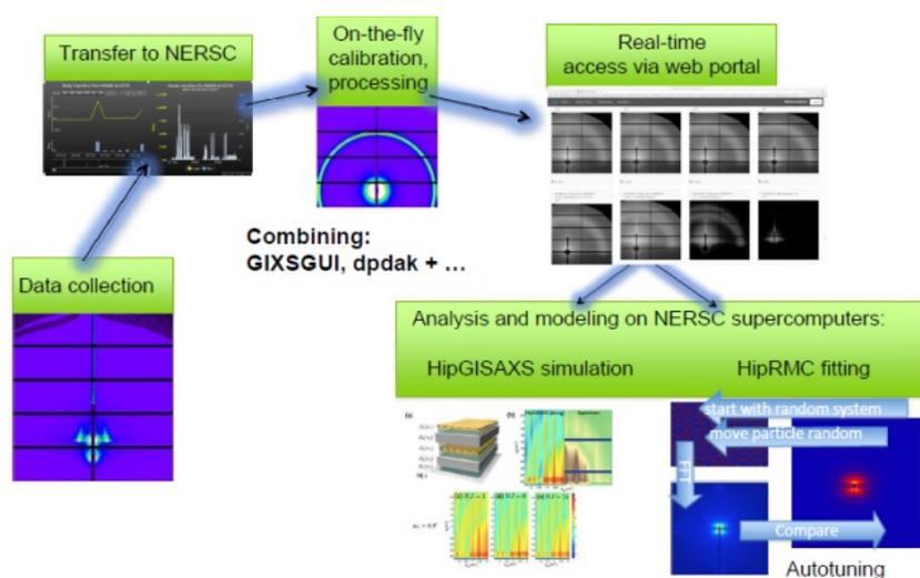
**Figure 7.** Real-time data analysis and modeling setup that streams grazing-incidence small-angle x-ray scattering (GISAX) data to the high-performance computing resources at the National Energy Research Scientific Computing Center (NERSC). Note: GIXSGUI = GISAX graphical user interface; HipRMC = High-performance Reverse Monte Carlo; dpdak and HipGISAXS are the names of software packages. | Images courtesy of S. Billinge, Columbia University
