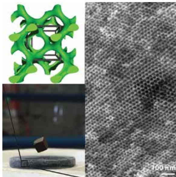
**Figure 18.** Block copolymer self-assembly directed synthesis of mesoporous gyroidal superconductors.<sup>27</sup> | From S. W. Robbins et al. "Block Copolymer Self-Assembly-Directed Synthesis of Mesoporous Gyroidal Superconductors." *Science Advances* 2 [1]: Article ID e1501119. DOI: 10.1126/sciadv.1501119. © 2016.
