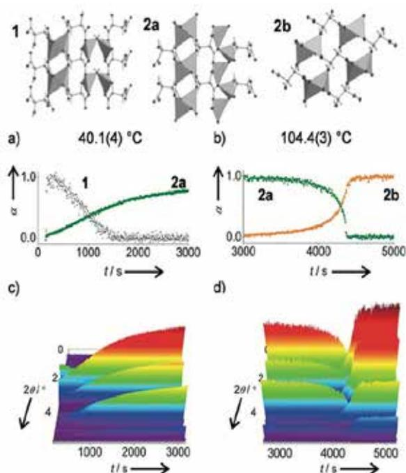
**Figure 52.** In situ monitoring of hydrothermal synthesis of a metal-organic framework by synchrotron XRD as a function of time.<sup>1</sup> | Reprinted with permission from H.H.M. Yeung et al. "In Situ Observation of Successive Crystallizations and Metastable Intermediates in the Formation of Metal-organic Frameworks." *Angewandte Chemie-International Edition* 55[6]: 2012–16. DOI: 10.1002/anie.201508763. © 2016 John Wiley and Sons.
