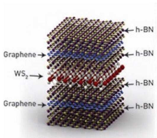
**Figure 46.** Heterostructure of stacked graphene, transition metal chalcogenide, and hexagonal boron nitride.<sup>104</sup> | Reprinted with permission from F. Withers et al. “Light-Emitting Diodes by Band-Structure Engineering in van der Waals Heterostructures.” *Nature Materials* 14 [3]: 301–06. DOI: 10.1038/nmat4205. © 2015 Macmillan Publishers.
