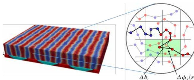
**Figure 34.** Prediction of block copolymer structure based on coarse grain model of dynamic self-assembly. | Image courtesy of P. Nealey and J de Pablo
