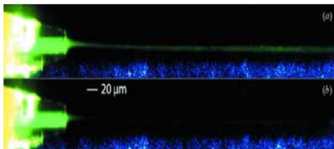
**Figure 65.** Stream of luminescent dye in a double-focusing mixing jet without (upper) and with (lower) quencher, illustrating the rapidity of mixing with this device.<sup>86</sup> | Reprinted from D. Wang et al. 2014. *Journal of Synchrotron Radiation* 21 [6]: 1364–66. Distributed under the terms of the Creative Commons Attribution [CC-BY] License.
