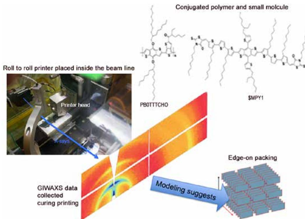
**Figure 60.** Demonstration of high-throughput in situ characterization of conjugated polymer phase formation. | Image courtesy of S. Billinge
