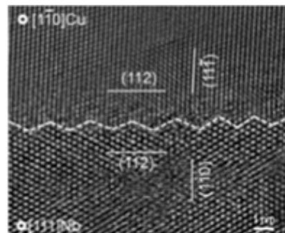
**Figure 49.** Synthesis of nanolaminates via extreme plastic straining of bimetallic composites can lead to a natural selection of interfaces that possess atomic order.<sup>60</sup> | Adapted with permission from I. J. Beyerlein et al. 2015. "Emergence of Stable Interfaces under Extreme Plastic Deformation." *PNAS* 111[12]: 4386–90. DOI: 10.1073/pnas.1319436111.
