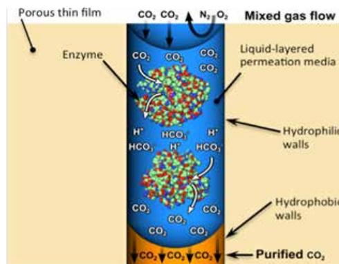
Figure 17. Nano-stabilized enzymatic membrane for CO<sub>2</sub> capture.<sup>2</sup> | Image courtesy of Sandia National Laboratories
