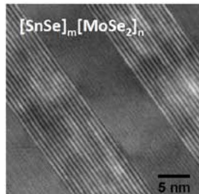
**Figure 12.** Alternating SnSe/MoSe<sub>2</sub> layers define a new phase deposited by a physical phase deposition method. A bulk composition of layered Sn–Mo–Se phase has not been reported.<sup>14</sup> | Reprinted with permission from M. Beekman et al., "Controlling Size-Induced Phase Transformations Using Chemically Designed Nanolaminates." *Angewandte Chemie International Edition* 52(50), 13211–14 (2013). DOI: 10.1002/anie.201305377. © 2013 John Wiley and Sons.
