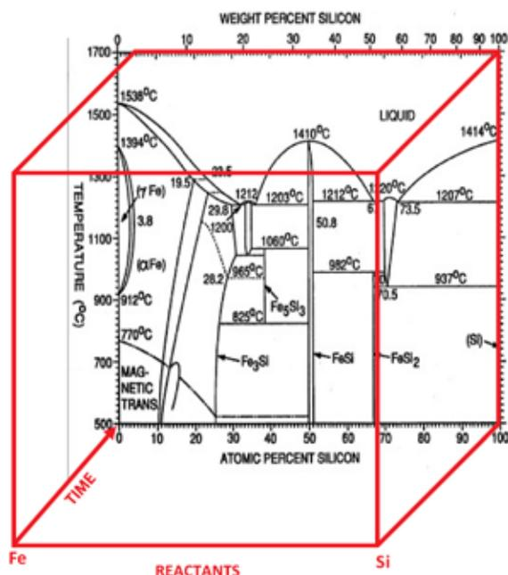
**Figure 15.** An example of a generic multivariable phase diagram incorporating reaction time to include both stable and kinetically stabilized materials within the illustration. The thermodynamic phase diagram in the end is the equilibrium phase diagram. | Image courtesy of M. Kanatzidis.
