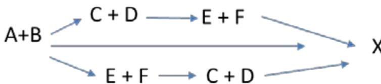
**Figure 9.** In this generic reaction scheme, reactants A and B combine to create the product X. A variety of pathways can occur during this process, including the formation of metastable phases (C, D, E, and F). Knowledge of the events occurring during synthesis and the relative energetics of species involved in the process have the potential to elevate materials synthesis to unprecedented levels of control. | Image courtesy of M. Kanatzidis
