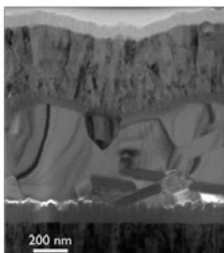
**Figure 24.** An example of interface failure, here at a  $\text{Cu}_2\text{ZnSnS}_4$ -substrate interface.<sup>75</sup> | Reproduced with permission of AIP Publishing from K. Wang et al. 2011. "Structural and Elemental Characterization of High Efficiency  $\text{Cu}_2\text{ZnSnS}_4$  Solar Cells." *Applied Physics Letters* 98 [5].
