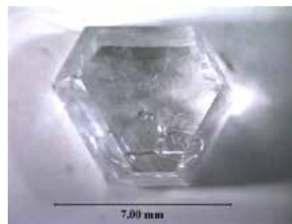
Figure 43. RBBF ( $\text{RbBe}_2\text{BO}_3\text{F}_2$ ), a new deep ultraviolet nonlinear optical crystal lasing at 175 nm. RBBF is grown under extreme conditions of hydrothermal synthesis. | Image courtesy of J. Kolis
