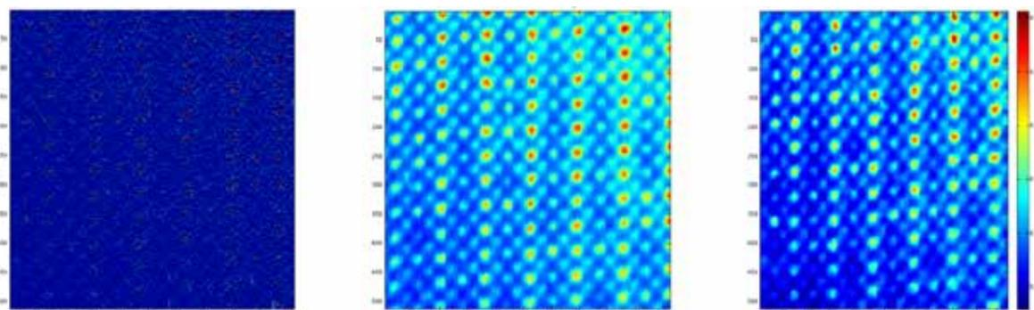
**Figure 66.** (Left) A randomly rastered STEM image using ~5% of the pixels. (Center) The full image acquired from a precise scan acquiring all the pixels. (Right) The compressive sensing reconstruction of (a) shows very good agreement with the full image.<sup>92</sup> | Image courtesy of Libor Kovarik, Pacific Northwest National Laboratory.
