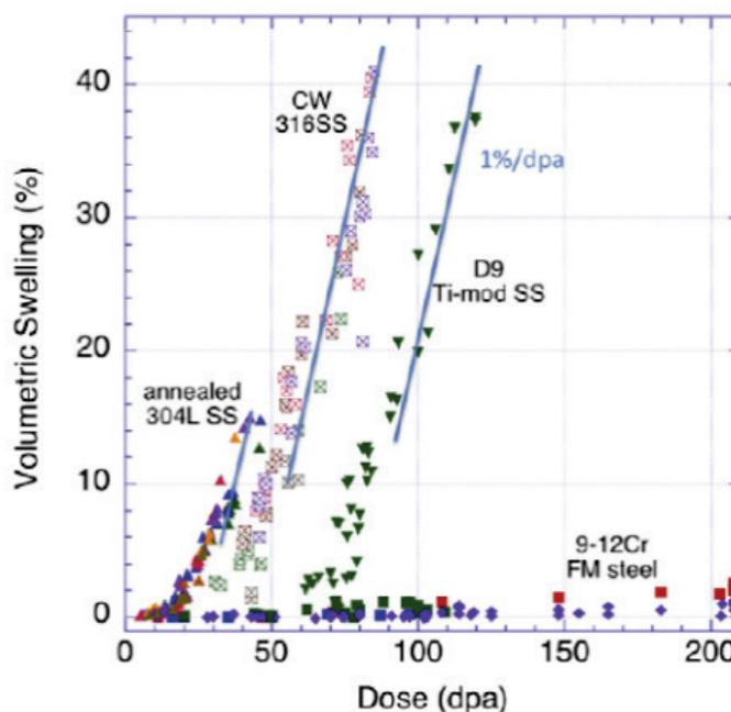
**Figure 6.** Cavity swelling in iron base cladding alloys. | Reprinted from *Acta Mater*, 61(3), S. J. Zinkle and G. S. Was, [Materials challenges in nuclear energy](#), 735–758, copyright 2013, with permission from Elsevier.
