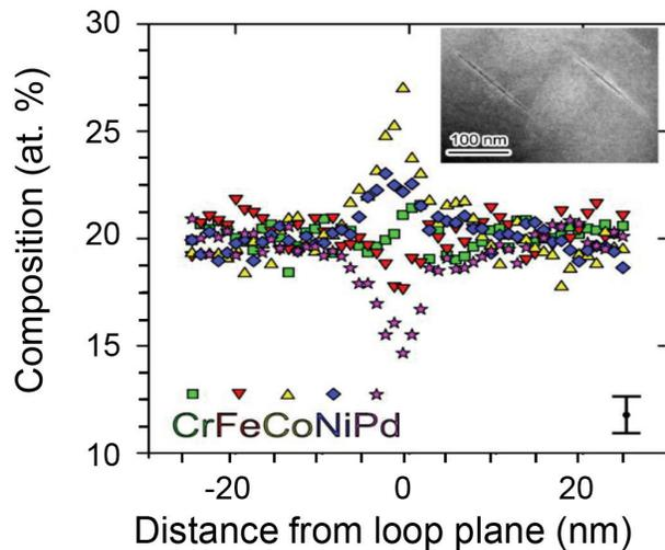
**Figure 42.** Compositional modification at an interstitial loop produced in NiCoFeCrMnPd equi-molar alloy following 1250 keV electron irradiation at 400°C. Iron and palladium are deficient and cobalt and nickel are enhanced at the loop. | Reprinted from *Acta Mater*, 126, M.-R. He et al., [Mechanisms of radiation-induced segregation in CrFeCoNi-based single-phase concentrated solid solution alloys](#), 182–193, copyright 2017, with permission from Elsevier
