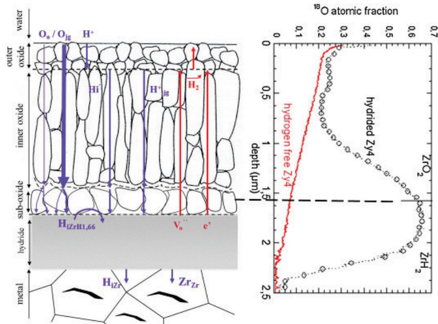
**Figure 26.** Schematic illustrating the mechanism of corrosion of zirconium hydride and impact of precipitated hydrides on Zircaloy-4 corrosion behavior. | Reprinted from *Corros. Sci.*, 98, M. Tupin et al., [Mechanism of corrosion of zirconium hydride and impact of precipitated hydrides on the Zircaloy-4 corrosion behavior](#), 478–493, copyright 2015, with permission from Elsevier
