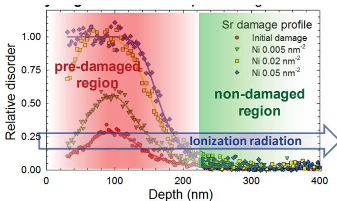
**Figure 16.** The synergistic effect of preexisting defects is illustrated: ionization leads to rapid amorphization in a defective region but no observable irradiation effects in a damage-free region. | Adapted from W. J. Weber et al. 2015. [Synergy of elastic and inelastic energy loss on ion track formation in SrTiO<sub>3</sub>](#), *Sci. Rep.* 5, 7726. Reprinted under terms and conditions of the Creative Commons license
