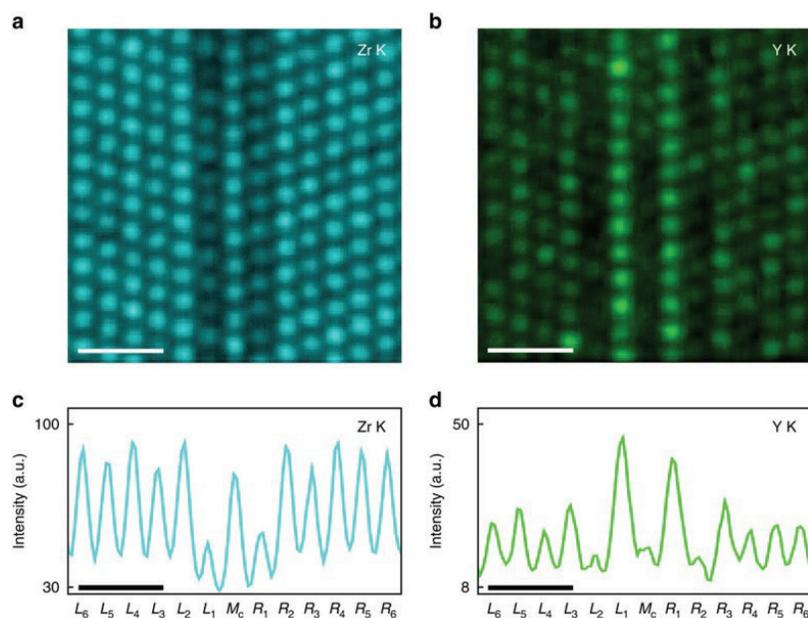
**Figure 39.** Aberration-corrected STEM energy-dispersive x-ray spectroscopy elemental maps for (a) zirconium and (b) yttrium at a grain boundary in yttria-stabilized zirconia.  $K\alpha$  emission intensity profiles for (c) zirconium and (d) yttrium. Different scales are used for the two intensity profiles. Scale bar is 1 nm. | Image courtesy of B. Feng et al. 2016. [Atomically ordered solute segregation behaviour in an oxide grain boundary](#), *Nat. Commun.* 7, 11079.
