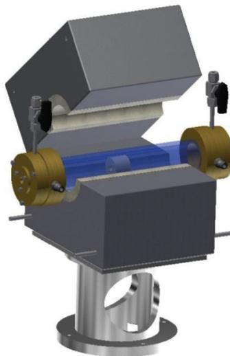
**Figure 2.** High-temperature cell for x-ray adsorption measurements of molten salts. | Reprinted from *J. Nucl. Mater.* 494, October, C. Bessada et al., [High temperature EXAFS experiments in molten actinide fluorides: The challenge of a triple containment cell for radioactive and aggressive liquids](#), 192, copyright 2017, with permission from Elsevier
