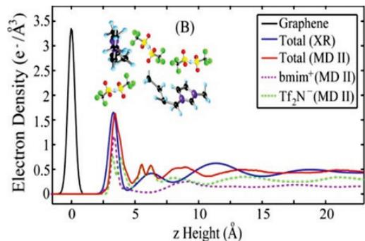
**Figure 43.** The molecular-scale vertical distribution of room-temperature ionic liquid ions at a graphene electrode under potential control obtained by x-ray reflectivity is compared directly with molecular dynamics simulations. | Reprinted with permission from H. Zhou et al. [Nanoscale perturbations of room temperature ionic liquid structure at charged and uncharged interfaces](#), ACS Nano, 6, 9812–9827, copyright 2012 American Chemical Society
