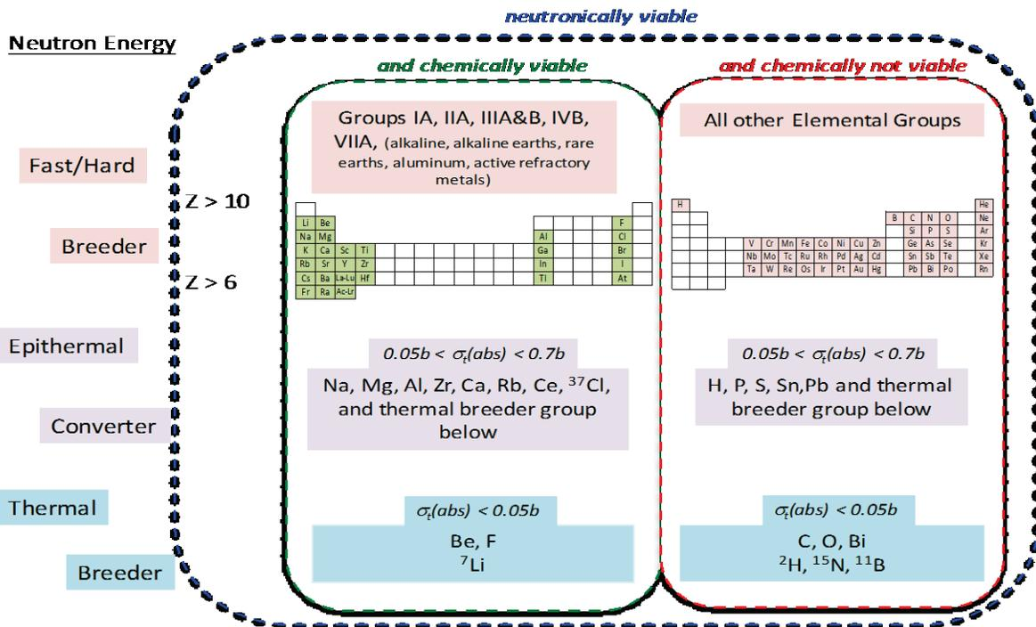
**Figure 21.** Approach to screening candidate molten salts for the MSRE (where  $\sigma_t(\text{abs})$  is total neutron absorption cross-section). | Image courtesy of Oak Ridge National Laboratory
