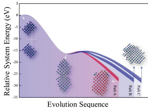
**Figure 18.** Multiple pathways of interstitial cluster evolution in bcc iron with comparable large transition states can exhibit substantial differences in the evolutionary path of the system. | Reprinted with permission from H. Xu et al. *Phys. Rev. Lett.*, 110, 2013. [Solving the puzzle of \(100\) interstitial loop formation in bcc iron](#), 265503. Copyright 2013 by the American Physical Union.
