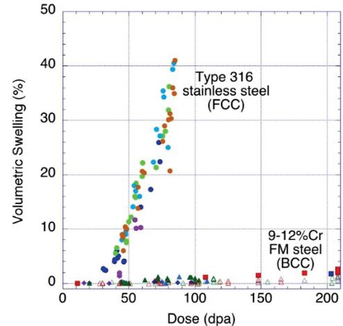
Swelling of fcc and bcc steels as a function of heavy ion dose in units of displacements per atom. | Reprinted from *Acta Mater.*, 61/3, S. J. Zinkle and G. S. Was, [Materials challenges in nuclear energy](#), 735–758, copyright 2013, with permission from Elsevier.
