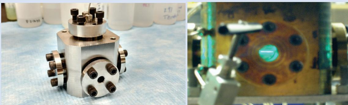
(Left) Supercritical water cell equipped with five sapphire windows allowing simultaneous irradiation and spectroscopy. (Right) Laser light transiting the cell while it is under temperature and pressure. | Images courtesy of Bruce Mincher, Idaho National Laboratory
