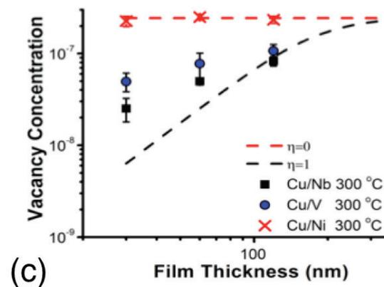
**Figure 33.** Sink efficiency  $\eta$  measured during 1.8 MeV Kr irradiations at 300°C for Cu/Nb, Cu/V, and Cu/Ni interfaces. The Cu/Nb interface is close to a perfect sink ( $\eta \approx 1$ ), Cu/Ni is close to a very poor sink ( $\eta \approx 0$ ). | Reprinted from *Acta Mater.* 82, S. Mao et al. [Quantitative comparison of sink efficiency of Cu-Nb, Cu-V and Cu-Ni interfaces for point defects](#), 328–335, copyright 2015, with permission from Elsevier
