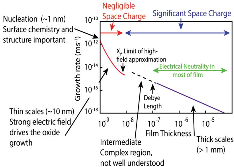
**Figure 28.** Oxide layer growth kinetics as a function of passive film thickness. 24 Cabrera and Mott theory applies for films thinner than  $X_1$  and Wagner theory applies for films thicker than the Debye length and  $X_1$ . | Reprinted with permission from A. Atkinson, [Transport processes during the growth of oxide films at elevated temperature](#), *Rev. Mod. Phys.* 57, 437, April 1, 1985. Copyright 1985 by the American Physical Society
