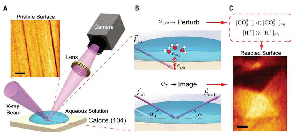
**Figure 8.** X-ray imaging of radiation-stimulated calcite dissolution. | From N. Laanaitet al. 2015. [X-ray-driven reaction front dynamics at calcite-water interfaces](#), *Science* 349(6254), 1330–1334. Reprinted with permission from AAAS
