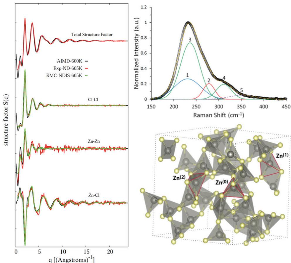
**Figure 1.** Coupled ab initio molecular dynamics with neutron diffraction and Raman vibrational spectroscopy to identify distinct polymorphs in  $\text{ZnCl}_2$  molten solutions. | Reprinted with permission from A. Alsayoud et al. 2016. [Structure of  \$\text{ZnCl}\_2\$  melt. Part I: Raman spectroscopy analysis driven by ab initio methods](#), *J. Phys. Chem. B* 120, 4174–4181. Copyright 2016 American Chemical Society
