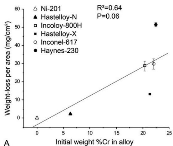
**Figure 14.** Correlation between chromium content in the alloys and weight loss due to corrosion. Samples from nickel-based alloys were exposed to FLiNaK salt at 850°C for 500 hours. | Reprinted from *Molten Salt Chemistry: From Lab to Applications*, eds. F. Lantelme and H. Grout, K. Sridharan and T. R. Allen, "Corrosion in Molten Salts, 241–267, Elsevier, Oxford, copyright 2013, with permission from Elsevier
