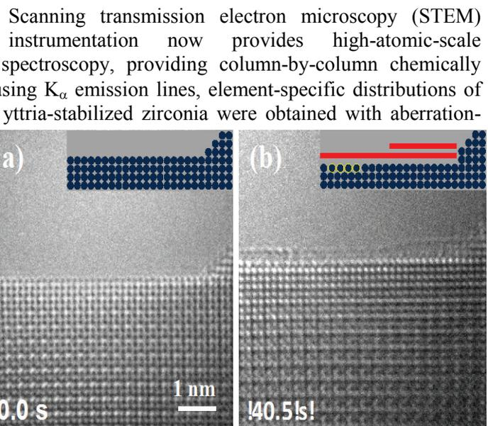
**Figure 38.** In-situ observation of oxide growth on  $\text{Ni}_3\text{Al}$  imaged at high resolution in an aberration-corrected transmission electron microscope. | Image courtesy of Guangwen Zhou, SUNY Binghamton
