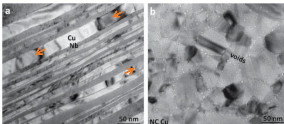
**Figure 25.** (a) Cu-Nb composites with 20 nm individual layer thickness are nearly void-free after helium ion irradiation at 450°C to 3 dpa. Arrows indicate small, isolated voids in the thicker copper layers. (b) Irradiation damage and grain growth were observed in nanocrystalline copper under identical conditions. | Images courtesy of Massachusetts Institute of Technology, W. Han, [Design of radiation tolerant materials via interface engineering](#), *Adv. Mater.*, 2013, 25, 6975–6979
