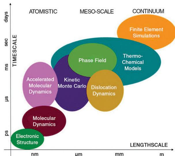
**Figure 13.** The time and length scales appropriate to different calculation modalities. | Reprinted from *Mater. Today* 12(11), M. Stan, [Discovery and design of nuclear fuels](#), 20–28, copyright 2009, with permission from Elsevier
