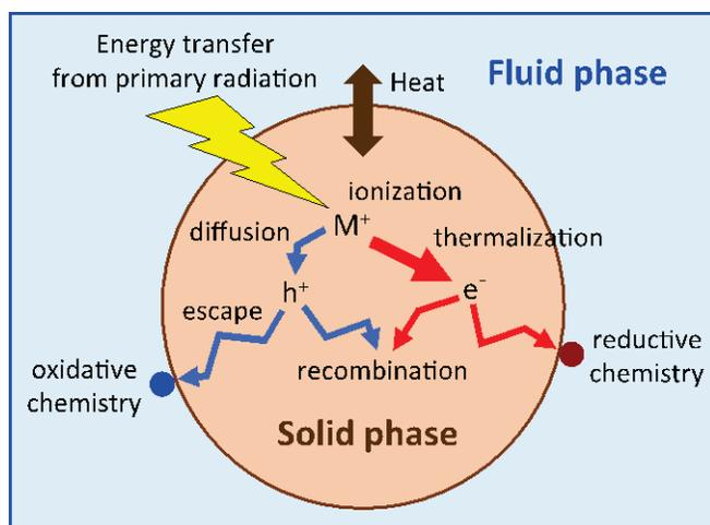
**Figure 24.** Radiolytic energy delivered near interfaces or into nanoparticles can result in higher yields of charge separation and reaction products in the surrounding fluid phase as a result of migration of radiolytic species to the interfacial region. | Image courtesy of James Wishart, Brookhaven National Laboratory
