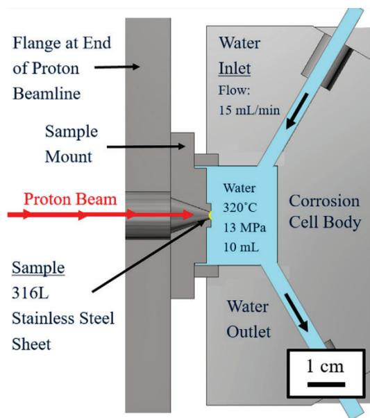
**Figure 11.** Proton beam irradiation of 316L stainless steel while exposed to high-temperature water with added hydrogen to study the effect of radiation on corrosion. | Reprinted from J. Nucl. Mater. 493, S. S. Raiman and G. S. Was, [Accelerated corrosion and oxide dissolution in 316L stainless steel irradiated in situ in high temperature water](#), 207–218, copyright 2017, with permission from Elsevier
