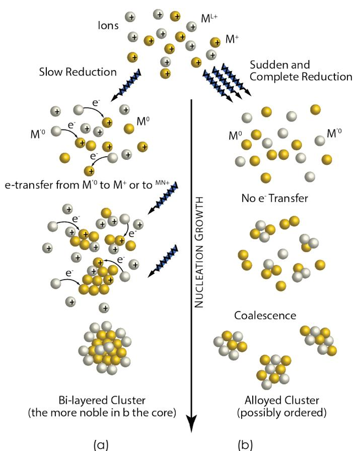
**Figure 5.** Radiation pathway for nanoparticle and alloy synthesis. | Reprinted from *Catal. Today* 113(3–4), J. Belloni, [Nucleation, growth, and properties of nanoclusters studied by radiation chemistry: Application to catalysis](#), 141–156, copyright 2006, with permission from Elsevier
