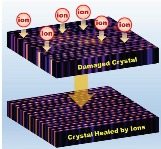
**Figure 17.** Bombarding a material with energetic charged particles can heal, rather than damage, the crystalline structure of SiC through local heating. | Reprinted from Y. Zhang et al. 2015. [Ionization-induced annealing of pre-existing defects in silicon carbide](#). *Nat. Commun.* 6, 8049, under terms and conditions of the Creative Commons license.
