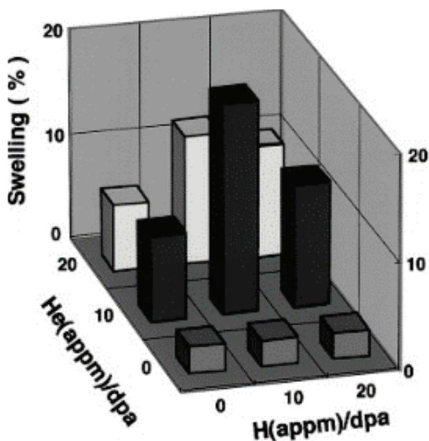
**Figure 29.** Synergistic effects of helium and hydrogen ion beam irradiation leading to swelling. | Reprinted from *J. Nucl. Mater.*, 283–287, Part 1, N. Sekimura et al., [Synergistic effects of hydrogen and helium on microstructural evolution in vanadium alloys by triple ion beam irradiation](#), 224–228, copyright 2000, with permission from Elsevier
