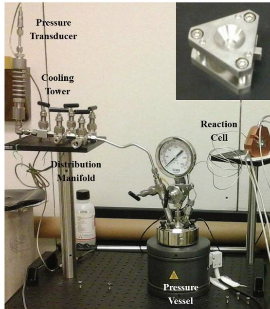
**Figure 9.** Corrosion-resistant apparatus for high-pressure and high-temperature x-ray studies. | Reproduced from M. S. Elbakhshwan et al. 2016. "Sample environment for in situ synchrotron corrosion studies of materials in extreme environments," *Rev. Sci. Instrum.* 87, 105122, with permission of AIP Publishing
