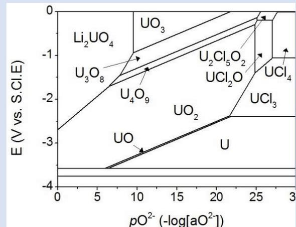
Predominance diagrams of U, in NaCl-KCl at 750°C. | Reprinted from R. Abdulaziz et al. 2016. Predominance diagrams of spent nuclear fuel materials in LiCl-KCl and NaCl-KCl molten salt eutectics, | *Int. J. Electrochem. Sci.* 11, 10417-10435. Image courtesy of *Int. J. Electrochem. Sci.* under the terms and conditions of the Creative Commons license
