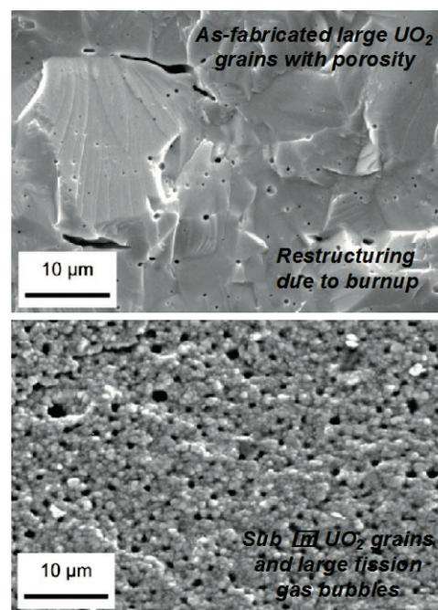
**Figure 32.** Illustration of microstructural changes in traditional fuel ( $\text{UO}_2$ ) that defy current predictive capability. | Reprinted from *Mater. Today*, V. Rondinella et al., [The high burn-up structure in nuclear fuel](#), 24-32, copyright 2010, with permission from Elsevier
