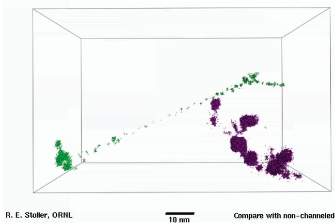
**Figure 15.** Comparison of defect production in two nominally equivalent high-energy displacement cascades in iron (shown separately in green and purple). | Image courtesy of R. E. Stoller, Oak Ridge National Laboratory
