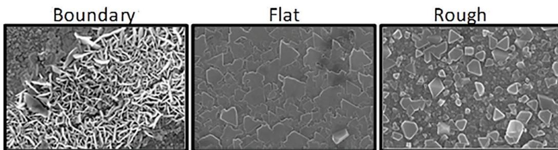
**Figure 41.** The corrosion morphology changes depending on the surface orientation to the environment or the grain boundary orientation. Systematic design of the overall material structure could better control the stability of the overall oxide, thus extending component lifetime. | Image courtesy of Todd Allen, University of Wisconsin–Madison
