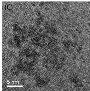
Figure 35. d-UO<sub>2</sub> NPs at pH=3, with 7 days irradiation. | Image courtesy of T. M. Nenoff et al. [Synthesis and low temperature in situ sintering of uranium oxide nanoparticles](#), *Chem. Mater.* 2011, 23(3), 5185–5190, copyright 2011 American Chemical Society
