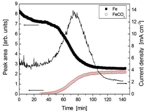
**Figure 12.** Plot of current density (light line) during siderite growth on iron as monitored by in situ x ray diffraction (heavy lines). | Reproduced from B. Ingham et al., 2015, [First stages of siderite crystallisation during CO<sub>2</sub> corrosion of steel evaluated using in situ synchrotron small- and wide-angle x-ray scattering](#), *Faraday Discuss.* 180(0), 171–190, with permission of The Royal Society of Chemistry
