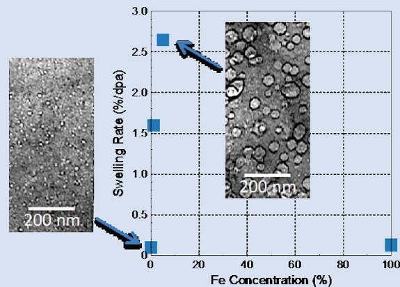
Sensitivity of radiation damage to V-Fe BCC alloy composition. | Reprinted from *J. Nucl. Mater.*, 258–263, K. Fukumoto et al. [Swelling behavior of V-Fe binary and V-Fe-Ti ternary alloys](#), 1431–1436, copyright 1998, with permission from Elsevier.
