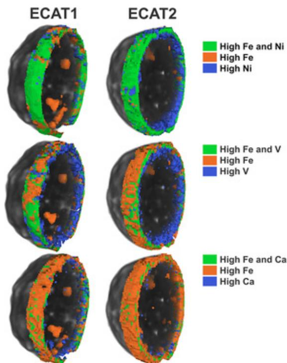
Figure 21. Two dimensional slices for each elemental channel of the two different FCC catalyst particles. From Kalirai S., U. Boesenberg, G. Falkenberg, F. Meirer, and B. Weckhuysen, *ChemCatChem*, 2015, 7: 3674–3682. Copyright Wiley-VCH Verlag GmbH & Co. KGaA (NonCommercial 4.0 International [CC BY-NC 4.0]).
