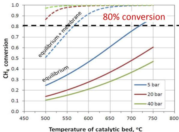
**Figure 22.** Predicted  $\text{CH}_4$  conversion achieved for SMR as a function of temperature and pressure with and without a  $\text{H}_2$  membrane. From Saric (2015). Reproduced with permission.
