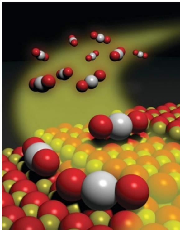
**Figure 16.** When exposed to high temperature in air, platinum desorbs from Pt nanocrystals as PtO<sub>2</sub> (grey and red), and can be trapped on CeO<sub>2</sub> (gold and red). Figure from Jacoby 2016; courtesy of Abhaya Datye (University of New Mexico); artist Cortland Lewis (Pacific Northwest National Laboratory).
