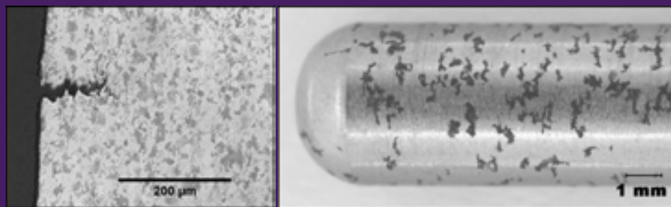
Different forms of steel corrosion after testing in a tank waste simulant (left to right): environmental cracking, pitting corrosion, and liquid-air interface corrosion (Brossia et al. 2007a and 2007b). Left: Image courtesy of DOE; right: image courtesy of DOE Office of River Protection.
