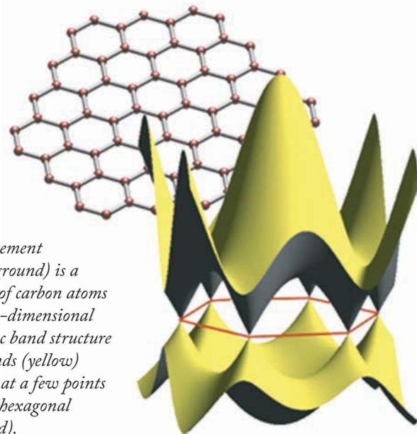
*The atomic arrangement of graphene (background) is a honeycomb lattice of carbon atoms arranged in a two-dimensional plane. Its electronic band structure consists of two bands (yellow) that intersect only at a few points at the corners of a hexagonal Brillouin zone (red).*
