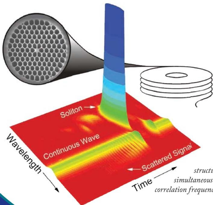
*Inelastic scattering of a continuous wave on a femtosecond soliton in a nanostructured photonic crystal fiber, observed with simultaneous time and spectral resolution using cross-correlation frequency resolved optical gating techniques.*
