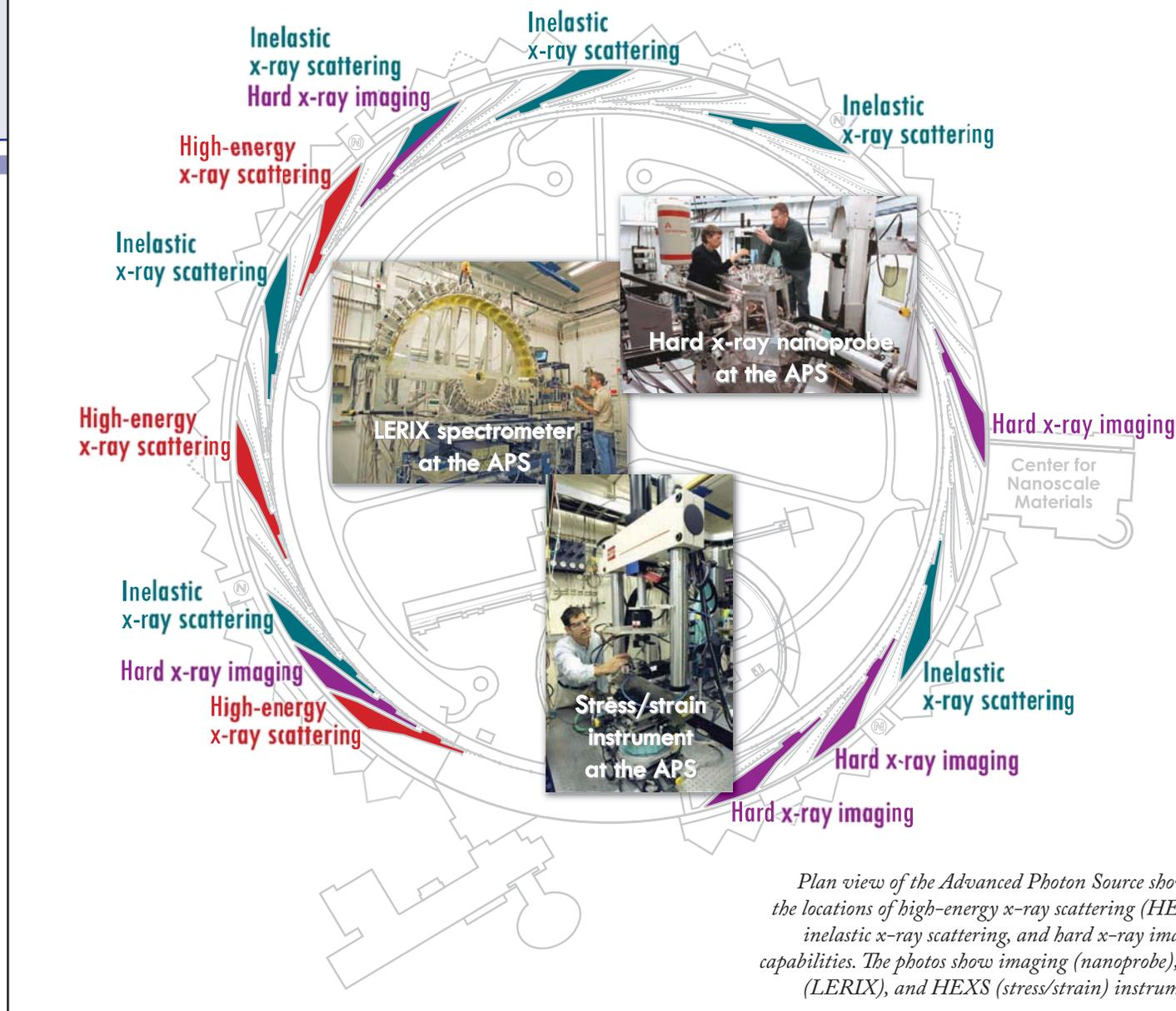
Plan view of the Advanced Photon Source showing the locations of high-energy x-ray scattering (HEXS), inelastic x-ray scattering, and hard x-ray imaging capabilities. The photos show imaging (nanoprobe), IXS (LERIX), and HEXS (stress/strain) instruments.
