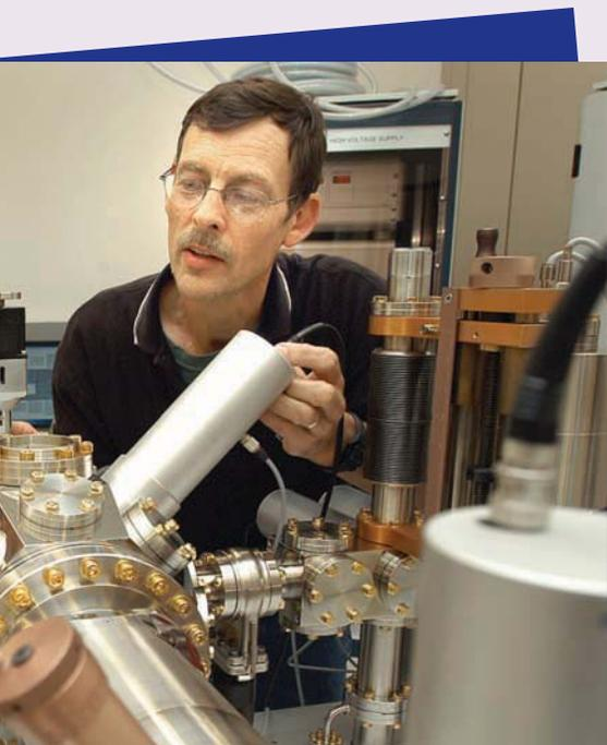
*Lights, Camera, Action!* CFN user Professor Peter Bennett of Arizona State University (at right) and facility scientist Peter Sutter (at left) align the CFN's low-energy electron microscope, a unique tool for capturing real-time movies of dynamic surface processes at the nanometer scale.
