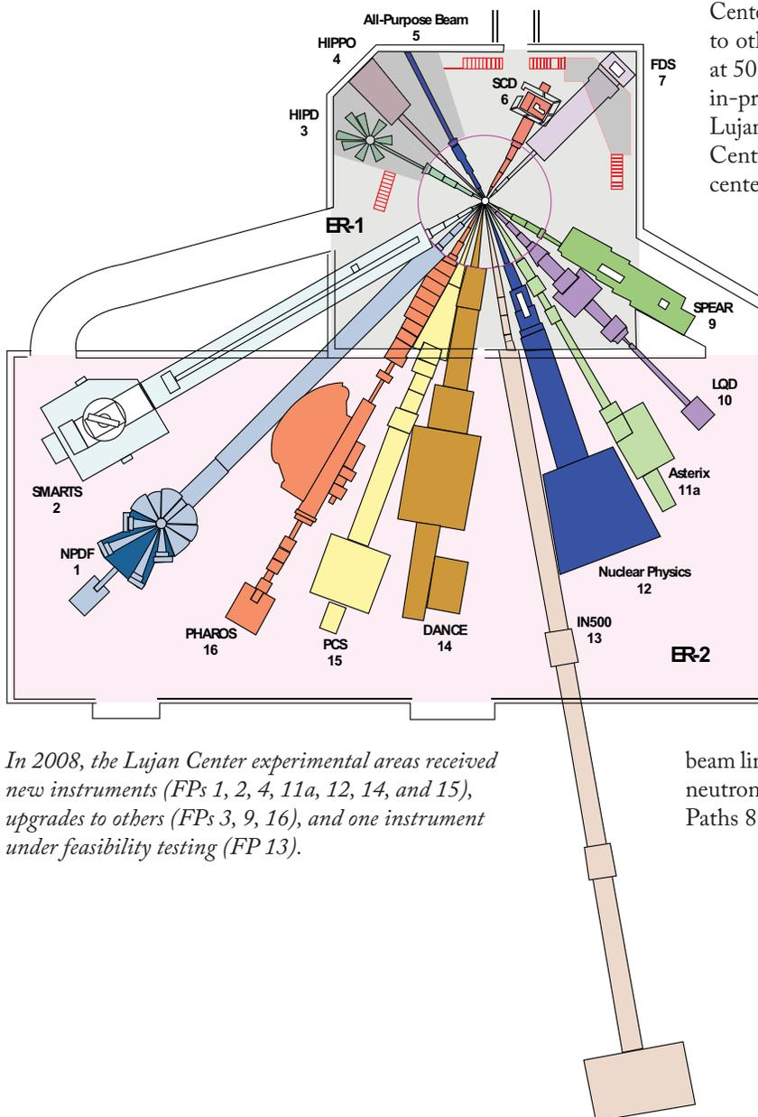
*In 2008, the Lujan Center experimental areas received new instruments (FPs 1, 2, 4, 11a, 12, 14, and 15), upgrades to others (FPs 3, 9, 16), and one instrument under feasibility testing (FP 13).*
