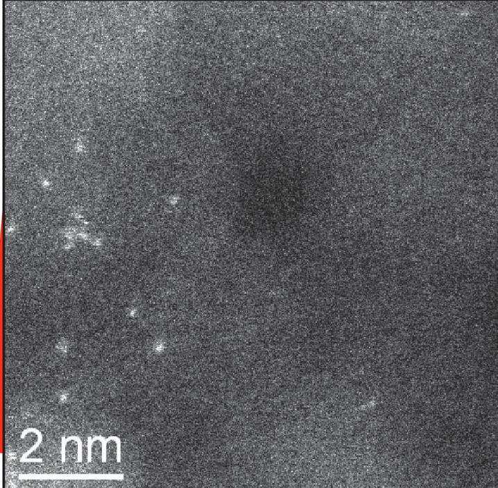
A high-resolution transmission electron microscopy (HRTEM) image showing platinum (Pt) atoms and clusters. The image is a grayscale micrograph with a dark background. Numerous small, bright white dots are scattered across the field, representing individual Pt atoms. In some areas, these dots are grouped together to form small, irregular clusters. A white scale bar is located in the bottom right corner of the image, labeled '2 nm'.
