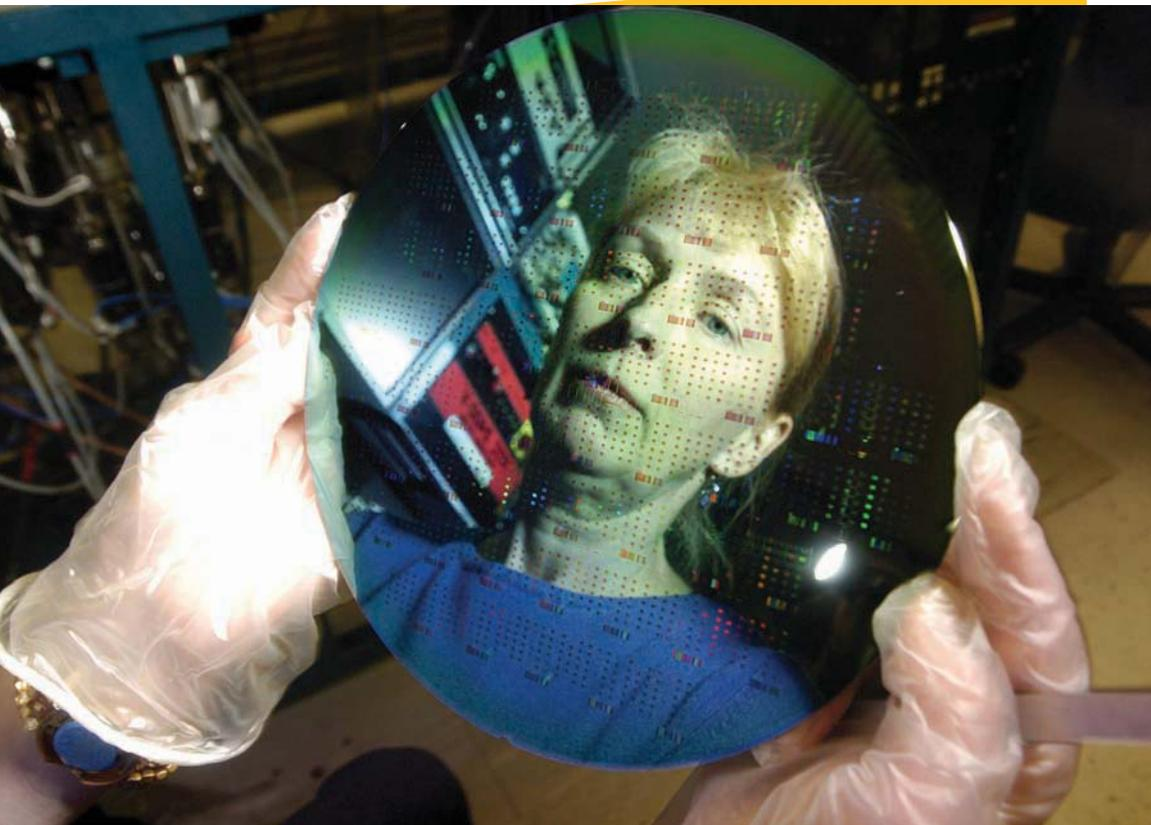
*IBM researcher Simone Raoux with a wafer that contains millions of new computer memory switches. Raoux performs research partly with time-resolved x-ray diffraction at the NSLS to develop a material that could lead to a new kind of computer memory chip used for storing digital media. Photo courtesy of Noah Berger/The New York Times/Redux.*
