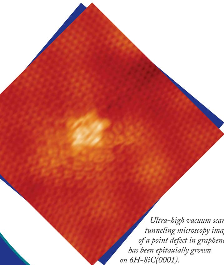
*Ultra-high vacuum scanning tunneling microscopy image of a point defect in graphene that has been epitaxially grown on 6H-SiC(0001).*
