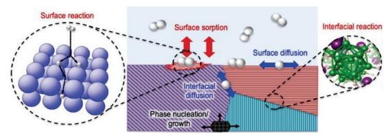
**Figure 2-4**. Illustration of some of the key surface and interface processes taking place during cycling of a typical nanoscale metal hydride material.<sup>59</sup> Reprinted with permission: B. Wood, et al., *Industrial & Engineering Chemistry Research*, **59** 5786-5796 (2020). Copyright 2020, American Chemical Society.
