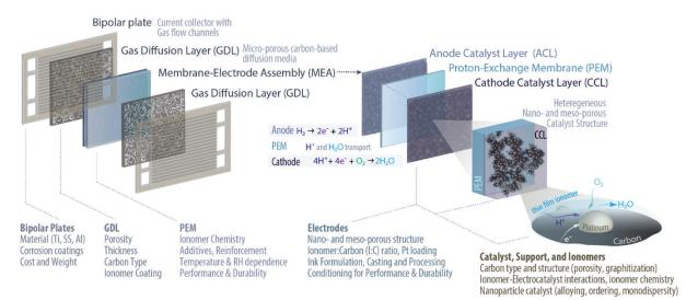
**Figure 4-5.** Representation of a PEMFC stack showing components and complexity of a functioning device including bipolar plates, gas diffusion layer, PEM, and electrodes.<sup>7</sup> Reprinted with permission: <u>D.A. Cullen, et al., Nature Energy</u>, **6** 462-474 (2021) Copyright 2021.
