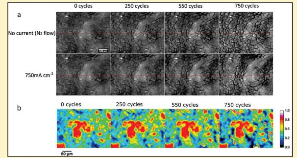
**Figure S8-1.** Morphology changes of PEMFC catalyst layer during voltage cycling using operando X-ray CT. (A) In-plane gray-scale tomographs show crack evolution with cycling for dry (*top*) and wet (*bottom*) conditions. (B) Color-coded porosity of cathode layer at 0 cycles and after 250, 550 and 750 cycles.<sup>98</sup> Reprinted with permission: R.T. White, et al., *Scientific Reports*, **9** 1843 (2019) under Creative Commons Attribution 4.0 International (CC BY 4.0). Copyright 2019.
