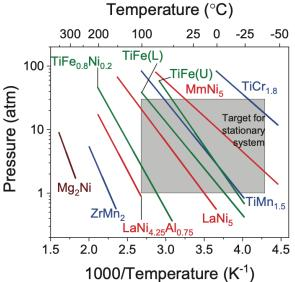
**Figure 2-3.** van't Hoff plots showing a wide range of hydrogen interaction energies measured in interstitial metal hydrides with estimated targets for stationary applications.<sup>40</sup> Image reprinted from <u>Modi and Aguey-Zinsou</u>, <u>Front. Energy Res.</u> under <u>Creative Commons</u> <u>Attribution 4.0 International (CC BY 4.0)</u>. Copyright © 2021 Modi and Aguey-Zinsou.
