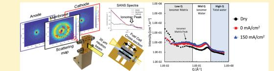
**Figure S7-2.** Schematic of operando small-angle neutron scattering of an operating fuel cell and representative scattering data showing evolution of the structure of the fuel cell membrane with cell current.<sup>97</sup> Reprinted with permission: J. Lee, et al., ACS Applied Energy Materials, **3** 8393-8401 (2020), Copyright 2020, American Chemical Society.
