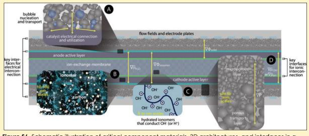
**Figure S6.** Schematic illustration of critical component materials, 3D architectures, and interfaces in a PEM electrolyzer. Key driving forces leading to bulk and interface reactions and transport processes are shown in each panel (A–D) and discussed above. Image used with permission from Shannon Boettcher, University of Oregon.
