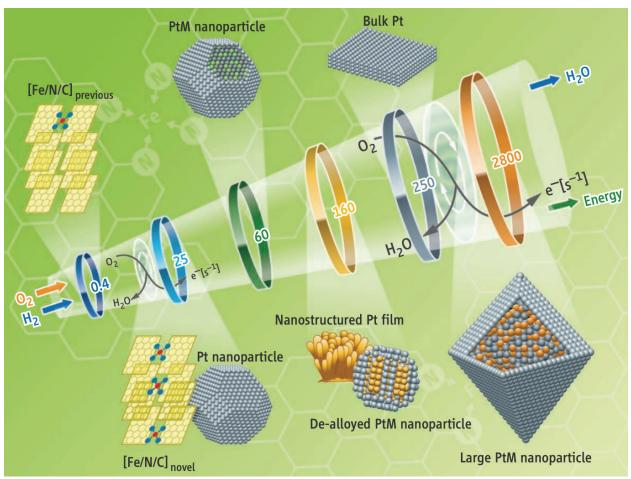
**Figure 4-4.** Illustration of different model oxygen reduction reaction electrocatalysts with increasing turnover frequencies targeting improved electrocatalytic performance.<sup>111</sup> Illustration by Aaron Ashley.
