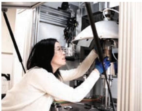
**Synthesizing New Materials at High Pressure.** Staff scientist Hong Zheng prepares to grow crystals in the extreme conditions of Argonne National Laboratory's (ANL) high-pressure floating zone furnace. The high temperatures and pressures produced by the furnace enable the discovery of new quantum materials that cannot be grown under ambient conditions. [Courtesy ANL]
