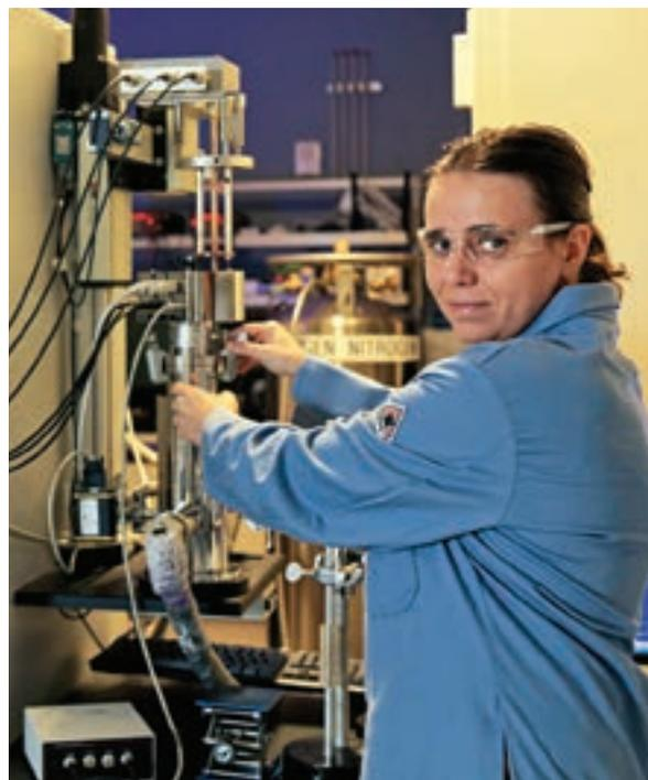
**Developing Complex Materials with Enhanced Properties.** Vera Bocharova, of Oak Ridge National Laboratory (ORNL), performs broadband dielectric spectroscopy, a technique capable of capturing a variety of material synthesis mechanisms and phenomena by probing temperature-dependent dynamics on time scales from  $10^{-8}$  to 100 seconds. [Courtesy ORNL]
