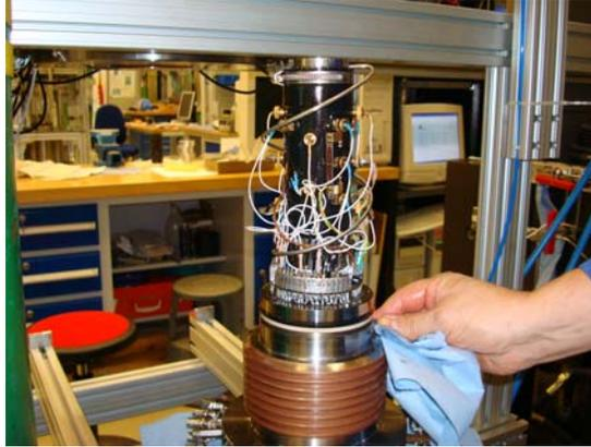
Figure 1. Sample assembly. The PZT transducers are installed along the cylindrical surface of the sample.
