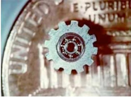
*LIGA-micromachined gear for a miniature electromagnetic motor.*
