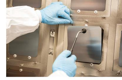
Commercial-sized perovskite-silicon solar cells that are nearing commercial production. (Oxford PV)
