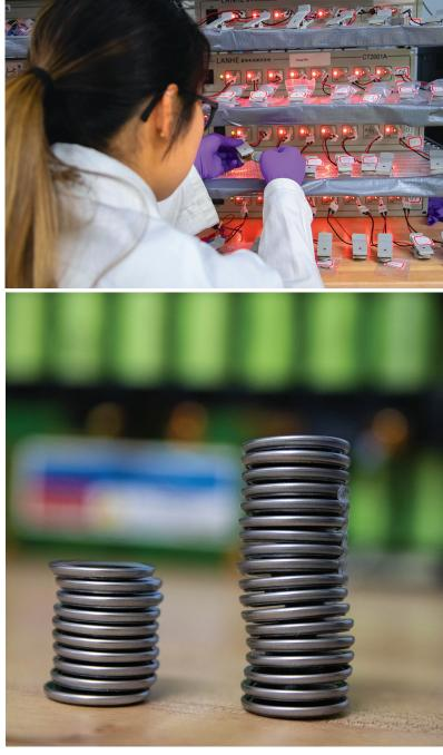
*Top:* Dr. Siu conducts electrochemical tests on potential battery materials. *Bottom:* The lefthand stack of battery cells made of a novel cathode material has the same energy storage capacity as the righthand stack of cells used in the current generation of batteries. *(Marc Francis Hidalgo)*
