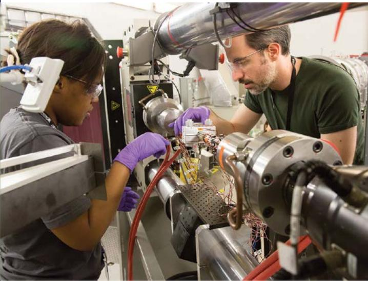
Top: Protons accelerated by this underground linear accelerator at Oak Ridge National Laboratory are collided with a mercury target, generating high-energy pulses of neutrons that are directed into multiple beamlines for research into the properties of materials. *(Genevieve Martin / Oak Ridge National Laboratory)*
