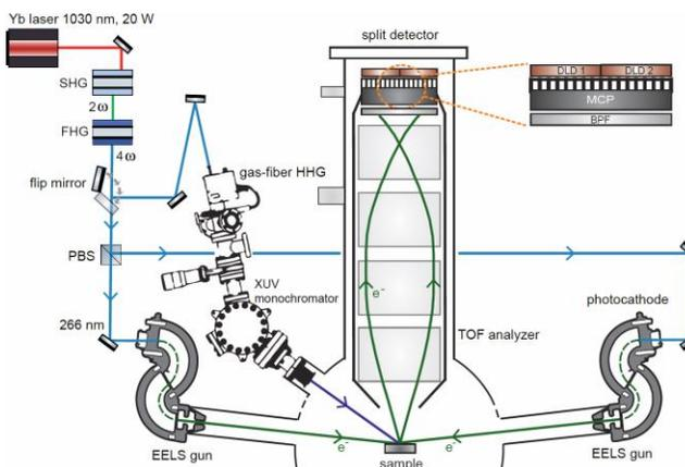
**Figure 2** Conceptual illustration of a two-electron, time-of-flight, Einstein-Podolsky-Rosen spectrometer, which uses coherent pairs of electrons to detect valence band phenomena in quantum materials.
