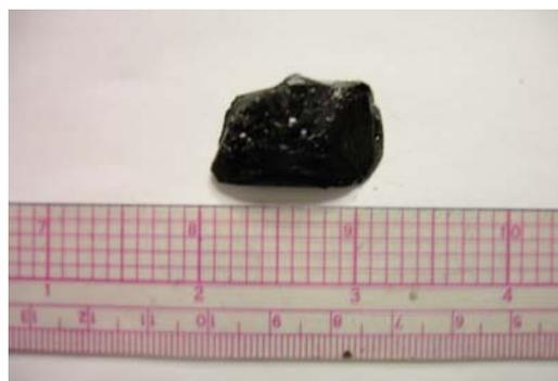
Fig. 4: YbRh<sub>2</sub>Si<sub>2</sub> single crystals for INS measurements
