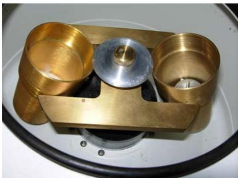
Fig. 3: Centrifuge system for 50 ml crucibles
