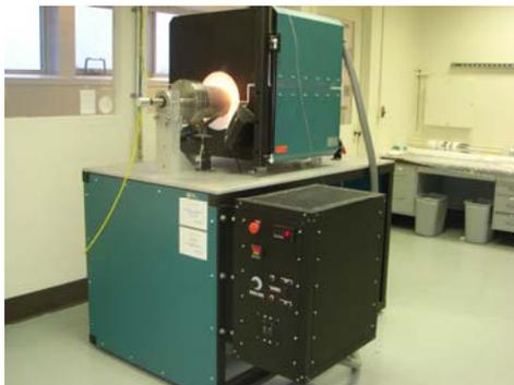
Fig. 1: In-situ decanting high T flux furnace
