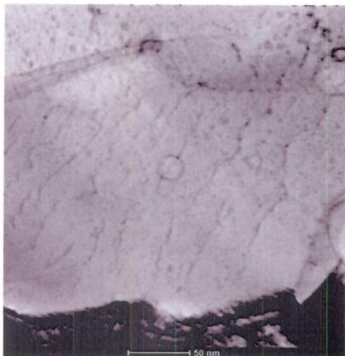
Fig.2 Bright field STEM image of a grain containing dislocations in the 14YWT alloy following deformation at 950°C. The dislocations exhibit numerous cusps along their lengths, and evidence for direct pinning on the nanoclusters. The dislocations appear to be bowed in the same direction, suggesting difficult movement through the dense field of nanoclusters.
