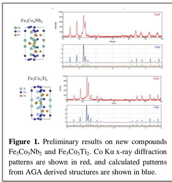
**Figure 1.** Preliminary results on new compounds  $\text{Fe}_3\text{Co}_3\text{Nb}_2$  and  $\text{Fe}_3\text{Co}_3\text{Ti}_2$ . Co  $K\alpha$  x-ray diffraction patterns are shown in red, and calculated patterns from AGA derived structures are shown in blue.
