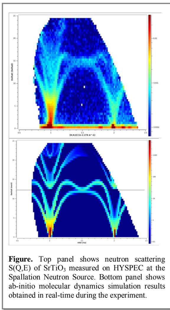
**Figure.** Top panel shows neutron scattering  $S(Q, E)$  of  $\text{SrTiO}_3$  measured on HYSPEC at the Spallation Neutron Source. Bottom panel shows ab-initio molecular dynamics simulation results obtained in real-time during the experiment.
