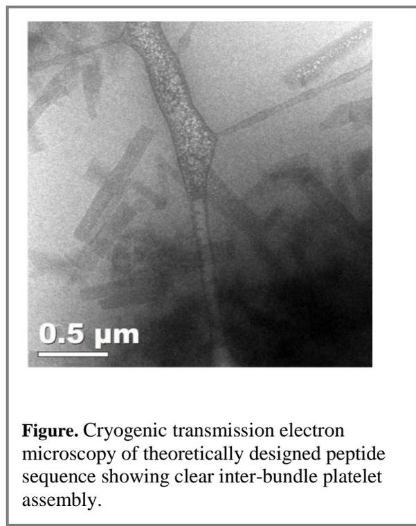
**Figure.** Cryogenic transmission electron microscopy of theoretically designed peptide sequence showing clear inter-bundle platelet assembly.
