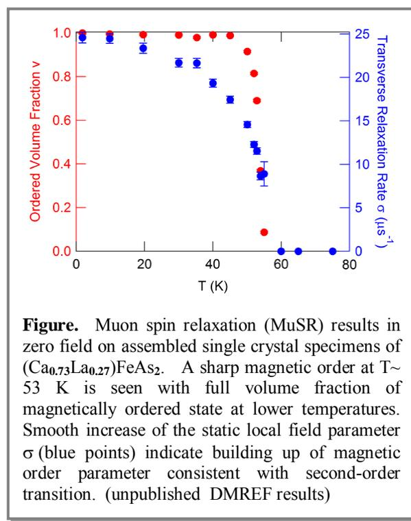
**Figure.** Muon spin relaxation (MuSR) results in zero field on assembled single crystal specimens of  $(\text{Ca}_{0.73}\text{La}_{0.27})\text{FeAs}_2$ . A sharp magnetic order at  $T \sim 53$  K is seen with full volume fraction of magnetically ordered state at lower temperatures. Smooth increase of the static local field parameter  $\sigma$  (blue points) indicate building up of magnetic order parameter consistent with second-order transition. (unpublished DMREF results)
