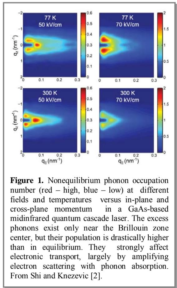
**Figure 1.** Nonequilibrium phonon occupation number (red – high, blue – low) at different fields and temperatures versus in-plane and cross-plane momentum in a GaAs-based midinfrared quantum cascade laser. The excess phonons exist only near the Brillouin zone center, but their population is drastically higher than in equilibrium. They strongly affect electronic transport, largely by amplifying electron scattering with phonon absorption. From Shi and Knezevic [2].
