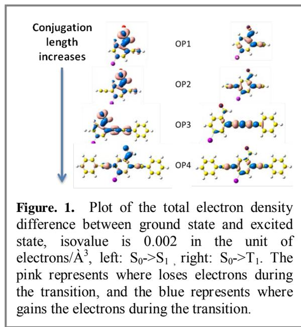
**Figure 1.** Plot of the total electron density difference between ground state and excited state, isovalue is 0.002 in the unit of electrons/ $\text{\AA}^3$ , left:  $S_0 \rightarrow S_1$ , right:  $S_0 \rightarrow T_1$ . The pink represents where loses electrons during the transition, and the blue represents where gains the electrons during the transition.
