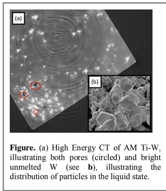
**Figure.** (a) High Energy CT of AM Ti-W, illustrating both pores (circled) and bright unmelted W (see b), illustrating the distribution of particles in the liquid state.
