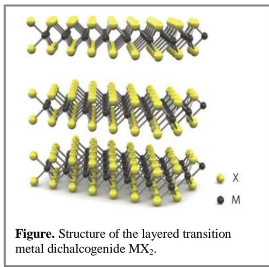
**Figure.** Structure of the layered transition metal dichalcogenide  $\text{MX}_2$ .
