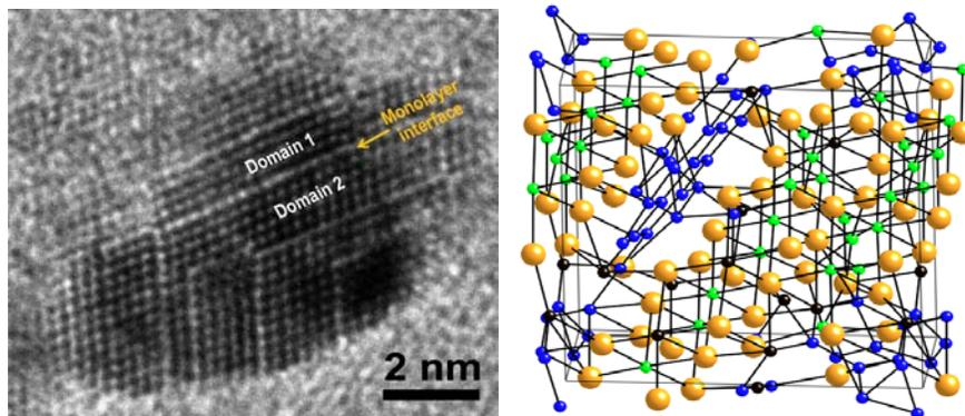
**Figure 2.** HRTEM image of a nano needle in the Zr<sub>41</sub>B<sub>30</sub>C<sub>8</sub>N<sub>20</sub> film showing nano domains separated by monolayer interfaces and the simulated structure for Zr<sub>42</sub>B<sub>32</sub>C<sub>8</sub>N<sub>18</sub> resembling the experimental structure.
