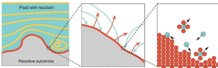
**Figure 1:** Schematic representation of the scales involved in the reactivity of nanoporous catalysts, from the macroscopic (fluid flow regime) to the mesoscopic (transport of reactants and products to/from surfaces) to the microscopic (atomic-scale reactions).
