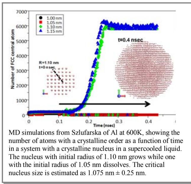
MD simulations from Szlufarska of Al at 600K, showing the number of atoms with a crystalline order as a function of time in a system with a crystalline nucleus in a supercooled liquid. The nucleus with initial radius of 1.10 nm grows while one with the initial radius of 1.05 nm dissolves. The critical nucleus size is estimated as 1.075 nm  $\pm$  0.25 nm.
