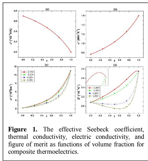
**Figure 1.** The effective Seebeck coefficient, thermal conductivity, electric conductivity, and figure of merit as functions of volume fraction for composite thermoelectrics.
