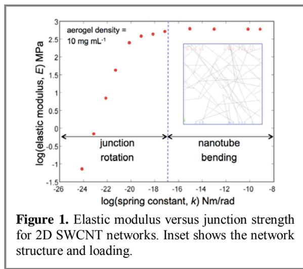
**Figure 1.** Elastic modulus versus junction strength for 2D SWCNT networks. Inset shows the network structure and loading.
