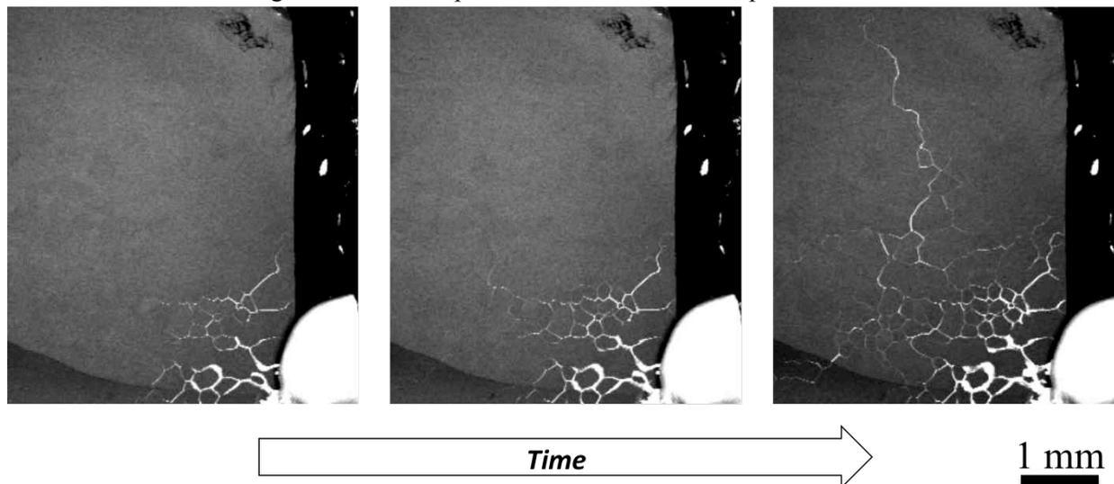
**Fig. 1:** Time-lapse sequence of an *in situ* Ga permeation experiment. The Ga reservoir is at the bottom right corner. Note the high diffusivity GB path that branches out from the initial cluster of wetted GBs in the last frame on the right.
