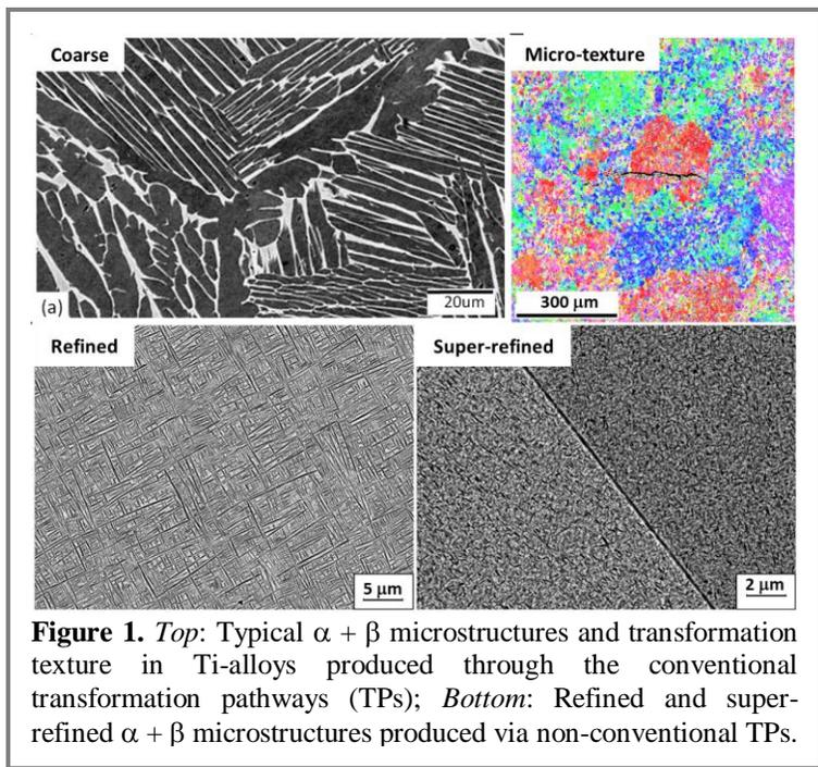
**Figure 1.** *Top:* Typical  $\alpha + \beta$  microstructures and transformation texture in Ti-alloys produced through the conventional transformation pathways (TPs); *Bottom:* Refined and super-refined  $\alpha + \beta$  microstructures produced via non-conventional TPs.
