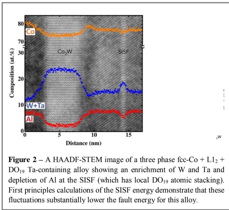
**Figure 2** – A HAADF-STEM image of a three phase fcc-Co +  $L1_2$  +  $DO_{19}$  Ta-containing alloy showing an enrichment of W and Ta and depletion of Al at the SISF (which has local  $DO_{19}$  atomic stacking). First principles calculations of the SISF energy demonstrate that these fluctuations substantially lower the fault energy for this alloy.
