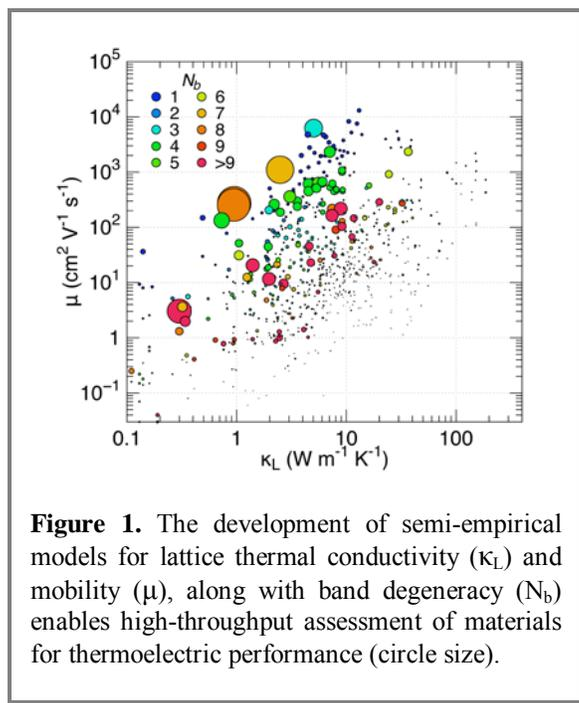
**Figure 1.** The development of semi-empirical models for lattice thermal conductivity ( $\kappa_L$ ) and mobility ( $\mu$ ), along with band degeneracy ( $N_b$ ) enables high-throughput assessment of materials for thermoelectric performance (circle size).
