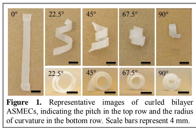
**Figure 1.** Representative images of curled bilayer ASMECs, indicating the pitch in the top row and the radius of curvature in the bottom row. Scale bars represent 4 mm.
