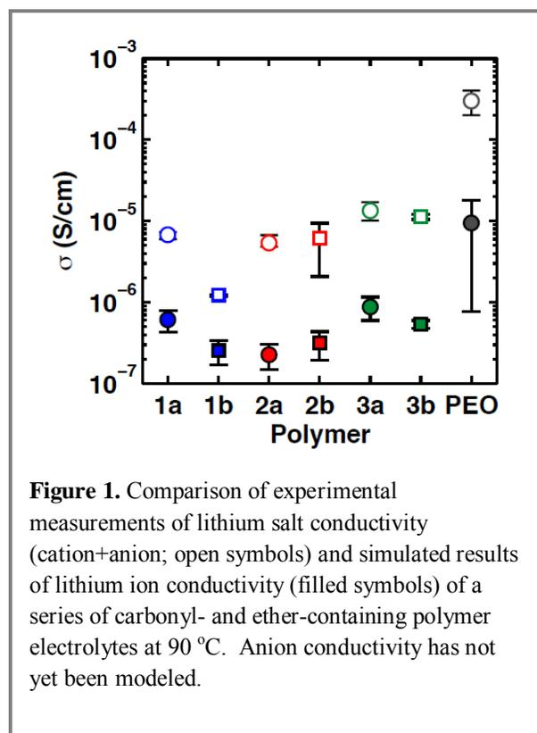
**Figure 1.** Comparison of experimental measurements of lithium salt conductivity (cation+anion; open symbols) and simulated results of lithium ion conductivity (filled symbols) of a series of carbonyl- and ether-containing polymer electrolytes at 90 °C. Anion conductivity has not yet been modeled.
