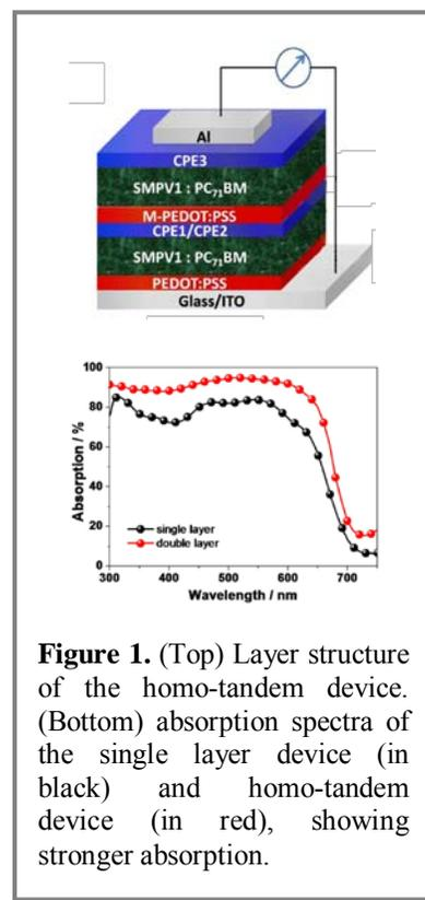
**Figure 1.** (Top) Layer structure of the homo-tandem device. (Bottom) absorption spectra of the single layer device (in black) and homo-tandem device (in red), showing stronger absorption.
