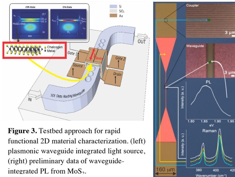
**Figure 3.** Testbed approach for rapid functional 2D material characterization. (left) plasmonic waveguide integrated light source, (right) preliminary data of waveguide-integrated PL from MoS<sub>2</sub>.
