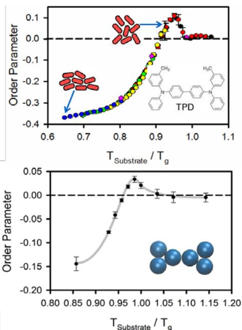
**Figure 2.** Molecular orientation in PVD glasses can be controlled by the substrate temperature (upper panel). Molecular orientation can increase the efficiency of organic electronics such as OLEDs. Computer simulations reproduce the experimental trends and explain the result in terms of preferred orientation at the surface of the equilibrium liquid and the ability to reach local equilibrium at a given substrate temperature (lower panel).
