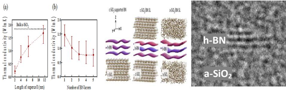
**Figure 1.** Molecular dynamics predictions of the cross-plane thermal conductivity as a function of the number of BN layers, which are embedded in an amorphous-SiO<sub>2</sub> (left) indicate flattening above 3-layers (middle). HRTEM image (right) of the corresponding synthesized h-BN SiO<sub>2</sub> structure.
