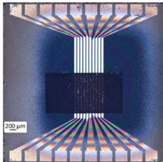
**Figure 1.** Optical image of ten element heater array
