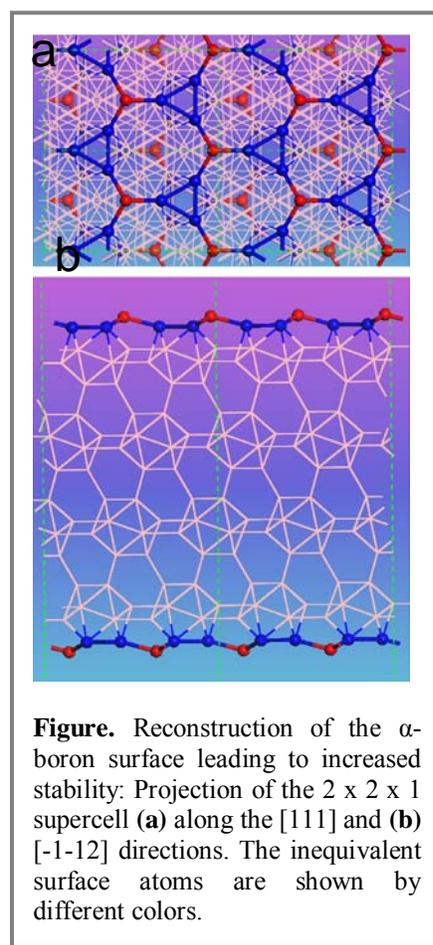
**Figure.** Reconstruction of the  $\alpha$ -boron surface leading to increased stability: Projection of the  $2 \times 2 \times 1$  supercell (a) along the [111] and (b) [-1-12] directions. The inequivalent surface atoms are shown by different colors.
