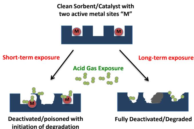
**Figure 1:** Changes induced in sorbents/catalysts upon short- and long-term exposure to acid gases. Materials are typically treated as passive in these environments, but can change dramatically upon exposure to  $\text{SO}_x$ ,  $\text{NO}_x$ , and  $\text{H}_2\text{S}$ .
