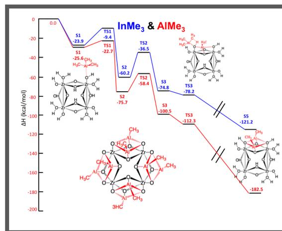
**Atomic layer deposition of Group III metals:** The NU-1000 core has four distinct faces, two exposed to large pores and two exposed to small pores. InMe<sub>3</sub> and AlMe<sub>3</sub> react with exposed OH groups to deposit eight metal atoms in a structure predicted by theory and confirmed by X-ray powder diffraction.
