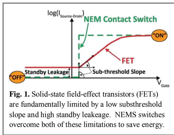
**Fig. 1.** Solid-state field-effect transistors (FETs) are fundamentally limited by a low subthreshold slope and high standby leakage. NEMS switches overcome both of these limitations to save energy.
