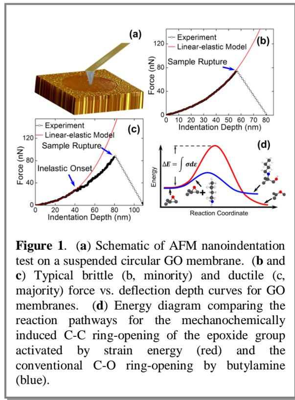
**Figure 1.** (a) Schematic of AFM nanoindentation test on a suspended circular GO membrane. (b and c) Typical brittle (b, minority) and ductile (c, majority) force vs. deflection depth curves for GO membranes. (d) Energy diagram comparing the reaction pathways for the mechanochemically induced C-C ring-opening of the epoxide group activated by strain energy (red) and the conventional C-O ring-opening by butylamine (blue).
