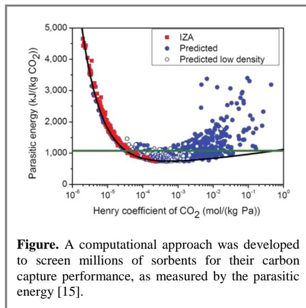
**Figure.** A computational approach was developed to screen millions of sorbents for their carbon capture performance, as measured by the parasitic energy [15].
