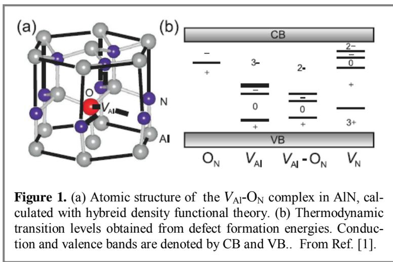
**Figure 1.** (a) Atomic structure of the  $V_{Al}-O_N$  complex in AlN, calculated with hybrid density functional theory. (b) Thermodynamic transition levels obtained from defect formation energies. Conduction and valence bands are denoted by CB and VB. From Ref. [1].
