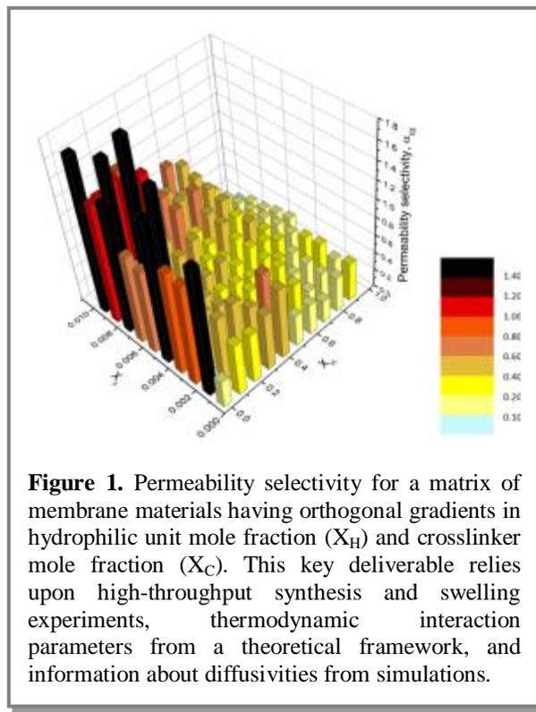
**Figure 1.** Permeability selectivity for a matrix of membrane materials having orthogonal gradients in hydrophilic unit mole fraction ( $X_H$ ) and crosslinker mole fraction ( $X_C$ ). This key deliverable relies upon high-throughput synthesis and swelling experiments, thermodynamic interaction parameters from a theoretical framework, and information about diffusivities from simulations.
