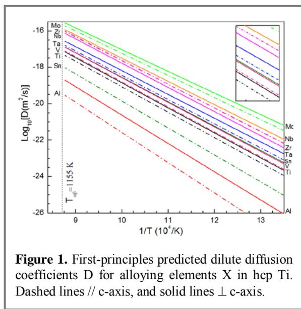
**Figure 1.** First-principles predicted dilute diffusion coefficients D for alloying elements X in hcp Ti. Dashed lines // c-axis, and solid lines  $\perp$  c-axis.
