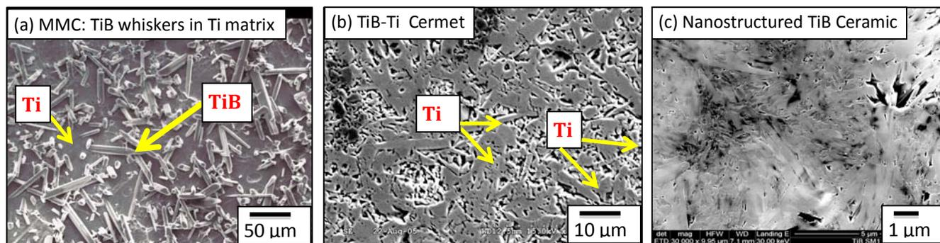
Figure 2. Prior work on binary Ti-B system: (a) Ti MMC containing isolated TiB whiskers ( $\sim 24\%$  TiB)<sup>i</sup>, (b) TiB-Ti cermet ( $\sim 90\%$  TiB) containing alpha-Ti metal phase<sup>ii</sup>, (c) Dense pack of high aspect ratio TiB whiskers forming bulk nanostructured TiB ceramic ( $\sim 98\%$  TiB) by reaction in solid state as documented in our work<sup>iii</sup>.
