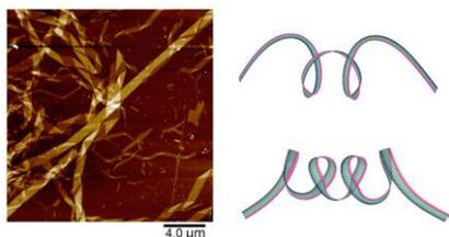
Fig 1. AFM image of dried  $C_{16}K_1$  nanofibers that were initially assembled in aqueous solutions at pH = 5 and with no added NaCl (left). Shapes of nanoribbons from simulation and theory as the salt concentration increases (right).
