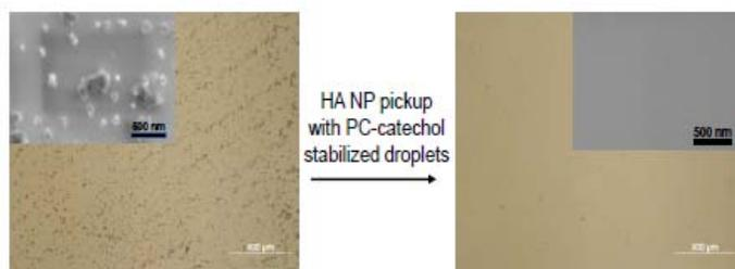
**Figure 4.** Optical microscopy images (scale bar: 500  $\mu\text{m}$ ) of Si substrates before (left) and after (right) HA pickup (SEM image insets are of the same substrates, scale bar: 500 nm).
