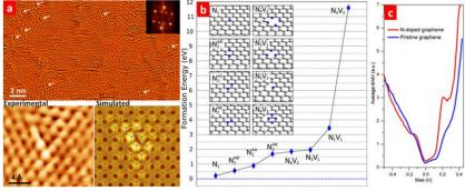
Figure 2. (a), Highly resolved experimental and simulated STM images of  $N2^{AA}$  dopants from as-synthesized NG sheets. (b) Calculated formation energy of different N-doping configurations. (c) Local electronic characteristics of NG sheets based on dI/dV curves measured on  $N2^{AA}$  dopants (red curve) and on pristine graphene (blue curve).
