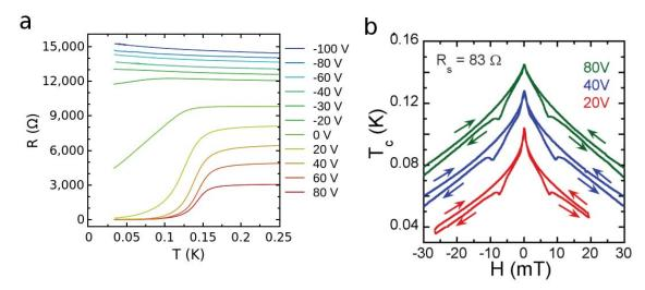
Figure 1: (a), Superconductor to insulator transition (SIT) tuned by a back gate voltage,  $V_g$ . (b) Phase diagrams,  $T_c$  vs. H, at a bias point of  $R_S = 83 \ \Omega$ , at the foot of the resistive transition, at three different gate voltages. Data for  $V_g = 40$  V are shifted by 10 mK and data for  $V_g = 80$  V by 20 mK for clarity (from Publication 1).
