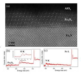
Figure 2. (a) HRSTEM image of a Fe<sub>4</sub>N / Fe<sub>3</sub>O<sub>4</sub> / AlO<sub>x</sub>/Fe stack. (b) EEL spectrum on reaction layer. (c) EEL spectrum on the bottom Fe<sub>4</sub>N layer.
