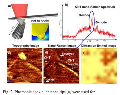
Fig. 2. Plasmonic coaxial antenna tips (a) were used for hyperspectral nano-Raman imaging of carbon nanotubes with 20 nm resolution. A representative nano-Raman spectrum is shown in (b). (c)-(e) show topographic and and spectral images of CNTs using the D-mode vibration peak .intensity.
