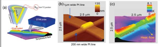
*Figure 2:* (a) Depicts a scanning probe with an integrated thermocouple. (b) The topography of a 200 nm wide metal line that is electrically isolated from a 1 $\mu$ m wide line which acts like a fin. (c) Temperature field of the sample when an electric current passes through the 200 nm line. Adapted from [10].
