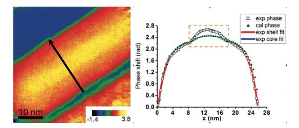
Fig. 1. Reconstructed phase image of SiGe NW with the area used for profile labeled with black arrow with arrow for phase-shift line profile. The result is shown by white squares on the right. The core region is fitted with a polynomial shown in blue and shell region is also fitted with a polynomial shown in red. The green triangles are calculated phase shifts using the projected thicknesses obtained from HAADF intensities. (Li et al., 2011)
