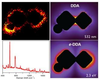
Figure 4: Experimental plasmon map of Ag aggregate responsible for Raman enhancement (top left) and singlemolecule SERS of Rhodamine 6G (bottom left). Near-electricfield enhancement obtained from plane wave excitation at 532nm (2.3 eV) (top right) and EEL probability at 2.3 eV (bottom right).
