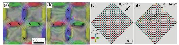
**Fig. 1.** Experimental images of the magnetic induction in an artificial spin ice lattice. (a), (b) ALTEM images showing detail at (a) node obeying spin ice rule and (b) node exhibiting a magnetic monopole defect. (c), (d) MFM images at different values of applied field showing part of the reversal process. Schematics show how color relates to magnetization direction for all four images. The oval in (d) shows the formation of a chain of reversed islands equivalent to a Dirac string.
