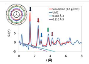
**Figure 4:** Experimental PDF for UMC versus 1.5 g/cm<sup>3</sup> simulated structure. The straight line slope scales with atomic density of scattering atoms: 0.088 Å<sup>-3</sup> (UMC; blue) and 0.11 Å<sup>-3</sup> (graphite, purple). Insert: origin of PDF peaks graphite structure.
