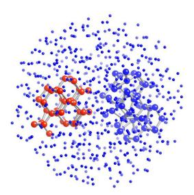
**Figure 1:** Paracrystalline model of amorphous silicon. The red bonded region shows a strained cubic silicon paracrystallite embedded in a matrix of disordered silicon (unbonded blue dots). The paracrystallite is viewed close to the cubic [110] direction. The region of blue bonded atoms is also disordered, and illustrates more clearly the bonding disorder.
