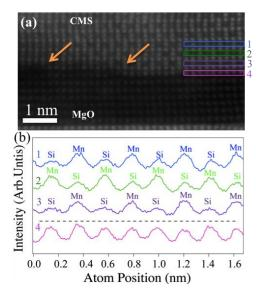
Figure 3. (a) HRSTEM image of the interface of CMS/MgO. CoCo/O and MnMn/O interface terminations are shown in the image on the left and right, respectively. Steps on the top surface of the MgO are indicated by the orange arrows. (b) Horizontal profiles taken on the MnSi planes in CMS electrode and the interface layer. The colors and the labeled numbers of the line profiles correspond to the colors of the horizontal windows in (a).
