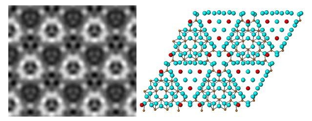
Figure 4: Left, inversion of the raw data from HREM images of the SrTiO<sub>3</sub> (111) 3x3 surface, and right, provisional structure with Ti atoms brown, Sr atoms red and O atoms blue.
