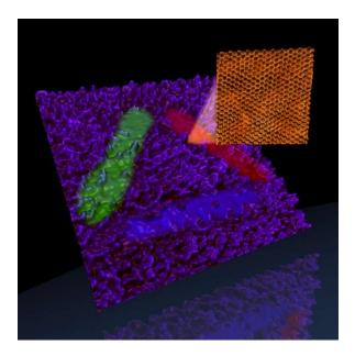
Figure 2: Argonne National Laboratory logo patterned at the atomic-scale (STM image rendered with false coloring added). Hydrogen saturated graphene was controllably patterned via STM induced electron stimulated desorption. The inset shows an atomic-scale image of the patterned graphene, which is structurally preserved and demonstrates the reversible nature of this process.
