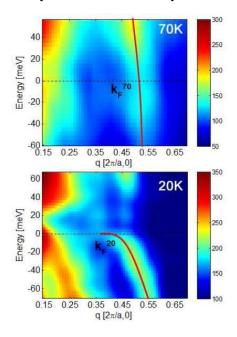
**Figure 2.** Transition from a small to large Fermi surface in CeCoIn<sub>5</sub> showing the development of the heavy fermion state with decreasing temperature detected by spectroscopic mapping with the STM.
