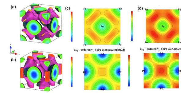
Fig. 2: Electronic charge difference for  $L1_0$ -FePd from QCBED measurements (a) and (c), and DFT (GGA, Wien-2K) calculation in (b) and (d). In (c) and (d) at top and bottom are shown (001) and (002) sections, respectively.
