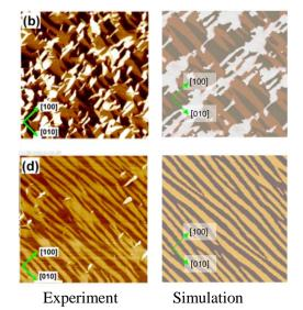
Fig.3. Comparison between experimentally observed 4-variant and 2-variant domain structures of BiFeO<sub>3</sub> films using PFM (left) (Ramesh) and those obtained from phase-field simulations (right).
