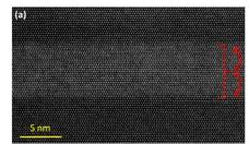
Figure 4: HAADF STEM image of the  $In_{0.15}Ga_{0.85}N$  QW region in an LED. showing no signs of lateral In composition fluctuations. The image was acquired with an electron dose <1% of the reported damaging dose for InGaN at 200 kV.
