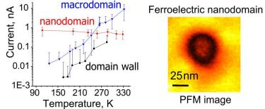
Left: temperature dependence of various conducting entities on the surface of lead zirconate. Nanodomains are metallic in stark contrast to both macrodomains and their domain walls. Right: SPM image of a typical ferroelectric nanodomain.
