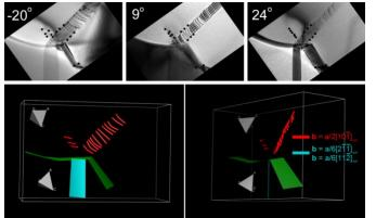
Figure 4. 3D-dislocation model of interaction shown in Figure 3 with example aligned images used in the tomogram reconstruction. Stage tilt is given in each image. The alignment markers are present in the images as black circles.
