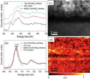
Figure 4. STEM EELS results of the inverse TMR after field cooling. (a) O K edge ELNES extracted from the barrier, top and bottom interfaces. (b) Fe L edge core level shift between upper and lower CoFe/AlOx interfaces (c) simultaneous HAADF image on the area where EEL SI was taken. (d) The intensity map of the pre peak of O K edge.
