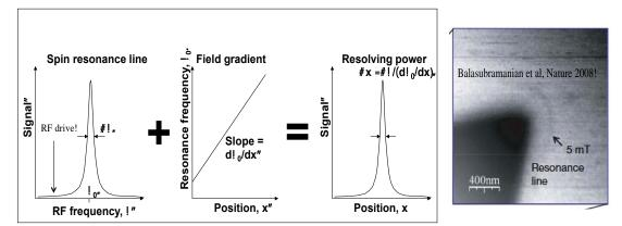
Figure 1: a) Principle of DC magnetic field imaging. The RF drive is kept detuned from the resonance, and whenever the field in the sample matches the difference between the two, we get a signal. (b) Image of resonance slice, obtained using a diamond nanocrystal tip, from a magnetic nanostructure. Taken from Ref. [1].
