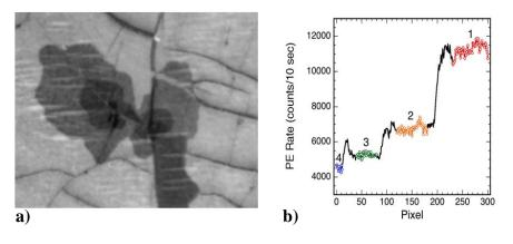
Figure 4: a: PEEM micrograph of multi-layer graphene growth on copper. Areas with 1 to 4 layer coverage are clearly discernible; b: line scan for the photoemission rate (1 pixel corresponds to 10nm.
