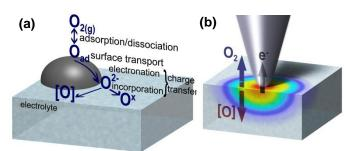
**Figure 1.** (a) Schematic representation of ORR/OER reaction mechanism in pure conductors and mixed-ionic electronic electrodes (b) ESM approach for probing local ORR/OER activity
