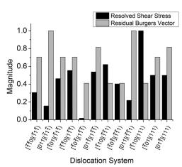
Figure 5. Relative resolved shear stress and normalized magnitude of the Burgers vector of the residual grain boundary dislocation from the interaction shown in Figure 3 on all available slip systems involving partial dislocations in the emitted grain.
