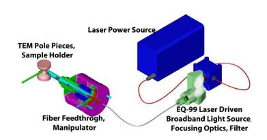
*Figure 1:* Overview of *in situ* illumination showing IR laser, broadband light source and fiber feed through and manipulator.
