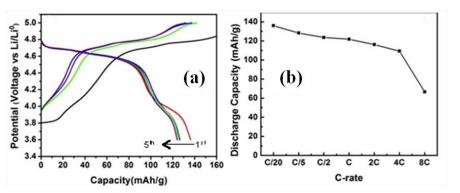
Figure 2: Electrochemical properties of LiNi<sub>0.5</sub>Mn<sub>1.5</sub>O<sub>4</sub> thin film (a) charge-discharge curves for 5 different cycles and (b) discharge capacity as a function of c-rate. [2]
