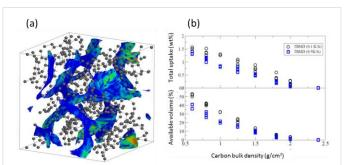
Fig. 5: (a) Simulated carbon structure  $(1.25 \text{ g/cm}^3)$  showing pockets for H<sub>2</sub> adsorption with favorable adsorption energy (< -10 kJ/mol), with blue indicating weaker, and red stronger adsorption sites; (b) Correlation between total H<sub>2</sub>uptake (298 K at 50 bar), available volume, and bulk carbon density. Data show reproducibility between structures obtained in repeated simulations with two quenching rates (black - 0.1 K/fs; blue – 0.5 K/fs).
