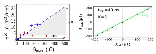
Figure 3: (a) Comparison of sensitivity and dynamic range between our technique (red squares) and standard measurement techniques (blue dots). For more details, see Ref. [2]. (b) Demonstration of the excellent linearity of our technique (blue dots) over a wide dynamic range. The green line is not a fit, but the expected theoretical readout of a perfect sensor.
