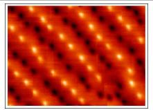
**Figure 1** MFM image of Vortex-Antivortex pairs acquired on a Py/Nb bilayer magnetically coupled at T=5.7 K. The image is in zero applied magnetic field. V-AV pairs are spontaneously generated by the stray field of the Py. The scan area is  $11.4x8.7 \ \mu m^2$ .
