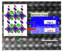
**Fig. 2.** Real-space, atomic-resolution mapping of a spin state superlattice in  $La_{0.5}Sr_{0.5}CoO_{3.\delta}$ . Insets: crystal structure along with the map of the O *K* edge normalized pre-peak intensity, which for this compound correlates with the spin state of Co atoms [Gazquez 2011].
