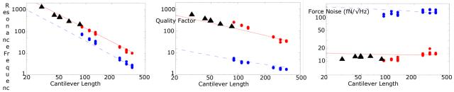
Figure 3 - Resonance frequency, quality factor, and force noise as a function of cantilever length for normal transitievers in air (•) and in water (•). The encased cantilevers ( $\blacktriangle$ ) in water have the same high-performance as normal cantilevers in air.
