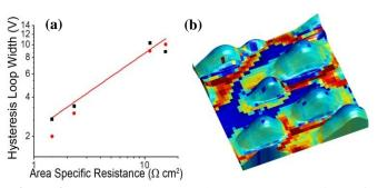
**Figure 2.** ESM on oxygen conductors. (a) Comparison of nanoscale ESM loop width with EIS macroscale measurements of LSCO surfaces (b) Overlay of electrochemical activity on the topography of Pt nanoparticles on YSZ reveals enhanced activity at the triple phase boundary.
