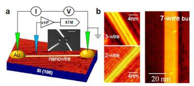
**Fig. 1** (a) A cryogenic four-probe STM is used to probe both the electrical transport and the electronic structures of individual  $GdSi_2$  nanowires (b) STM images of self-assembled nanowires with different width.
