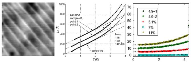
**Figure 1. Superfluid Density in Pnictides.** Using local scanning probes to map the superfluid density can reveal variations associated with doping, scattering, or structure, and help identify uniform samples for fundamental studies. Left: a map of the superfluid density in underdoped Co-doped BaFe2As2 shows strongly enhanced superfluid density on twin boundaries. Middle and right: The temperature dependence of the penetration depth in LaFePO (middle) and Co-Doped BaFe2As2 (right).
