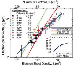
**Fig. 1** Dependence of pulse length on the electron sheet density at time 100 ps for various photoexcitation fluence F and extraction field at the cathode surface  $F_a$ , showing a universal power-law increase with exponent roughly  $\gamma$ ~0.5. Predictions based on mean-field and one-dimensional (1D) fluid models are also presented.
