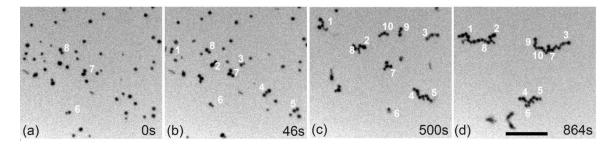
Figure 2 Time sequential images of Au NPs self-assembly in solution. (a) NPs separated on Si<sub>3</sub>N<sub>4</sub> membrane. (b) after exposure by electron beam with intensity of 1.0pA/cm<sup>2</sup> the dimers, trimers formed. (c) and (d) show the short chains formed by existing dimers, trimers and individual NPs attachment. The scale bar is 500nm.
