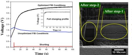
Figure 5: (a) Optimized FIB fabrication condition with preserved electrochemical activity of all-solid-state microbattery (b) two step fabrication process. [5]
