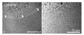
**Figure 2** Bright-field 15-ns pulsed TEM image (a) taken 1400 ns after initiation of a  $4.2-\mu$ J pump laser pulse and (b) a conventional TEM image of the same area taken minutes later. The arrows in (a) indicate the edge of the crystallization front.
