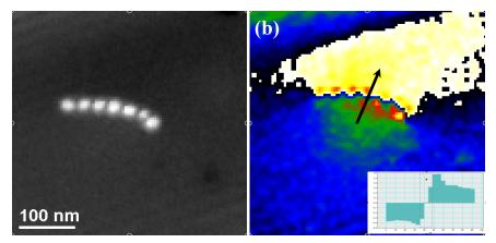
Fig. 3 (a) Holographic phase image of small Fe particles arranged in a chain. (b) Magnetic component of the phase signal obtained by acquiring reversed magnetic orientation holograms and subtracting the phases. Inset shows magnetic flux confined in the particles as steep ramp extending ~13 nm.
