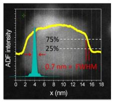
**Fig. 3.** ADF image of a cubic magnetite nanoparticle acquired at the Nion ultraSTEM100 in ORNL using the nanodiffraction mode. The edge of the particle can be used to estimate the full width at half maximum of the electron beam. 0.7 nm approx.
