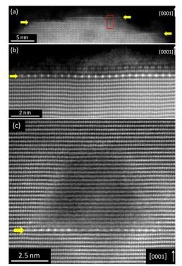
Figure 1: Z-contrast STEM images of Sb-doped ZnO NWs. (a) and (b) are images of NW tips in the  $[11\underline{2}0]$  and  $[10\underline{1}0]$  projections respectively. There are Sb-decorated H-H b-IDBs under the (0001) NW surfaces. (c) shows an internal void with a H-H b-IDB under it bottom surface. H-H b-IDBs in all the images are marked with yellow arrows. The red box in (a) shows where the lattice spacing analysis was done.
