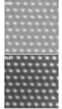
Figure 6: (a) The first of 512 frames of GaN [1120]. (b) The average of 512 frames after non-rigid registration. No other smoothing or image processing has been done. The red dots are the positions of the atomic columns determined by fitting.
