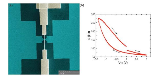
Figure 3: (a) False color scanning electron micrograph of a LAO/STO interface device fabricated by photolithography, electron-beam lithography and dry etching. Light blue-green areas are LAO/STO, dark blue areas are STO, and the gold areas are a metallic top gate. (b) Differential resistance as a function of the top gate voltage of the device of (a), at 77 K.
