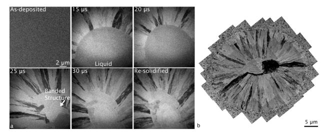
**Figure 3** a) Bright-field 15-ns pulsed TEM images taken before and with different time delays after laser melting. b) Conventional bright-field TEM montage image of an entire laser-melted and re-soldified region.
