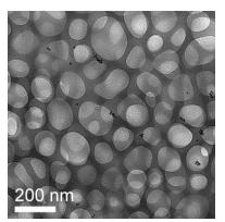
Figure 3. TEM image of a free standing PS-PEO/LiTFSI electrolyte showing a honeycomb morphology. The sample shows a lamellar morphology in the bulk. Unpublished results of Allen and Minor.
