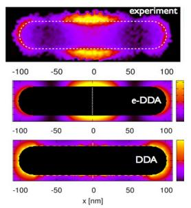
Figure 3: Comparison of the experimentally measured EEL probability map (top) for a loss energy of 2.0 eV. The dimensions of the Ag nanorod are 202x40nm and corresponds to the n=2 mode of the rod. The theoretically calculated EEL probability map for 2.0 eV (middle) is also compared to the electric field enhancement obtained under plane wave excitation at the same energy (bottom).
