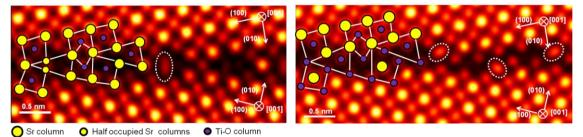
**Figure 1: Average images of the two different atomic structures from a dataset of over 400 cropped experimental images.** Of these cropped images, 35% images show the symmetric structure in a); and 65% images show the rigid-body shift structure in b). The identified structural units are overlaid on the left part of each image. In the average image, atomic columns showing elongated shapes suggest the presence of varying positions along the boundary.
