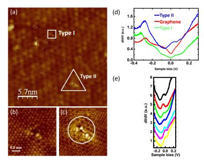
Fig. 2 STM and tunneling spectroscopy of graphene after modification by Ar plasma. (a-c) STM images of type *I* and *II* defects ( $V_s=5$  mV,  $I_t=0.9$  nA). (d) Representative dI/dV spectra taken on graphene, type *I* and *II* structures. (e) Spatially resolved dI/dV spectra taken across the type *II* defect.
