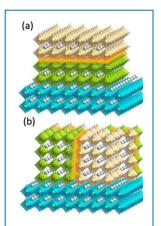
**Fig. 2:** Schematic view of in-plane epitaxial (a) vs. out-of-plane self-assembled nanostructured (b) interfaces of perovskites-type oxide heterostructures.
