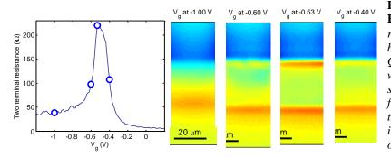
Figure 3. Images of the edge state in a HgTe/HgCdTe Hall bar. Left: resistance of a 30 µm by 60 µm Hall bar. The peak is believed to indicate the Quantum Spin Hall Insulator (QSHI), where the current should flow in edge states. Right: images of the magnetic field from the transport current indicate that current flows uniformly through the interior away from the peak, but flows on the edges in the QSHI state.
