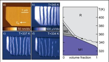
**Fig. 13.** Topography (a) and *s*-SNOM (b-d) of VO<sub>2</sub> MIT with gradual growth of insulating (dark) domains, with remaining metallic phase islands persisting well below the nominal  $T_{MIT}$ . Right: Corresponding volume fraction of M1, M2, and R phases for micro-crystals derived from the combination of *s*-SNOM and micro Raman spectroscopic imaging.
