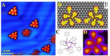
Fig. 3. (a). Topographic STM images of "magic" clusters of phenylacetylene on Au(111). (b) The fully relaxed hexamer.(c) Natural Bond Orbital analysis of the CH/ $\pi$  bonding motif.(d) Simulated STM image for fully relaxed hexamer.
