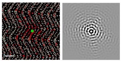
Left: reacted  $CH_3SSCH_3$  molecules (red) surrounding a pulse of hot-electrons injected into the surface from an atomically-sized STM tip (green square). Right: probability density of hotelectrons around a point of origin (center) on the gold surface with finite density of elastic scatterers and an inelastic mean-free path of ~ 5nm. This observable is effectively probed in delocalized reaction experiments.
