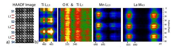
**Figure 1**. STEM ADF image of 2x2 LaMnO3-SrTiO3 oxide artificial superlattice, with corresponding ELNES inner-shell spectra. The vertical axis of the spectra is aligned with corresponding position in the STEM image, and the horizonal axis is energy loss at an absorption edge. Color shows intensity of inelastic scattering.
