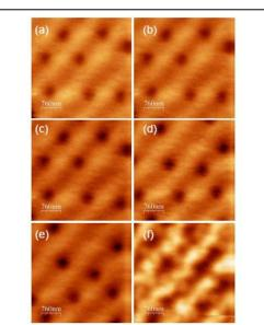
Figure 2 MFM images of a Py/Nb bilayer at T=5.5 K. The applied magnetic field perpendicular to the surface is swept from (a)H= -16 Oe, to (b)=+14 Oe, (c) H=+34 Oe, (d) H=+37 Oe, (e) H=+47 Oe, (f) H=+95 Oe. The scan area is 3800 nm x 3800 nm.
