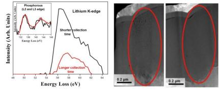
Figure 6: (a) EELS spectrum showing the effect of longer collection time and (b) showing the e-beam damage due to longer collection time (left) and shorter collection time (right). [5]
