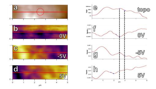
Figure 3: Line profiles of topographic and SSPM images (red lines) collected under various bias conditions at 400°C applied thermal load. The vertical black dotted lines represent the individual grain topographic feature (red dotted circle). The surface potential line traces indicate local linear resistances are observed across individual grains, trending with their bias conditions.
