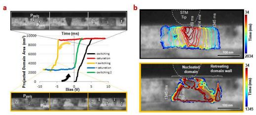
**Fig. 2. Interface assisted switching** – **a**, Chronological TEM image series of local polarization reversal in  $PbZr_{0.2}Ti_{0.8}O_3$  as it traverses the hysteresis loop shown at center. The loop was derived from the total switching domain area. **b**, The same two switching events showing the domain extent versus time.
