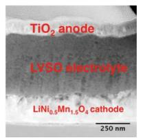
Figure 4: Cross-sectional SEM image of the all-solidstate battery prepared by PLD and subsequent FIB TEM/EELS investigation. Moreover, there were no crack or pin holes even after the anode  $TiO_2$  deposition. In spite of the FIB processing and the STEM observations, the solid electrolyte remains amorphous as examined by diffraction in TEM. The interfaces between the layers are found to be sharp and well defined.
