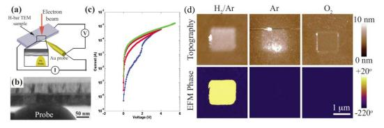
**Fig 2.** (a) Schematic showing in-situ TEM transport measurement set-up, (b) cross-section image of a Pt/HfO<sub>x</sub>/Pt heterostructure, and (c) electroforming curves recorded from the same region. (d) Topography (upper row) and EFM phase images (lower row) after tip-induced stress analysis of a 1.5  $\mu$ m×1.5  $\mu$ m square region of TiO<sub>2</sub> in H<sub>2</sub>/Ar, Ar, and O<sub>2</sub> environments.
