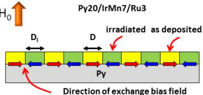
**Direction of exchange bias field** Figure 1: Schematic of a permalloy (Py) exchange biased sample fabricated by coating a 20 nm thick continuous Py film with a 7 nm IrMn layer capped by a 3 nm Ru layer (not shown) to avoid oxidation. A striped pattern of exchange bias field is generated by depositing the IrMn layer while exposed to an external, in-plane magnetic field followed by selective irradiation of IrMn layer with He ions in a reversed, in-plane magnetic field.
