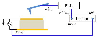
Fig. 2. Schematic of SMEM setup showing the basic principle of SMEM operation. The local moments of ME domains induced by modulated electric field produce modulated stray fields which are sensed by MFM (resonant frequency shift) and demodulated by a PLL followed by a lockin amplifier.
