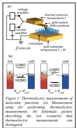
temperature of the tip is directly dependent on the temperature of the surface thus enabling measurement of local temperature with nanoscale resolution.
