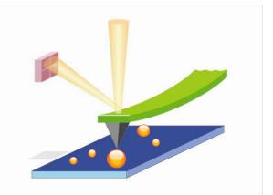
Figure 1. Schematic representation of electrical analysis of nano sized interface with SPM.
