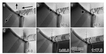
Figure 3. Frames taken from a video showing dislocations interacting with a high angle grain boundary during straining at 400°C. Video times are given in each image. Frames b and c indicate that, upon absorbing a dislocation (indicated by arrow head), a lead Shockley partial dislocation is emitted from the boundary within  $1/10^{\text{th}}$  of a second.
