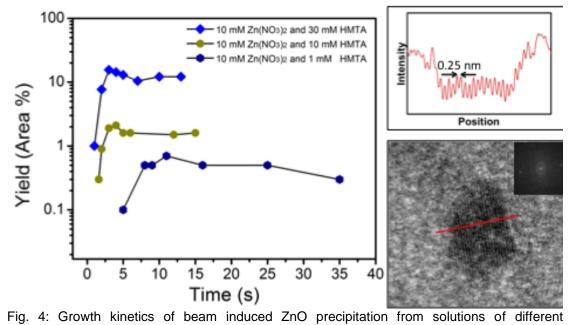
Fig. 4: Growth kinetics of beam induced 2nO precipitation from solutions of different composition and an associated HRTEM image take during in-situ nucleation and growth. Note that no growth was observed for 10 mM  $Zn(NO_3)_2$  solutions containing no HMTA.
