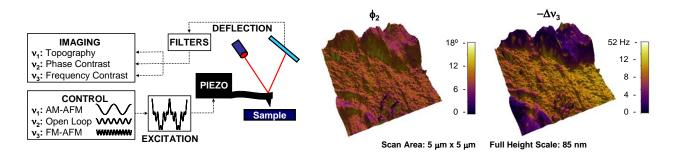
**Figure 1.** Schematic of previously implemented triple-frequency intermittent-contact AFM controls scheme (left); typical images of the second eigenmode phase ( $\phi_2$ , center) and negative of the third eigenmode frequency shift ( $-\Delta v_3$ , right) superimposed on the topography acquired with the first eigenmode for a tri-block co-polymer calibration standard. [S. D. Solares and G. Chawla, J. Appl. Phys., 108, 054901 (2010)]
