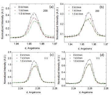
**Figure 3**: Change in 200 diffraction peak profile for randomly oriented polycrystalline sample, (a) parallel, and (b) transverse, to the direction of applied electric field. Figures (c) and (d) show change in 111 diffraction peak profile for the same sample, parallel, and transverse to the applied electric field direction, respectively.
