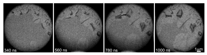
**Figure 1** Bright-field 15-ns pulsed TEM images of laser-induced crystallization of amorphous GeTe. The time indicates the delay between the laser pulse that initiated crystallization and the electron imaging pulse.
