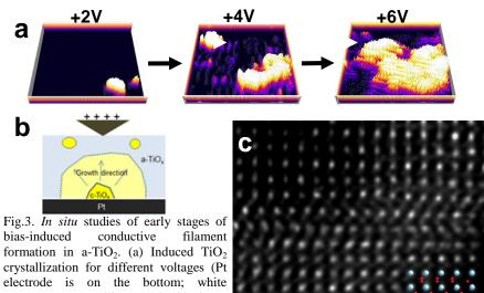
crystallization for different voltages (Pt electrode is on the bottom; white represents crystalline and black – amorphous material), (b) schematic of the filament nucleation, (c) Stacking faults in  $TiO_2$  close to Pt electrode indicating reduction.
