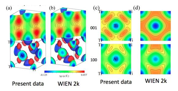
Fig. 1: Comparison of electronic charge difference maps for  $L1_0$ -TiAl obtained by QCBED experiment (a), (c) and DFT (GGA, Wien-2K) calculation in (b), (d). Note the bonding charge accumulation in the tetrahedral interstices (a), (b) and overestimated electron delocalization between Ti-Ti second nearest neighbors along [010], (c) vs. (d).
