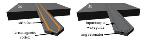
Figure 1. (a) Active magnetic probe. (b) Active optical probe.
