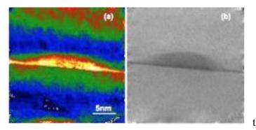
Fig. 2. (a) Phase and (b) amplitude images calculated from the reconstructed hologram of wurzite GaN QD, with base diameter of 23 nm and a height of 3.75nm.
