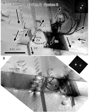
associated diffraction pattern of dislocations interacting with twin boundaries. Arrows show direction of dislocation motion.
