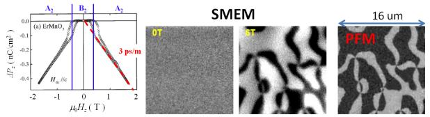
**Fig. 3.**  $\Delta P_z(H)$  at 4.2K of ErMnO<sub>3</sub> with *H* // c-axis by Sugie et al. (ref. 7) Preliminary SMEM data of ErMnO<sub>3</sub> at 0 T and 6 T. RT-PFM image of the same area.  $V_{mod}$ =200 V<sub>rms</sub>,  $f_{mod}$ =50 Hz.
