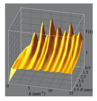
**Figure 2:** Three dimensional plot showing the calculated normalized variance, *V*(*k*), as a function of scattering vector *k* and microscope resolution, *R*. The mean paracrystalline grain size is 1.2 nm, and the variance is a maximum near  $R \approx 0.8$  nm, which is the value of  $\lfloor$  for this model. For  $R > \lfloor$  the variance decays approximately as
