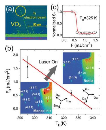
*III.* Decoupling of structural and electronic phase transition in VO<sub>2</sub>.
