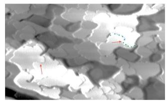
Figure 2. A (600nm x 360nm) AFM image of a 50nm thick insulating ice film on Pt(111) grown at 140K showing the arrangement of molecular-height steps. The red arrows point to threading screw dislocations with a burgers vector equal to the height of two steps (separately marked by the green and blue dots, respectively), establishing that the film is composed of hexagonal ice Ih. In contrast, thinner films are predominately cubic ice Ic.
