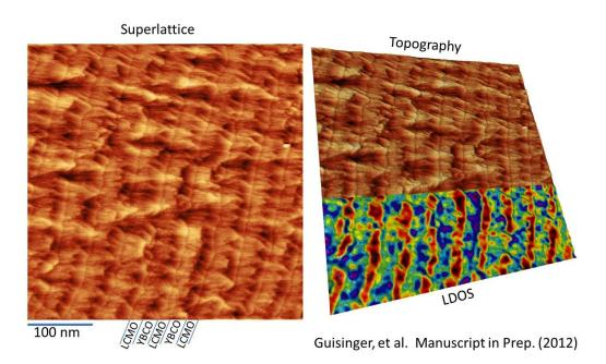
Figure 1: Cross-sectional STM utilized to study the interfaces of an oxide superlattice that includes simultaneous topographic and electronic band mapping.
