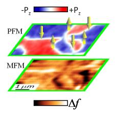
Fig. 1 | Preliminary results. RT-PFM image and MFM image (5.5 K, 0.2 T) taken at the same location on the (001) surface of multiferroic hexagonal ErMnO<sub>3</sub>. The arrows in PFM image represent the net magnetic moments in ferroelectric domain walls.  $\Delta f = 0.8$  Hz.
