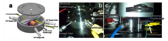
Figure 2: (a) schematic of the miniature environmental chamber design; (b) digital photograph of the actual miniature chamber as fabricated; (c) digital photograph of miniature chamber integrated with a commercial AFM scan head, while operating.
