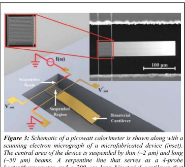
(~50  $\mu$ m) beams. A serpentine line that serves as a 4-probe heater/thermometer and a 200  $\mu$ m long bimaterial cantilever that acts as an ultra-sensitive thermometer are integrated into the suspended region. Adapted from [7]
