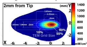
*Figure 3*: The light distribution as a function of position on the TEM sample when the end of the optical fiber is located 2 mm from the TEM
