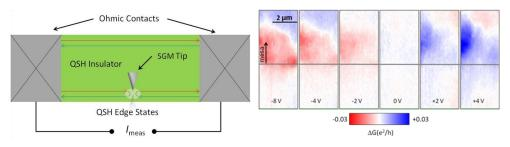
Fig. 2 (Left) Schematic of the SGM setup for study of the 2D topological insulator (not to scale). (Right) In the vicinity of the mesa edge (grey solid line), a clear tip effect on the conductance can be observed.
