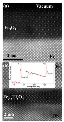
Figure 1 (a) HRSTEM image of a  $Fe_3O_4$  film oxidized at 400 C (b) a second phase layer  $Fe_3$ . <sub>x</sub>Ti<sub>x</sub>O<sub>4</sub> at the TiN/Fe interface. The inset of 2(b) is an EEL spectrum from the second phase.
