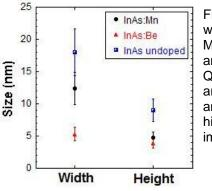
Fig. 1: Comparison of widths and heights of Mn-doped, Be-doped, and undoped InAs QDs. These values are based upon an analysis of several high resolution images of the QDs.
