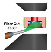
Figure 2: Schematic diagram of end of fiber in the ETEM adjacent to TEM sample located in hot stage furnace between upper and lower pole pieces of objective lens. The 30° cut refracts light towards the TEM sample.
