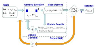
Figure 2: Flowchart for phase estimation algorithm (PEA).
