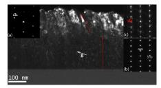
Figure 3. Dark-field image with the [111] **g** vector of the ZB structure. SAD patterns of (a) the ZB top layer, (b) the WZ bottom layer, and (c) a region with both WZ and ZB. Additional spots in (c) are caused by double diffraction and twinning in the ZB phase. The angle between the grain boundaries in the WZ and ZB corresponds to angle between  $[0001]_{WZ}$  and  $[220]_{ZB}$ .
