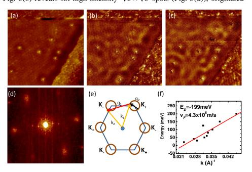
Fig. 3 **dI/dV imaging of defect scattering in graphene.** (a) STM ( $V_s$ =-50 mV,  $I_t$ =1.0 nA, 45x45 nm<sup>2</sup>) and (b) & (c) simultaneously acquired dI/dV images at  $E_F$ -50 and  $E_F$ -20 meV, respectively, using lock-in technique. (d) FT pattern of image (b). (e) Diagram showing inter- and intra-valley scattering. (f) Dispersion obtained by measuring  $q_2$  as a function of energy.
