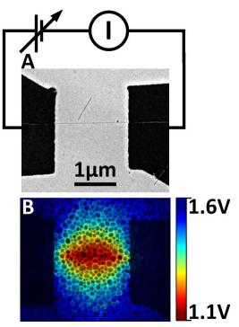
Figure 2. Thermal dissipation about a current-carrying nanotube. (A) measurement schematic and TEM image of the nanotube and contacts, prior to indium deposition. (B) (original in color) Thermal map of the platform where color indicates the melting voltage of each indium island, overlaid with a black and white image of the indium islands.
