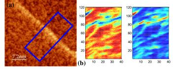
**Figure 3.** (a) Atomically-resolved STM image and (b) principal component analysis of the I-V spectroscopic image acquired in the box in (a). Electronic inhomogeneity at the defect is clearly seen.
