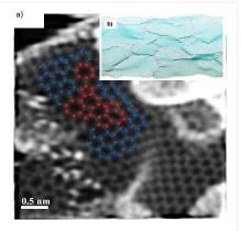
**Fig. 6:** Atomic resolution STEM image typical for graphenes in nanoporous carbons, showing defective rings of 5-7 atoms (a) and 3D relaxed graphene sheet with ripples and folds introduced by topological defects (b).
