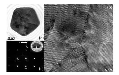
Figure 1 (a) bright field TEM image of 90°-cross sectional Ag NW. (b) HREM image of core area of (a) (by ACAT). (c) electron diffraction pattern of 45°-cross section of Ag NW with electron beam parallel with [010]. The inset is a shadow image. [5]
