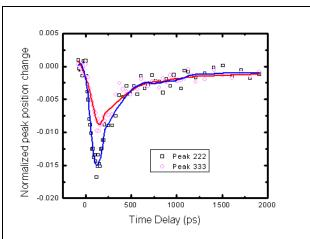
Fig.1 Ultrafast electron diffraction measurements of (222) and (333) peak positions of Ag nanocrystals supported on TiO<sub>2</sub> under 200 mW, 120 fs pulsed laser illumination. The peak position is normalized by length of g.
