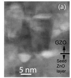
Figure 2. High resolution annular brightfield STEM image of the interface between the undoped ZnO seed layer and GZO grown under metal-rich conditions showing IDBs terminated by pores.
