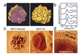
**Figure 3** Revealing the correlation of valence state with nanoporous structure in cobalt catalysts by in situ environmental TEM. (a) 3-D tomographic reconstruction of an as-prepared  $CoO_x/SiO2$  nanoparticle. (b) Co  $L_{2,3}$  edges of the catalysts from in situ EELS measurements. (c) In situ TEM of structural changes of the catalysts at different reduction conditions. (d) An only 3.5 nm silica shell can prevent the particle from oxidation at room temperature.
