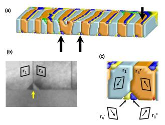
Figure 1. (a) Cross-section of a BiFeO<sub>3</sub> film with vertical 109° domains along the  $[100]_p$  direction. (b) Cross section dark field TEM image of a 20nm BiFeO<sub>3</sub> film on insulating TbScO<sub>3</sub> substrate. (c) Enlarged cross-section of (a) showing an example of triangular domains at the film/substrate interface from simulation.
