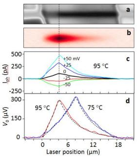
Figure 1. SPCM applied to a suspended VO<sub>2</sub> nanobeam. (a) Reflection image of a device at 95 °C: the darker region is metallic (M), the paler insulating (I). (b) Photocurrent image at bias V=0, showing a peak at the M-I interface. (c) Line traces of photocurrent lph along nanobeam center for series of V. (d) Line traces of determined photo-emf V0 = RIph at two temperatures. Dashed lines are the predicted photothermal voltage.
