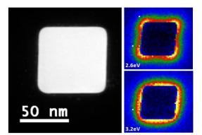
Figure 2: ADF image and STEM/EELS derived plasmon maps for a Ag nanocube. The 2.6 eV mode appears in the optical spectrum; however the mode at 3.2 eV is optically dark.
