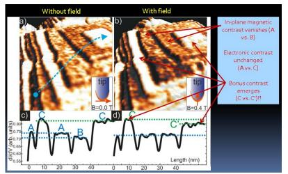
Fig. 1. SP-STM images of MnN spin pyramids with a) field OFF case; and b) field ON case. Line sections below in C) and D) illustrate the contrast between A and B layers without field and C and C' layers with field. [*Nano Letters (http://dx.doi.org/10.1021/nl204192n), (2012).*]
