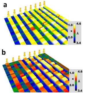
Fig. 1.Maps of oxygen distribution in vacancy ordered  $La_{0.5}Sr_{0.5}CoO_{3-\delta}$  films grown on different substrates given as oxygen content *x* in  $CoO_x$  layer: (a) film grown on NdGaO<sub>3</sub> is highly ordered brownmillerite  $La_{0.5}Sr_{0.5}CoO_{2.5}$  while (b) film on (La, Sr)(Al,Ta)O<sub>3</sub> has overall composition of  $La_{0.5}Sr_{0.5}CoO_{2.75}$  with a significant degree of disorder (from [2]).
