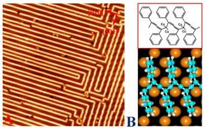
Fig. 4. (a) Highly ordered self-assembled linear polymer on Cu(100). (b) Chemical structure and ball-and-stick model of linear polymer from relaxed DFT calculations (lime is carbon, orange is copper substrate and cyan is hydrogen atoms).
