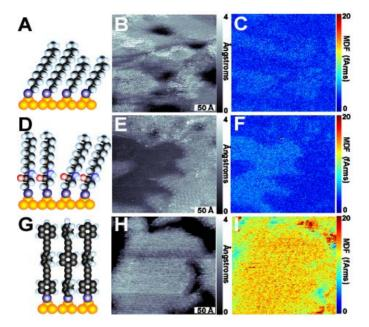
Figure 2. Simultaneous topographic and microwave polarizability mapping enables location of multiple bonds, heteroatoms, molecule-substrate contacts, and molecule-molecule contacts. This method is being used for chemical differentiation and for structural determinations.
