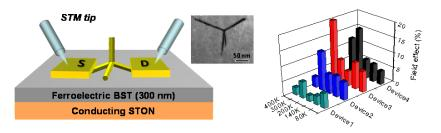
Figure 4. A cryogenic four-probe scanning tunneling microscopy (STM) is used to probe the electrical transport through individual CdS nanotetrapods with a ferroelectric  $Ba_{0.7}Sr_{0.3}TiO_3$ (BST) film as gate dielectric. A ferroelectric field effect transistor (FeFET) operation is demonstrated.
