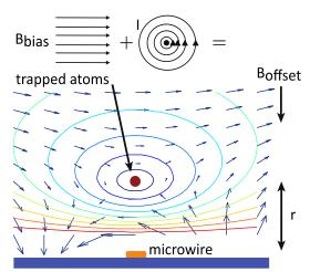
Figure 1: (a) Atom chip trapping principle. A cylindrically symmetric quadrupole magnetic field is created by superimposing a weak, homogeneous bias field B<sub>Bias</sub> with that from a microwire with current I. Weak-field seeking atoms---i.e., atoms in a Zeeman state whose energy increases for increasing magnetic field magnitude---are trapped in a small region around the zero of the magnetic quadrupole field.
