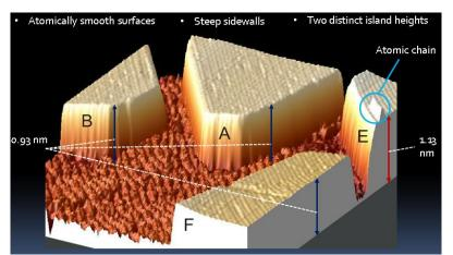
Fig. 3. 3-D rendered STM image of quantum height MnGa islands formed on GaN(000<u>1</u>) surface. Image size is 80 nm x 87 nm, Vs = -0.87 V, It = 156 pA. Islands labeled B, A, F have the same height; the island labeled E has a different height which is higher by one atomic layer than B, A, F. [Applied Physics Letters 100, 061602 (2012)]
