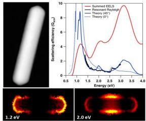
Figure 1: (Top) Annular dark field (ADF) image of a Ag nanorod with STEM/EELS spatial maps. (Bottom) Experimental and classical electrodynamics resonance-Rayleigh scattering spectra
