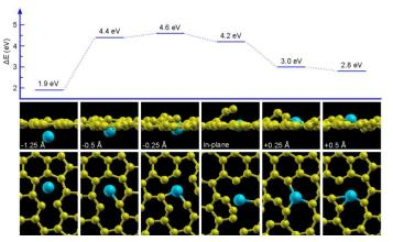
Fig. 1 **Calculated energies and Si diffusion process.** Snapshots of vertical migration process of Si through the warped interfacial layer in cross section (middle panel) and plane (bottom panel) view.
