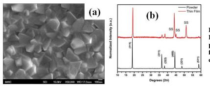
Figure 1: (a) SEM image of the  $LiNi_{0.5}Mn_{1.5}O_4/SS$  and (b) XRD patterns of  $LiNi_{0.5}Mn_{1.5}O_4$  thin film and powder for comparison. [1,2]
