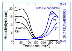
**Fig. 4:** Transport properties of 20nm ultrathin film of  $La_{0,7}Ca_{0,3}MnO_3$  shows insulating behavior. After application of Fe nanodots resistivity data of the same film shows a recovery to bulk-like behavior with a MIT temperature of 255 K at 0 T.
