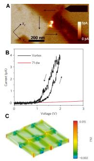
Fig. 1. Enhanced conductivity at vortex cores. (A) The in-plane PFM image of a fabricated vortex structure, with c-AFM overlay showing conductivity at the core. (B)The I-V curve at the vortex core, in comparison with 71° domain walls. (C) Trace of strain tensor of the vortex/anti-vortex lattice
