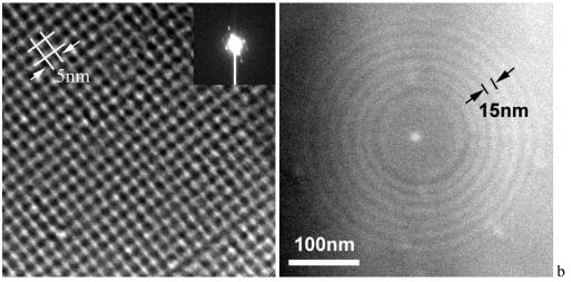
**Figure 2.** These patterns of elemental silicon in silicate glasses were written with a 0.2nm STEM probe, giving lines with 5nm period.
