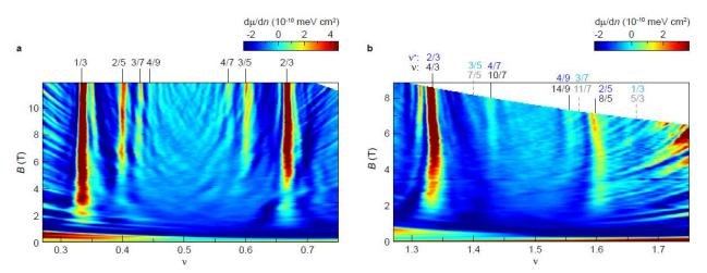
Figure 2.a, Inverse compressibility as a function of filling factor v and magnetic field B. Incompressible states follow the standard composite fermion sequence between v = 0 and 1. b, Finer measurement of inverse compressibility between v = 1 and 2. Incompressible states occur only at filling fractions with even numerators. The incompressible behavior adheres to the sequence  $v^* = 2 - v = 2p/(4p \pm 1)$  for  $p \le 2$ .
