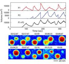
**Figure 1** Oscillatory growth of Bi nanoparticles. Trajectories of two particles showing pairwise oscillation.
