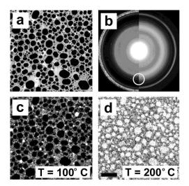
Figure 1. Demonstration of the principle of electron thermal microscopy. a) bright-field image of indium islands. b) a composite diffraction part of solid (left) and molten (right) islands. With the objective aperture at the circle, images c) and d) are produced in the solid and molten phases, respectively.
