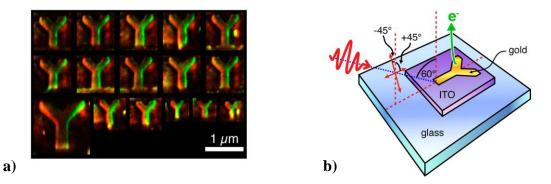
Figure 3a: Composite PEEM micrograph showing plasmon distributions in gold nanostructures when excited with visible light of different polarizations: green color relates to  $+45^{\circ}$  polarization, red color to  $-45^{\circ}$  polarization as defined in the excitation scheme in part b) of the figure.
