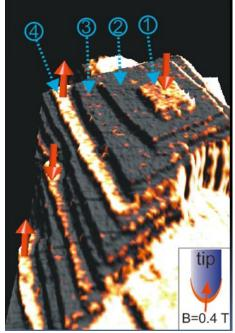
Fig. 2. SP-STM image of MnN Nanopyramid in 3-D rendering, with contrast level suppressed, in which you can see the contrast on the C/C' layers when out-of-plane field is ON. [*Nano Letters*]
