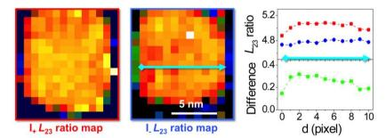
**Fig. 4.** Color coded  $L_{2,3}$  ratio maps obtained from a spectrum image of the nanoparticle shown in **Fig. 3** acquired at I<sub>+</sub> and at I<sub>-</sub>, respectively, along with the  $L_{2,3}$  profile along the direction of the blue arrow. The right panel shows the difference between the I<sub>+</sub> and I.  $L_{23}$  ratios, which should be proportional to the local magnetic moment.
