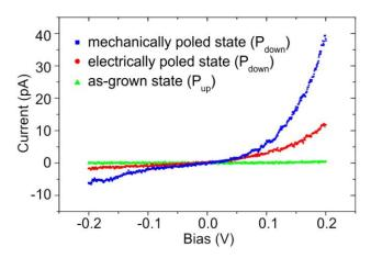
**Figure 2**. Comparative analysis of the mechanically and electrically induced TER effects. Local I-V curves measured for the as-grown film area with upward polarization (green), electrically downward-switched domain (red) and mechanically downward-switched domain (blue).
