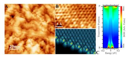
Fig. 1. (a) A typical GNR placed on a  $Si/SiO_2$  substrate observed in STM measurements (b) Atomic resolution image of an edge region with simulated STM images based on a reconstructed edge structure.(c) Color mapping for the calculated local density of states shows two spin-split peaks around the Fermi energy taken perpendicularly to the axis of a graphene ribbon.
