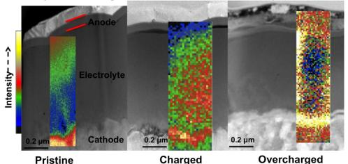
Figure 7: Li intensity mappings for pristine, charged, and overcharged samples. [6]
