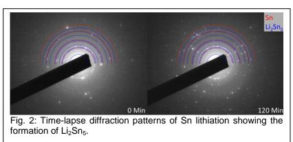
$1M \text{ LiPF}_6$  electrolyte in an enclosed environmental cell. Sn anodes display large volumetric strain during lithiation and delithiation. How the microstructure
