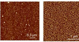
Fig. 5: AFM image of high density (3x10<sup>10</sup> cm<sup>-2</sup>) InAs QDs grown by droplet epitaxy on GaAs.
