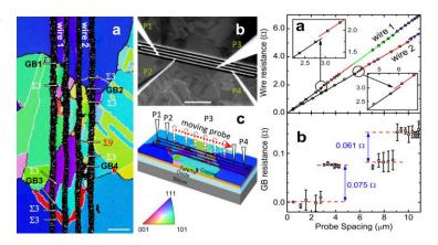
**Figure 2**. Left Figure: Structures of copper nanowires. (a), The inverse pole figure of EBSD map showing the orientations of grains and GBs. (b), SEM image showing four-probe STM contacted onto the same copper nanowire. (c), A schematic illustrating the resistance measurement procedure with 4-probe STM. Right Figure: resistance jumps near random GBs.
