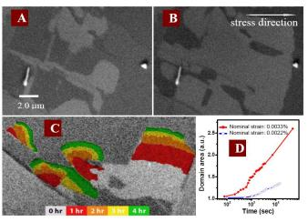
**Figure 3.** Strain-induced domain evolutions in the cleaved surface of a  $Sr_3(Ru_{0.8}Mn_{0.2})_2O_7$ . (A), Domain image before stress and (B), after applying an uniaxial compressive stress in the *ab* plane. (C), Domain evolution in time with nominal strain of 0.0022%. (D), Domain area change with time.
