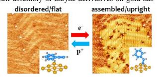
Transformation of a disordered mobile layer of physisorbed phenylacetylene molecules on the gold surface into a self-assembled arrangement of strongly bonded upright conjugated molecules by injection of hot electrons. Hot holes reverses the process.
