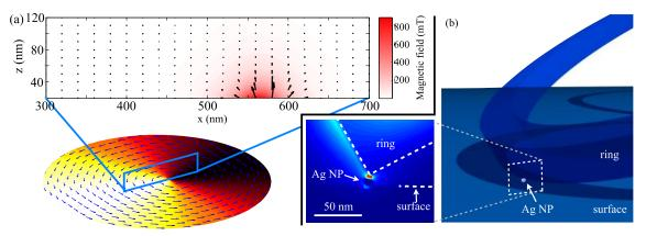
Figure 2. (a) Bottom: Micromagnetic simulation of magnetization of a 2  $\mu$ m diameter Permalloy disk. Top: Magnetic field in a region above the disk. (b) Right: Schematic of a ring resonator above a nanoparticle. Cantilever is not shown. Left: Finite-difference time domain simulation of electric field amplitude in and around the ring, in proximity to a nanoparticle.
