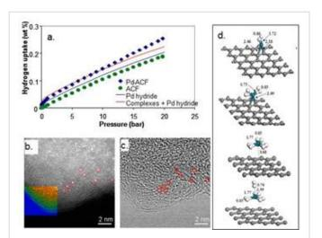
**Fig. 1** (a) Experimental  $H_2$  adsorption on ACF and Pd-ACF compared with behavior expected if all Pd is converted to Pd hydride and based on Kubas mechanism hypothesis. Also shown are (b) single Pd atoms and (c) carbon structures identified by HR-STEM; and (d) predicted Kubas structures for multiple bonding of  $H_2$  to single Pd atoms. [1,2]
