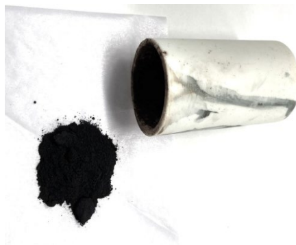
Figure 3. Regenerated lithium nickel manganese cobalt oxide (LiNi a Mn b Co c O d ) after pyrolysis of chelate in an alumina crucible at 800 °C.
