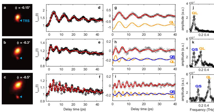
Figure 3. Truncation rod scattering (TRS) from (112) cut TaAs for incident angles of  $\Delta\phi =$  (a)  $-0.15^\circ$ , (b)  $-0.3^\circ$ , and (c)  $-0.5^\circ$  degrees. The resulting transients shown in (d-f) and (g-i) show the extracted QL and QS oscillations in the time domain, followed by frequency domain spectra in (j-l).
