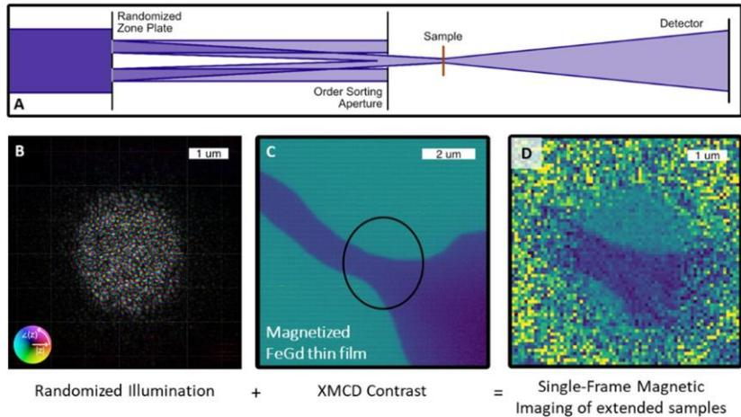
Figure 10. Randomized Probe Imaging. (A) Experimental setup. (B) Randomized illumination function. (C) Ptychographic reconstruction of magnetic domains in a FeGd film. (D) Single-frame reconstruction from the same sample (black circle in C).
