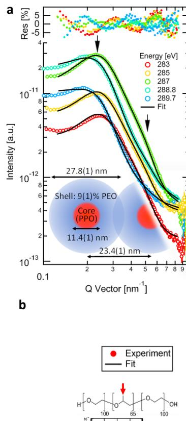
Figure 1: **RSoXS spectral analysis can extract quantitative molecular composition inside nanostructures.** (a) Simultaneous multi-resonance fit to extract both structural statistics and molecular composition (inset) of a Pluronic F127 organic nanocarrier used in drug-delivery. (b) F127 dynamics captured in a dual-flow experiment fit to a double exponential model. Inset is the F127 molecular structure, highlighting the single identifying chemical moiety.
