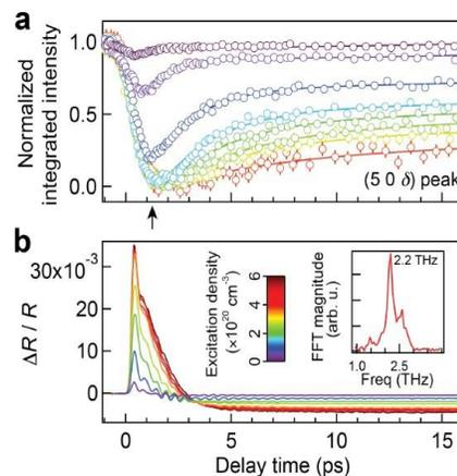
**Figure 1** **a**, Time evolution of the superlattice peak integrated intensity in  $\text{LaTe}_3$  upon photoexcitation at different excitation densities. **b**, Transient reflectivity as a function of delay time at different excitation densities. The color scale is the same in both panels. Inset: Fourier transform of the oscillatory component.
