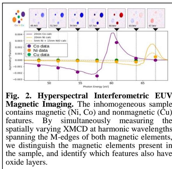
**Fig. 2. Hyperspectral Interferometric EUV Magnetic Imaging.** The inhomogeneous sample contains magnetic (Ni, Co) and nonmagnetic (Cu) features. By simultaneously measuring the spatially varying XMCD at harmonic wavelengths spanning the M-edges of both magnetic elements, we distinguish the magnetic elements present in the sample, and identify which features also have oxide layers.
