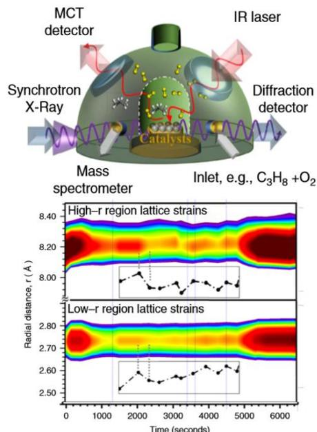
**Fig. 1** (first row) Set-up for combined *in situ* PDF and DRIFTS studies. (second row). Oscillatory behavior of bonding (2.75 Å) and higher-r distances in nanocatalysts during oxidation of propane [1].
