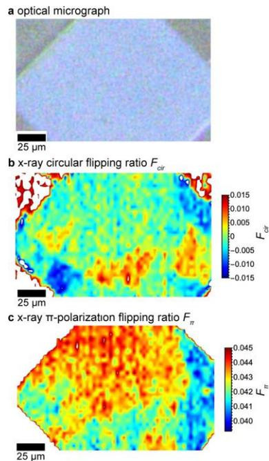
**Fig. 2: Domain imaging in GdIG SSE devices.** (a) Ppatterned GdIG layer from which GdIG has been removed in the area outside the light square. X-ray nanobeam diffraction maps of (b) circular-polarization flipping ratio  $F_{cir}$  and (c) linear  $\pi$ -polarization flipping ratio  $F_{\pi}$ . [1]
