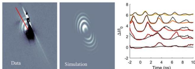
Figure 7. Diffuse x-ray scattering image (experiment and simulation) from STO following x-ray pumping, and time-dependent responses at selected phonon wavevectors. Shown are the difference between unpumped and pumped images, but the signals were so strong that the modulations were visible in the raw images. Representative traces on the right are in absolute units, offset for clarity.
