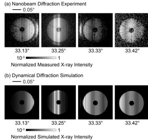
**Fig. 3: Nanobeam dynamical diffraction experiment and simulation.** (a) Observed and (b) simulated focused-beam dynamical diffraction patterns for a GaAs-AlGaAs heterostructure, at different values of the x-ray incident angle.
