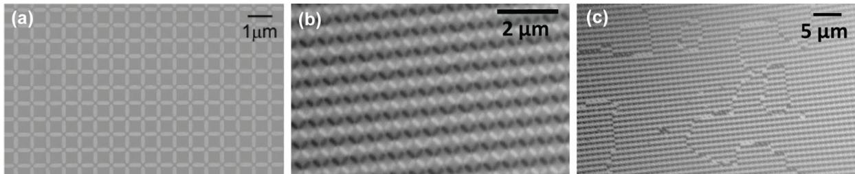
Figure 1. (a) Scanning electron micrograph of a square artificial spin ice fabricated from  $\approx 3$ -nm thick permalloy. (b) Anti-ferromagnetic ground state imaged by x-ray magnetic circular dichroism photoemission electron microscopy (XMCD-PEEM). (c) Superdomains of the AF ground state separated by superdomain walls.
