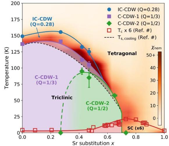
**Figure 2** Phase diagram of  $\text{Ba}_{1-x}\text{Sr}_x\text{Ni}_2\text{As}_2$  showing three different charge density waves, denoted IC-CDW, C-CDW-1, and C-CDW-2, superconductivity, and fluctuating nematic order (color scale), all in the same material system.
