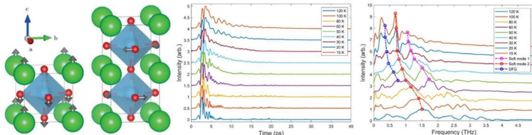
Figure 1. (a) Soft mode (left, shown in the high- $T$  cubic phase for simplicity) and antiferrodistortive (AFD) mode along which a cell-doubling transition into the low- $T$  tetragonal phase occurs at 105 K. (b) THz-induced lattice responses probed through optical second harmonic generation. (c) FT of data in (b) showing the two inequivalent soft modes and a difference-frequency feature which may be due to nonlinearly coupled AFD mode displacements.
