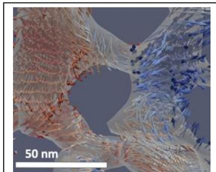
**Fig. 3. First general vector ptychotomography method to image spin textures in 3D.** 3D spin texture in spin-engineered, topologically distinct, magnetic metalattices. The spatial resolution is ~10 nm.
