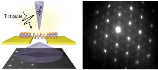
Figure 4. (a) Schematic illustration showing THz irradiation of a single-layer MoTe<sub>2</sub> sample that spans a 1-micron insulating gap between parallel gold lines of a THz field enhancement structure. Transmissive electron diffraction is then conducted on the sample. (b) Diffraction pattern from a multilayer sample reveals additional (dimmer) spots induced by a single THz shot, indicating the cell-doubling transition from the initial 2H phase to the 1T' topological insulator phase.
