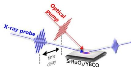
Figure 6. Schematic illustration of optical-pump, XRD-probe experiments on SRO/YBCO.
