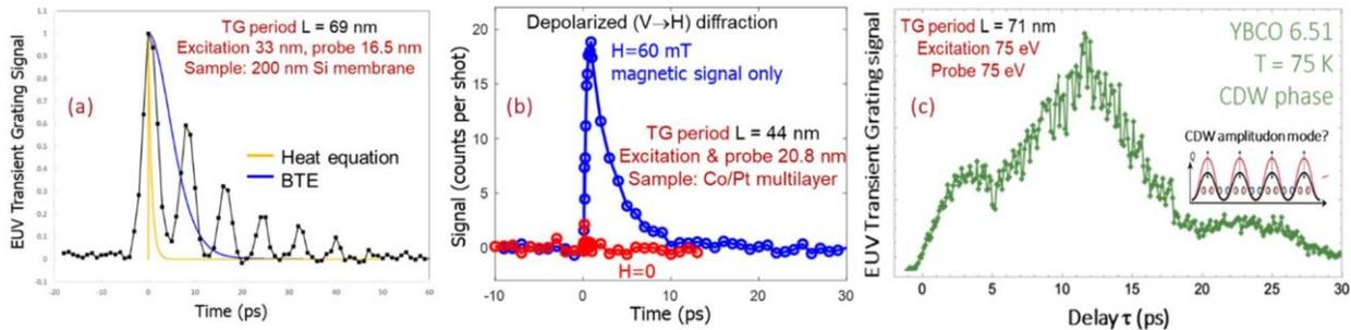
Figure 8. EUV transient grating results. (a) Thermoelastic response in Si showing highly nondiffusional nanoscale thermal transport kinetics. (b) Transient magnetization grating data from Co/Pt multilayer sample with external magnetic field to induce perpendicular magnetic anisotropy. (c) TG data from YBCO6.51 showing 2-THz oscillations that may reveal the CDW amplitudon mode at the TG wavevector.
