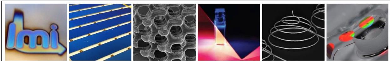
Representative LMI research efforts, from left: refractive index design via porous Si etching; concentrating photovoltaics capturing diffuse and direct irradiance; gyroid photonic crystal fabricated by two-photon lithography; photonic mirror and quantum dot design for luminescent solar concentrators; printed conductive Ag microstructures; conformal metafilm of Si nanoposts.
