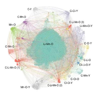
The reaction network for the C-Cl-Li-Mn-O-Y chemical system. The network contains 56 phases: 39 stable and 17 metastable. Chemical subsystems are labeled by color. The larger nodes indicate reactant nodes which are traversed on the 20 shortest pathways from precursors to targets in YMnO<sub>3</sub> synthesis.
