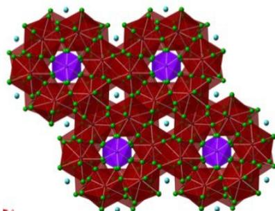
Structure of  $\text{Na}_3\text{AlPu}_6\text{F}_{30}$
