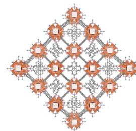
Single-crystal structure of Pu-MOF *Pu-Me<sub>2</sub>BPDC-12*
