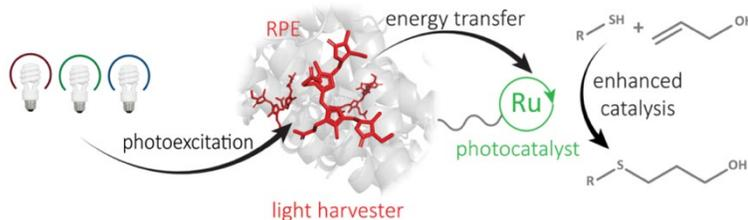
Prior work in BioLEC: Light-harvesting protein conjugated to Ru photocatalyst generates increased yields and makes reactions at previously unusable irradiation wavelengths possible.
