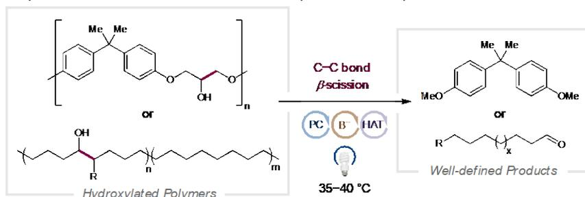
Prior work in BioLEC: photo-driven depolymerization of thermoplastics, enabled by light-driven O-H proton-coupled electron transfer. Approach is compatible with insoluble polymers and involves no stoichiometric reagents.
