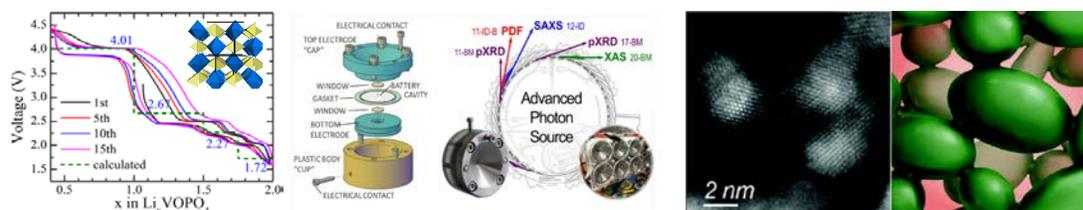
NECCES research from left to right: experimental and theoretical profiles of two Li cycling in  $\epsilon$ -LiVOPO<sub>4</sub>, AMPIX cell for in-situ synchrotron studies and techniques employed by NECCES at APS, TEM image and schematic of continuous Fe particle network enabling reversible conversion reaction of FeF<sub>2</sub>.
