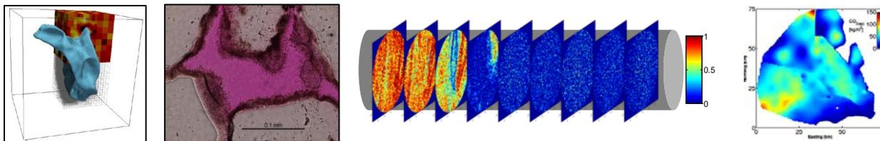
CFSES research, from left: Phase-field model of propagating fracture in a three dimensional heterogeneous media; Photomicrograph showing diffuse chlorite grain boundary after exposure to CO<sub>2</sub> (pink is the pore space between the grains); X-Ray computerized tomographic image of a core showing the uniform flow of CO<sub>2</sub> with surface-treated nanoparticles through a sandstone core; Distribution of dissolved CO<sub>2</sub> in the subsurface at Bravo Dome natural analog site.
