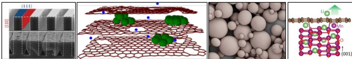
CEES research, from left: Crystallographically-controlled lithiation of silicon; Si/C composite anode architecture used by SiNode; Microspheres that are designed to melt and locally shut down a lithium ion battery when it overheats; Schematic of a graphene functionalized lithium manganese oxide cathode to control secondary reactivity (i.e., Mn loss).
