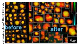
Using sophisticated techniques, EFRC researchers are observing, at the molecular level, how hydrogen fuel cells degrade. Microscope images reveal effects of aging on fuel cell catalyst nanoparticles.
