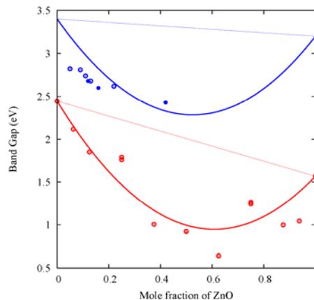
Variation of band gap as a function of Zn (O) concentration,  $x$ . Red: calculated BGs and smoothed  $E_g(x)$  curve using the estimated bowing parameter  $b$ . Blue: experimental data for (Ga<sub>1-x</sub>Zn<sub>x</sub>)(N<sub>1-x</sub>O<sub>x</sub>) solid solution and predicted experimental  $E_g(x)$  behavior using the estimated  $b$  and the limiting GaN and ZnO band gaps.
