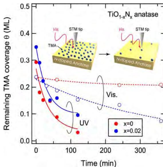
Fig. 3 STM results on the photodecomposition of TMA on pure and N-doped anatase (001) using UV and visible light.
