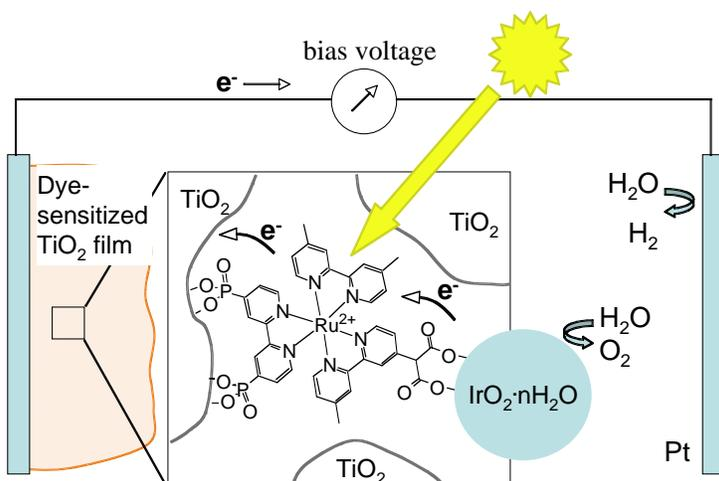
**Fig. 1.** Schematic of water splitting in an aqueous dye sensitized solar cell.
