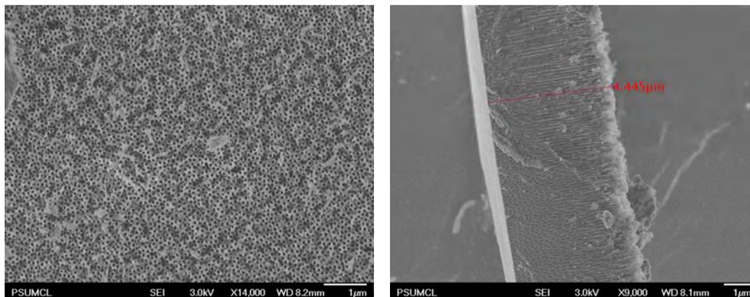
**Fig. 1:** Hematite nanotube arrays formed by anodization of Fe foil.
