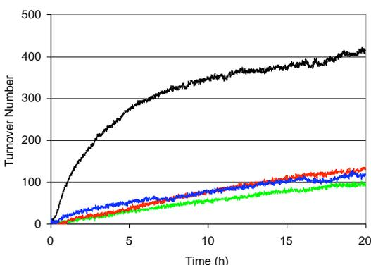
**Figure 1.** Kinetic plots of oxygen evolution vs time for complexes [Ru(tpy)(4-pic)<sub>3</sub>]<sup>2+</sup> (green), [Ru(bpy)(tpy)(4-pic)]<sup>2+</sup> (red), [Ru(dpp)(4-pic)<sub>2</sub>]<sup>2+</sup> (blue), and RuO<sub>2</sub> (black).
