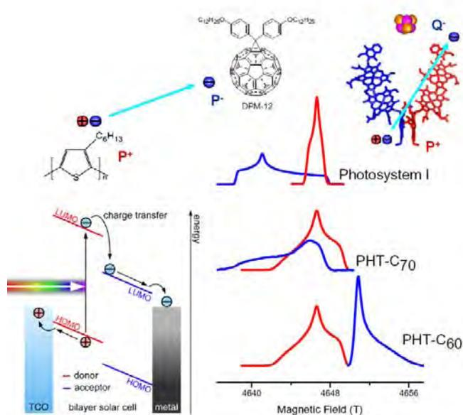
**Figure 1.** Schematic representation of the charge separation process in polymer-fullerene composites in comparison with photosystem I. Related HF EPR spectra are shown for positive (red) and negative (blue) polarons.
