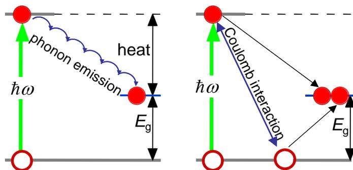
**Figure 1.** Traditional photoexcitation (left) versus carrier multiplication (right).  $E_g$  is the energy gap, which separates the valence from the conduction band.
