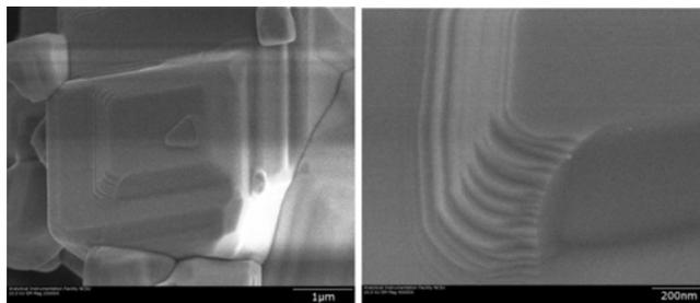
**Figure 2.** SEM Images of  $\text{AgNbO}_3$  particle surfaces exhibiting nano-stepped features.
