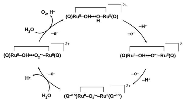
Proposed mechanism for water oxidation by the Tanaka catalyst in aqueous solution at pH 4.
