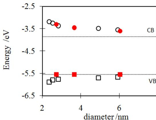
Figure 2. The graph plots the HOMO energies (open squares from electrochemistry and filled squares from photoemission measurements) and LUMO energies (open circles from electrochemistry and filled circles from photoemission measurements) of the different CdSe NPs as a function of their diameter. The dashed lines mark the bulk CdSe band positions, assuming that its valence band is pinned at 1.25 eV below the Fermi level of Au.
