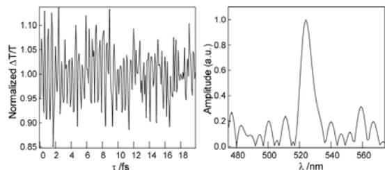
**Fig 1:** (left) Normalized transient absorption signal ( $\lambda_{\text{pump}}=522$  nm,  $\lambda_{\text{probe}}=1712$  nm;  $\Delta t = 27$  ps) during phase switching. (right) Fourier transform of signal.
