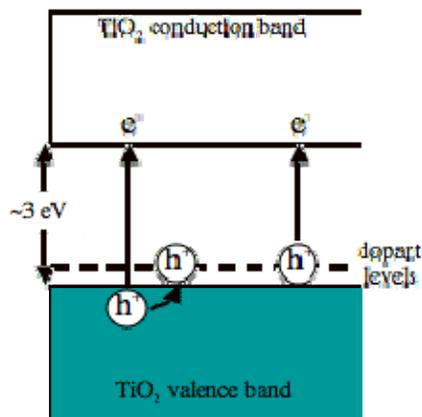
Fig. 1 Schematic illustration of band-to-band (left) and dopant-to-CB excitations in doped TiO<sub>2</sub>.
