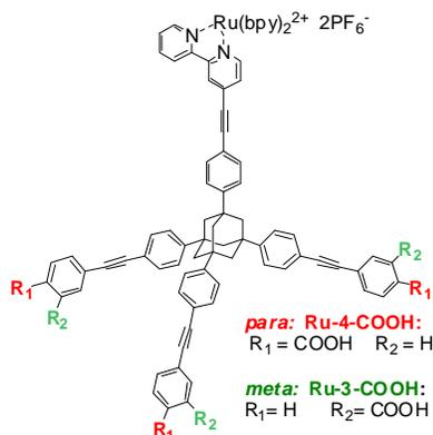
Two model dyes were synthesized for the experiments by an improved procedure: *meta* (Ru-3-COOH) and *para* (Ru-3-COOH) designed to compare the effect of a) different anchoring groups on surface binding modes and b) footprints size on injection and recombination dynamics. Binding was done on TiO<sub>2</sub> nanoparticle films, but sensitization of other semiconductor morphologies will be studied in the future.
