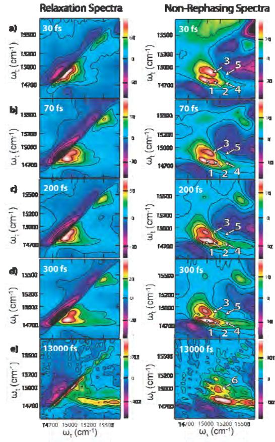
**Figure 1.** Experimental real 2D relaxation (left) and non-rephasing (right) spectra of LHCII at 77K. Arrows point to cross-peaks on the non-rephasing spectra to highlight energy transfer dynamics.
