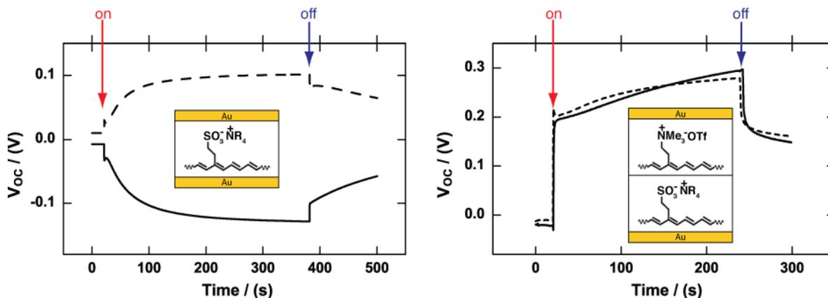
**Figure 3** - Time dependence of the photovoltage for a single layer ionomer structure and a bilayer heteroionic junction with illumination (100mW @ 532nm) on either side (solid vs. dashed line)
