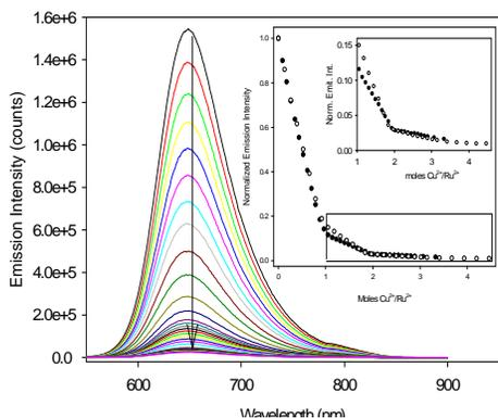
**Figure 2.** Spectrophotometric titration of  $\text{Cu}^{2+}$  into an acetonitrile solution of the  $\text{Ru}-(\text{bpy}-\text{bpy})_2$  hairpin.
