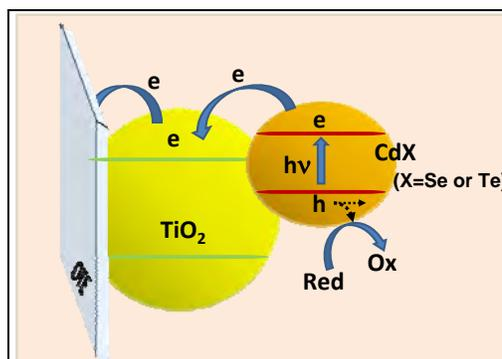
**Scheme 1.** Charge injection from excited semiconductor nanocrystal, CdX (X= Se or Te) into TiO<sub>2</sub> nanoparticle and scavenging of holes by a Red-Ox couple.
