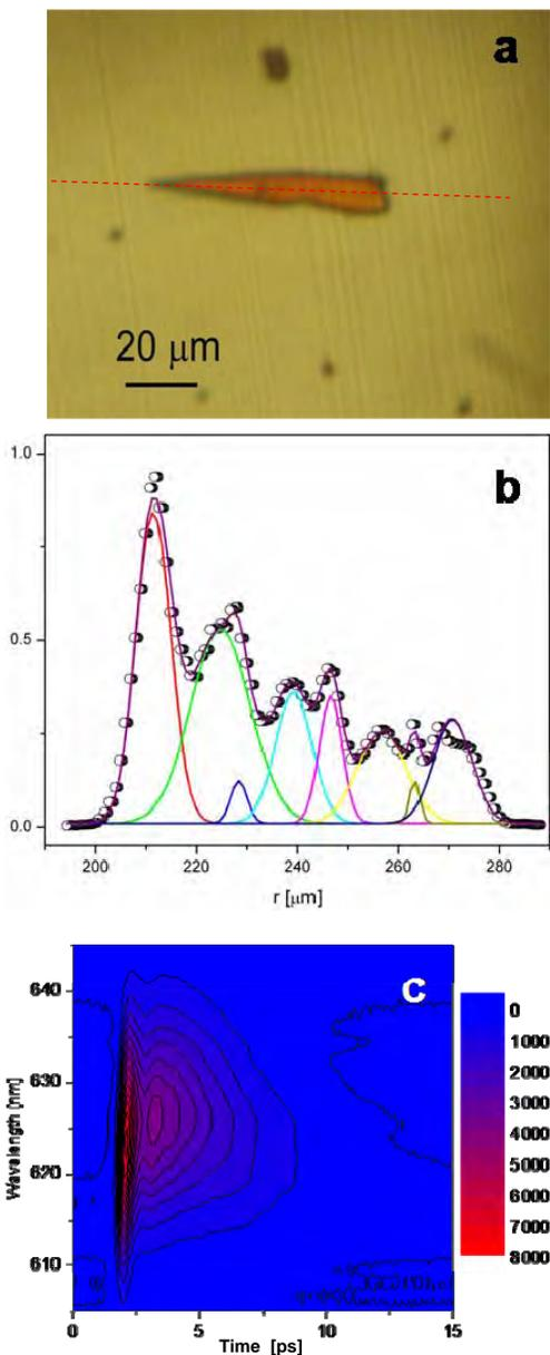
**Fig.1.** (a) A single 70×10 μm, 100 nm thick CdSSe nanobelt; (b) spatial emission cross-section collected 100 fs after the excitation; (c) spectrally and temporally resolved emission of the same nanobelt.
