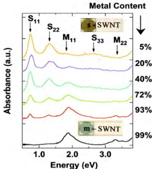
Figure: Absorption spectra of films formed from m- and s-SWNT samples.
