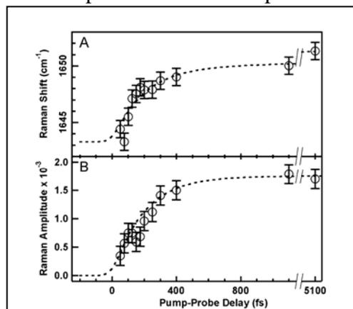
**Figure 1.** Time-dependence of the change in energy (A) and spectral amplitude (B) of the C=N stretching vibration of  $[\text{Fe}(\text{tren}(\text{py})_3)](\text{PF}_6)_2$  (**1**) derived from femtosecond stimulated Raman scattering data. The dashed lines correspond to fits to exponential kinetic models. Both the spectral shift and amplitude can be modeled with the same initial time constant of  $\tau = 190 \pm 50$  fs which is assigned to the formation of the  $^5T_2$  excited state of the
