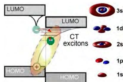
Fig. 1. Schematic illustration of charge transfer excitons at an organic donor-acceptor interface. Also shown are wavefunctions of a few CT excitons from numerical solutions to the Schrödinger equation within a dielectric continuum model.
