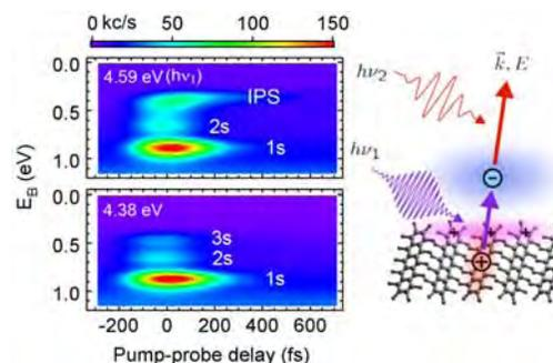
Fig. 2. Pseudo color plots of TR-2PPE spectra at different pump-probe delay times for a ~20 nm thick polycrystalline pentacene thin film grown on Si(111). The binding energy scale is referenced to the vacuum level. At  $h\nu_1 = 4.38$  eV (lower panel), the 1s, 2s, & 3s CT excitons are clearly resolved. When  $h\nu_1$  is increased to 4.59 eV, the delocalized image potential state (IPS) is also observed.
