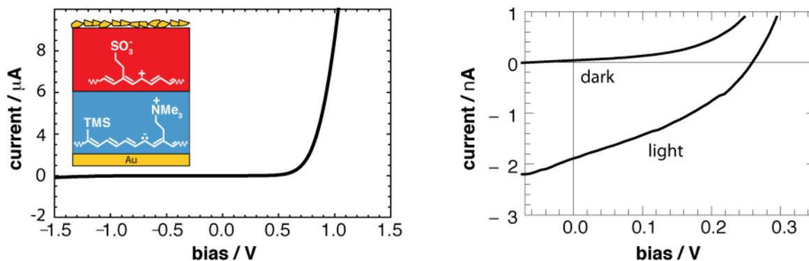
**Figure 2** - (left) Current-voltage behavior of the polyacetylene ionomer pn junction schematically shown inset. (right) Expanded current voltage curve including under illumination (50mW white light, tungsten-halogen)
