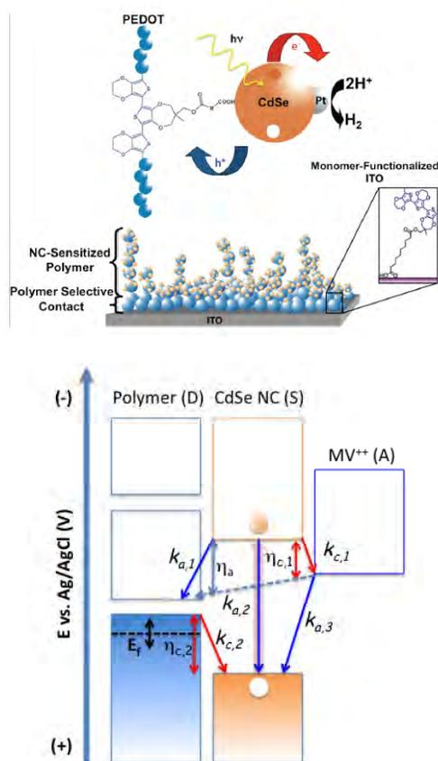
Fig. 1 – (up per) Schematic view s of electrochemically te tethered semic onductor nanoparticles; (lo wer) f rontier orb ital energy lev els w hich con trol rates of ET to/from the photoexcited SC-NP.
