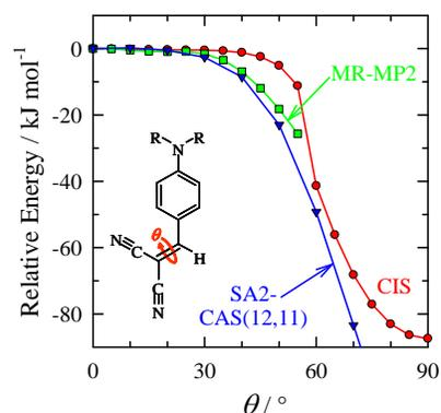
**Fig. 1:** Scans of the  $S_1$  potential energy surface of DMN in the gas phase using various model chemistries (6-31G(d) basis set).
