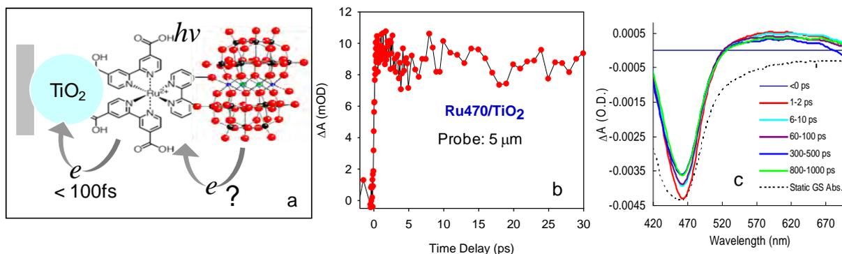
**Figure 1.** a) schematic view of the TiO<sub>2</sub>-Ru470-RuPOM photocatalytic system and b) Electron injection kinetics from Ru470 to TiO<sub>2</sub> probed by transient IR spectroscopy; c) Charge recombination kinetics probed by ground state recovery of Ru470-TiO<sub>2</sub>.
