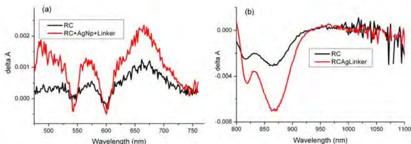
Figure 2: Transient Absorption spectra taken at pump-probe delay time of 80 ps for linked RC -Ag NP complexes compared with pure RCs for (a) visible and (b) near IR wavelength regions.
