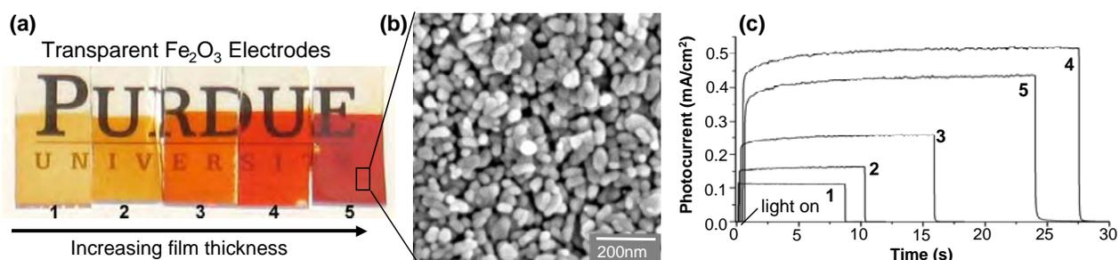
**Figure 1.** (a) Photograph, (b) SEM and (c) short-circuit photocurrents of anodically prepared  $\alpha$ -Fe<sub>2</sub>O<sub>3</sub> films in an acidic aqueous medium with varying deposition times; **1** (1 min), **2** (2 min), **3** (4 min), **4** (8 min), and **5** (16 min).
