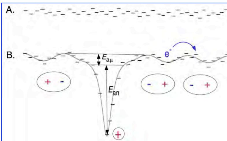
**Figure 1.** A. Schematic of an XSC conduction band showing uncorrelated gaussian disorder. B. Same with an ionized n-type dopant showing the (correlated) fluctuations caused by the majority of charges which remain bound. Activation energies for carrier generation and for mobility are shown.
