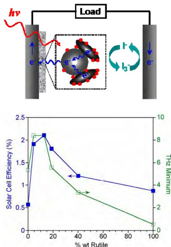
**Figure 1.** Top: Schematic representation of mixture of dye-sensitized anatase NPs with rutile NRs. Bottom: Overall cell efficiency and THz injection efficiency as a function of rutile NR fraction.
