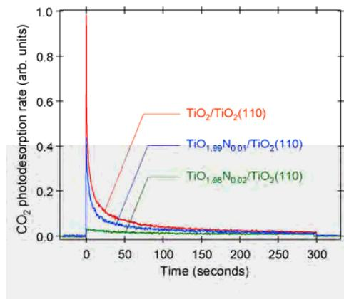
Fig. 2  $\text{CO}_2$  photodesorption spectra for TMA on pure and N-doped  $\text{TiO}_2$  rutile.
