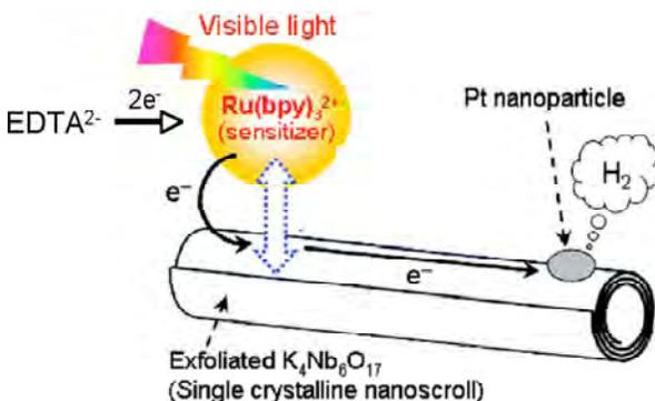
**Fig. 2.** Left: scheme for photochemical H<sub>2</sub> evolution. Right: TEM image of single crystalline nano-scrolls derived from K<sub>4</sub>Nb<sub>6</sub>O<sub>17</sub>.
