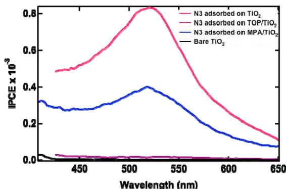
Figure 1. Sensitization spectra for N3 on anatase(101) single crystals were sensitized with on bare (pink), TOP-exposed (purple) and MPA-exposed surfaces.
