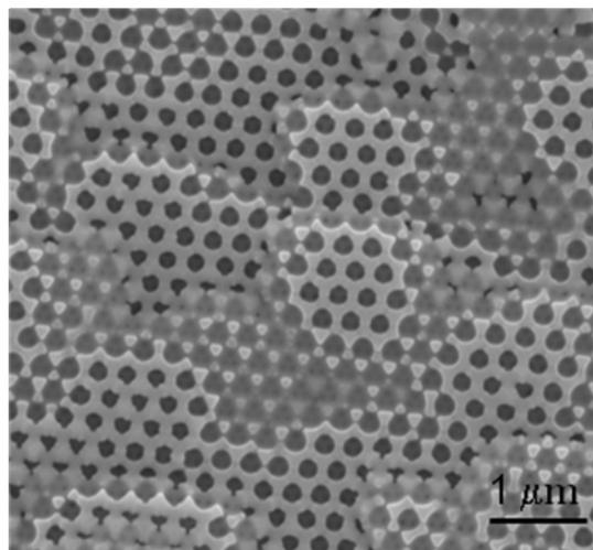
**Figure 1:** FE-SEM image of CdSe inverse opal film formed from 300 nm PS bead template.
