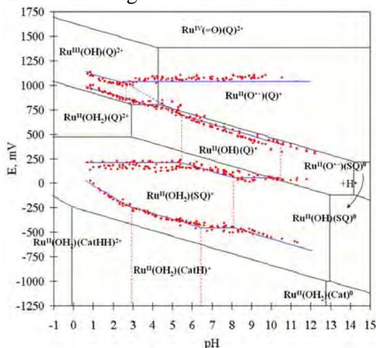
An experimental and theoretical Pourbaix diagram of Ru(OH<sub>2</sub>)(Q)(tpy)<sup>2+</sup>.  $E_{1/2}$  is relative to the SCE. The red dashed and solid blue lines correspond to the experimental  $pK_a$  and redox potentials. The black lines are the theoretical predictions.
