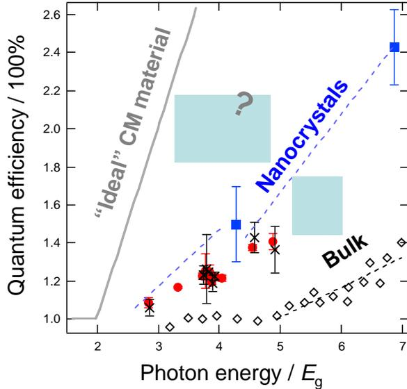
**Figure 2.** Photon-to-exciton conversion efficiencies in PbSe nanocrystals compared to bulk PbS. The grey line is the “ideal” efficiency line defined by energy conservation.
