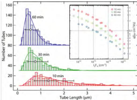
**Figure 2** – SWNT nanotube length distributions after 10, 30 and 60 minutes sonication. Inset shows how the peak TRMC signal is reduced as the nanotube length is decreased.
