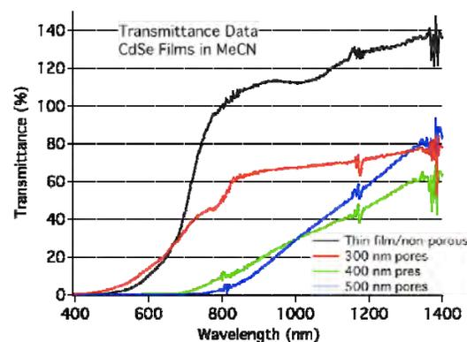
**Figure 2:** Transmittance data for non-porous and 300, 400 & 500 nm pore-sized inverse opal CdSe films in acetonitrile.
