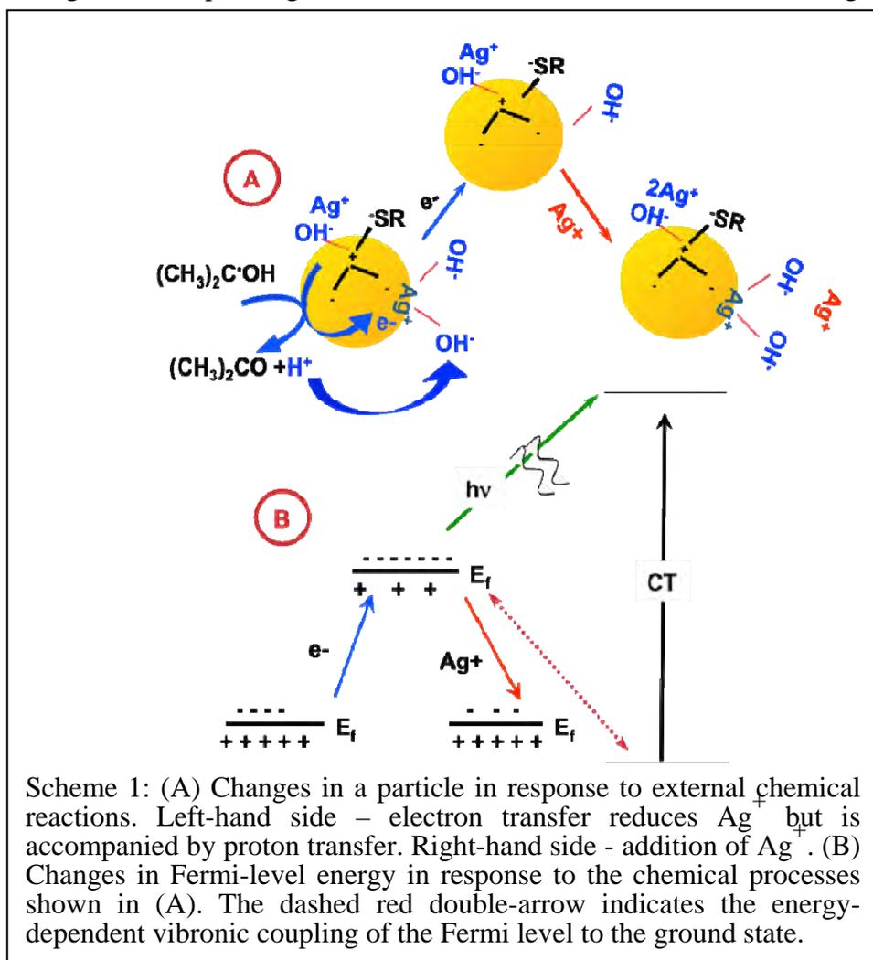
Scheme 1: (A) Changes in a particle in response to external chemical reactions. Left-hand side – electron transfer reduces  $Ag^+$  but is accompanied by proton transfer. Right-hand side - addition of  $Ag^+$ . (B) Changes in Fermi-level energy in response to the chemical processes shown in (A). The dashed red double-arrow indicates the energy-dependent vibronic coupling of the Fermi level to the ground state.
