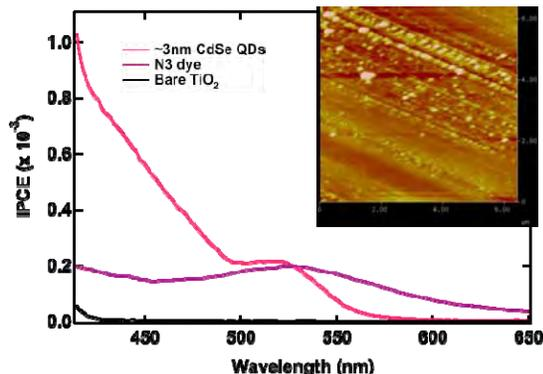
Figure 2. Rutile (110) single crystal sensitized with  $\sim 3$ nm CdSe QDs capped with MPA and N3 for comparison. Inset: AFM image of QDs on rutile where an intentional scratch was used to measure the stepheight of the monolayer.
