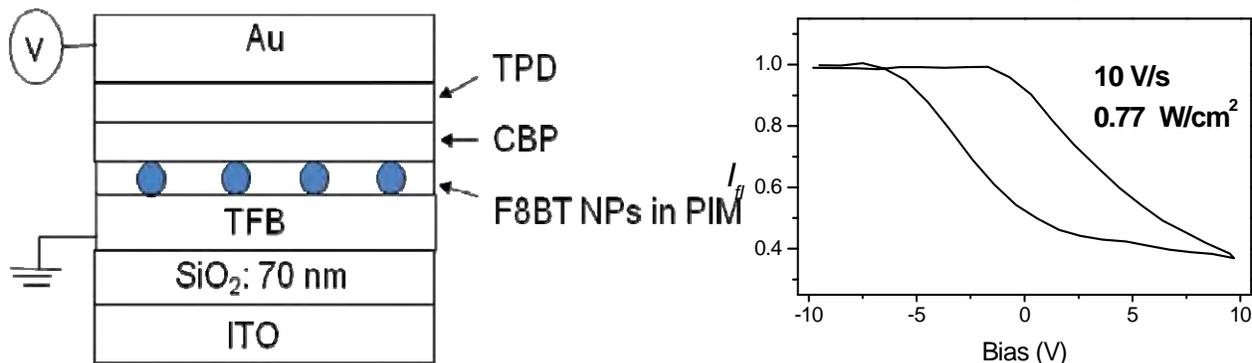
quantum efficiency for charge separation is indirectly probed by monitoring the quenching of the single-molecule fluorescence spectroscopy intensity in device geometry with external electrodes. Single molecule electron transfer rate constants  $k_{et}$  and other aspects of the kinetics and dynamics have been studied using **coordinated and simultaneous single molecule spectroscopy and device modulation** (E-field, excitation intensity, etc).
