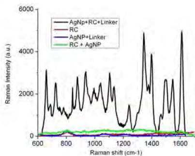
Figure 1: Raman spectra of RCs linked with Ag NPs compared with pure RCs, Ag NPs with linkers and unlinked RCs and Ag NPs.
