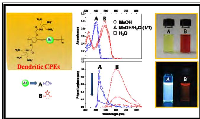
This approach is detailed by the results for two members of the cationic poly(*p*-phenylene ethynylene) (PPE) CPE family shown with phenylene (high gap) and benzothiadiazole (BTD) (low gap) linkages modifying the electronic structure. While the absorbance results demonstrate band gap narrowing (color change of yellow to red), aggregation effects are exemplified by the reduced fluorescence intensity as the solvent is changed from methanol to water.
