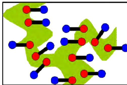
Figure 1. This cartoon illustrates localization of the dyads (red and blue dumbbells) between two phases, which form the anode (green) and cathode (white) of a photoelectric device that can be optically thick but physically thin.
