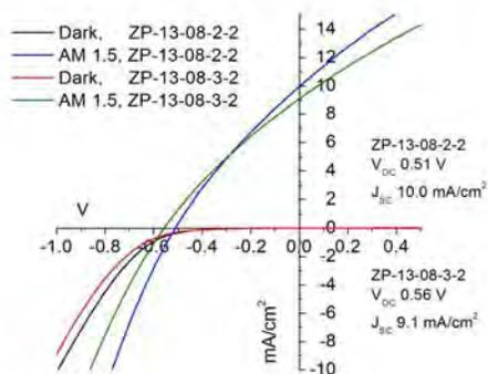
Fig. 2. Dark and light J-V traces of two Mg/ $\text{Zn}_3\text{P}_2$  Schottky diodes.
