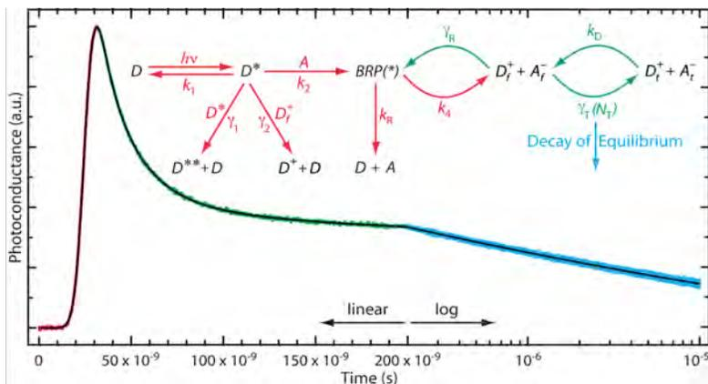
**Figure 1** - TRMC signal from a 1% blend of PCBM dispersed in P3HT recorded at moderately high laser powers to accentuate the second-order recombination process. The fit through the data arises from analysis of the kinetic scheme shown in the inset.
