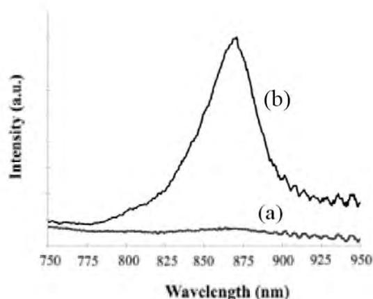
Fig. 1. Steady-state photoluminescence intensity of N<sub>2</sub>H<sub>2</sub>-functionalized samples (a) before and (b) after annealing.
