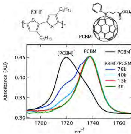
Fig. 3. FTIR spectra for P3HT/PCBM bulk heterojunctions. Also shown is a spectrum (black) for chemically reduced PCBM. The colors correspond to different P3HT molecular weight.
