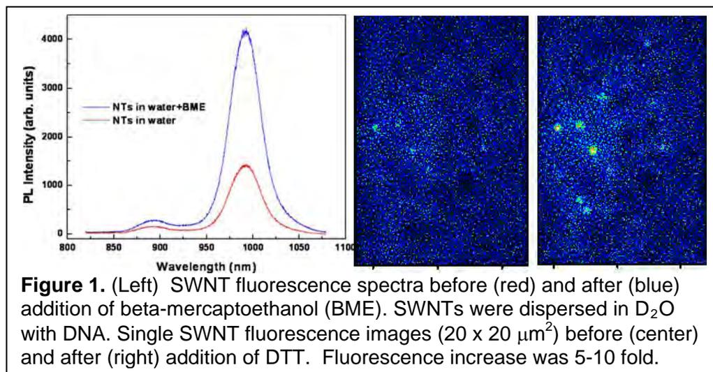
**Figure 1.** (Left) SWNT fluorescence spectra before (red) and after (blue) addition of beta-mercaptoethanol (BME). SWNTs were dispersed in D<sub>2</sub>O with DNA. Single SWNT fluorescence images (20 x 20 μm<sup>2</sup>) before (center) and after (right) addition of DTT. Fluorescence increase was 5-10 fold.
