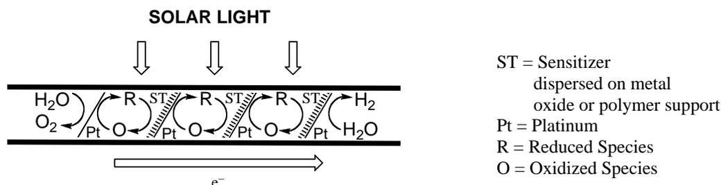
A multipanel dye-sensitized water-splitting device composed of three such panels arranged in series.
