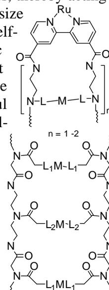
**Figure 1.** Two general structural motifs in the proposed experiments are (top) palindromic sequences and (bottom) hairpins, where M is Cu (II), L is bpy, and n is the number of repeat units on the chain.
