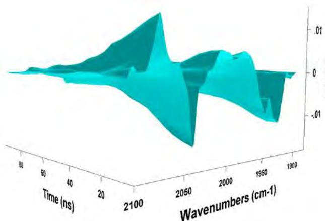
Time-resolved step-scan FTIR spectra of the MLCT excited state of ReCl(dnb-F<sub>26</sub>)(CO)<sub>3</sub> in scCO<sub>2</sub> (35 °C, 13.8 MPa), recorded after 410 nm excitation.
