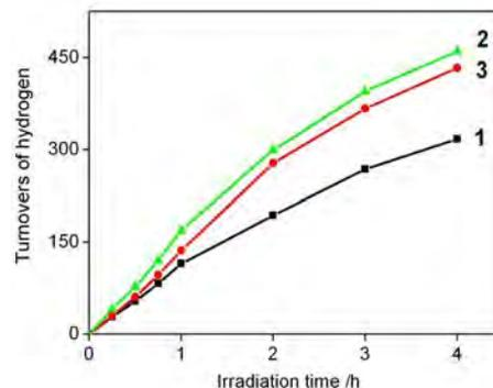
H<sub>2</sub> yield using Eosin Y ( $1.1 \times 10^{-5}$  M) and different cobalt complexes ( $2.0 \times 10^{-5}$  M),  $1.6 \times 10^{-2}$  M TEOA at pH=8.5.
