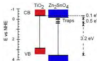
**Figure 1.** Comparative energy diagram of  $\text{TiO}_2$  and  $\text{Zn}_2\text{SnO}_4$  in aqueous solution at pH 4.8.
