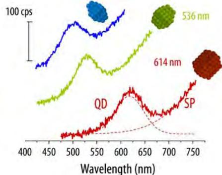
Fig 1. Electroluminescence from CdSe quantum dots of different sizes labeled with their PL maximum.
