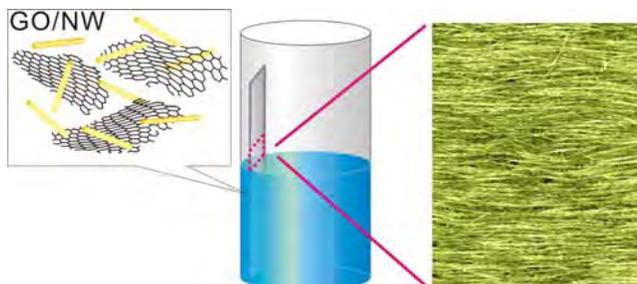
**Figure 2:** Coassembly of graphene oxide (GO) nanosheets and nanowires (NW) for nanowire alignment.
