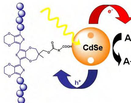
Fig. 1 – Schematic view of the photoelectrochemical reaction of an electrochemically “wired” semiconductor nanoparticle, involving hole-capture by an electron-rich polymer host and electron capture by a solution electron acceptor (e.g.  $H^+$ ).<sup>1,2,7</sup>
