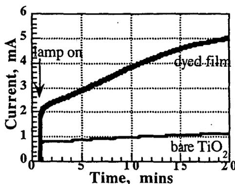
Figure 2. Current vs. time of DSSC's under UV illumination.
