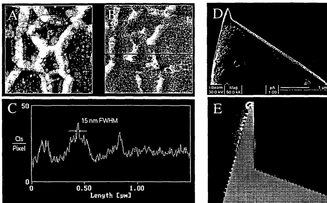
(A) Simultaneous topographic and (B) near-field TPE fluorescence images of thylakoid membranes, (C) and the cross-section of the black line in (B) with a feature with FWHM of 15 nm. (D) Electron micrograph of the FIB milled Au tip, and (E) Electric field distribution based on a FDTD simulation for the Au tip used for obtaining the images. The field is strongest at the apex of the tip, with a field enhancement of 80.
