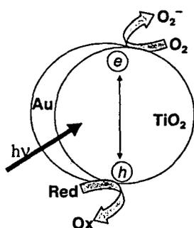
Figure 1. Improving the charge separation in a semiconductor-metal composite Nanoparticle
