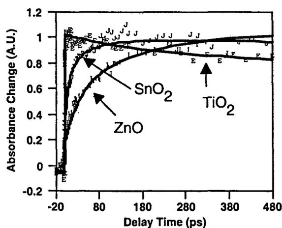
Fig. 1. Comparison of electron injection dynamics in Ru N3 sensitized TiO<sub>2</sub>, SnO<sub>2</sub> and ZnO thin film
