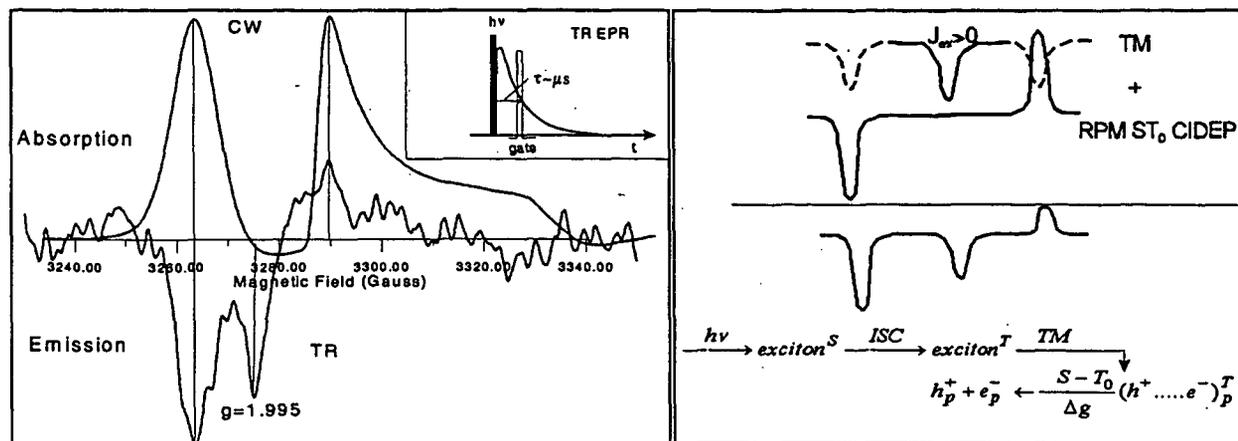
**Figure 2** Comparison between integrated continuous light-induced (upper trace) and time-resolved pulsed laser-induced (lower trace) EPR spectra from 4nmTiO<sub>2</sub> modified with ascorbate. The lower trace was obtained with a 550 nm laser (laser intensity 10 mJ per pulse, 10 ns pulse duration), 1  $\mu$ s after the laser pulse. Right section shows how triplet and radical pair mechanism of CIDEP in addition to fast exchange can contribute to the observed polarized spectrum.
