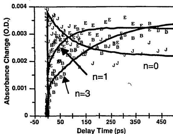
Fig. 2. Dependence of Electron injection rate on the number of CH<sub>2</sub> units in ReCon sensitized TiO<sub>2</sub> thin films
