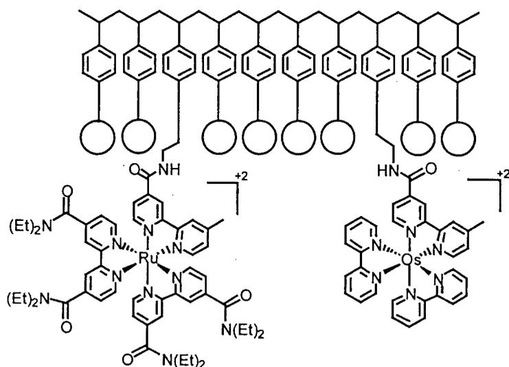
**Fig. 1:** Schematic diagram of PS-Ru<sub>17</sub>Os<sub>3</sub> assembly. Open circles represent Ru(II) and Os(II) complexes that are not shown for clarity.
