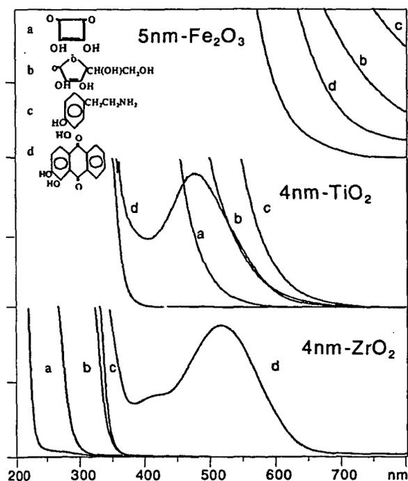
Figure 1 Optical properties of different metal oxide nanocrystallites surface modified with different enediol ligands, a-d.
