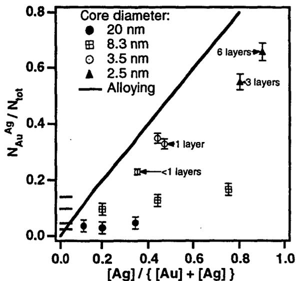
Figure 1: Size dependent alloying of  $\text{Au}_{\text{core}}\text{-Ag}_{\text{shell}}$  particles. Plotted is the fraction of Ag atoms around Au vs. the stoichiometry of particles of various sizes. Complete alloying will follow the diagonal line. Complete segregation will follow the small right-hand horizontal lines for the 20 to 2.5 nm (from bottom up) particles.
