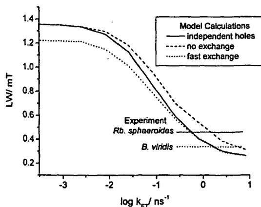
Figure 1. Comparison of calculated and experimental EPR line widths for oxidized LH-I complexes as a function of ET rate.
