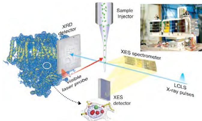
Fig. 1. Schematic of the simultaneous detection of XRD and XES of PS II crystals. PS II crystals are injected using an electrofocusing nanoflow system. Downstream of the X-ray laser is a multi-pixel detector that collects the X-ray diffraction from the crystals. A dispersive X-ray emission spectrometer with 16-cylindrically bent analyzer crystals focus the Mn K $\beta$  XES on a position sensitive detector.
