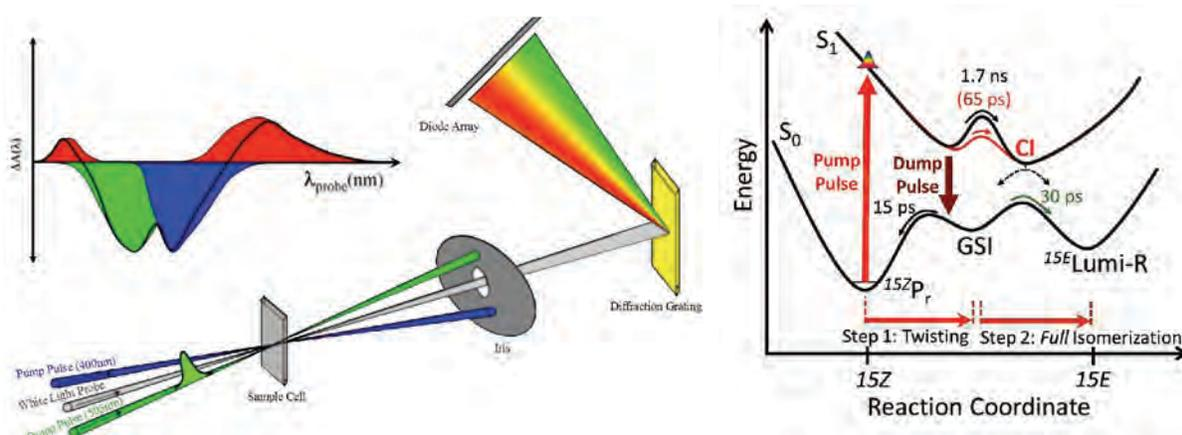
Figure 1. Left Panel: Schematic of the dispersed pump-dump-probe setup (with 400-nm pump, 500-nm dump and broadband whitelight probe). Inset: model transient absorption spectra. Right Panel: Potential Energy Surface of the forward reaction of NpR6012g4 based on target model of the dispersed pump-dump-probe. The dump pulse generates the reactive ground-state intermediate responsible for the second-chance initiation dynamics (SCID) and high quantum yield of this CBCR domain.
