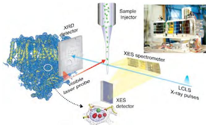
Fig. 1. Schematic of the simultaneous detection of XRD and XES of PS II crystals. PS II crystals are injected using an electrofocusing nanoflow system. Downstream of the X-ray laser is a multi-pixel detector that collects the X-ray diffraction from the crystals. A dispersive X-ray emission spectrometer with 16-cylindrically bent analyzer crystals focus the Mn Kβ XES on a position sensitive detector.
